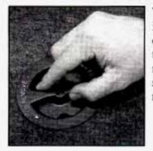
The equipment you'll need is in the trunk. Pull the carpeting from the floor of the trunk. Turn the center retainer nut on the compact spare cover to the left to remove it.
