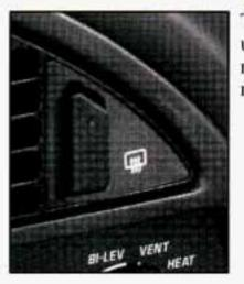
The rear window defogger uses a warming grid to remove fog from the rear window.
