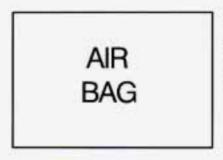
There is an air bag readiness light on the instrument panel, which shows AIR BAG.
