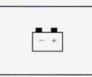
The charging system indicator light will come on when you start the engine, then it should go out. If it stays on, or comes on while you are driving, you may have a problem with the electrical charging system. It could indicate that you have a loose generator drive belt or another electrical problem. Have it checked right away. Driving while this light is on could drain your battery.
