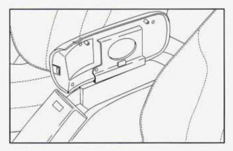
The armrest opens into a storage area for cassette tapes, gloves, etc. To open it, lift up on driver's side front portion of the armrest. A tissue holder is located under the lid of the armrest. There is also an accessory power outlet located in the front storage armrest. To use the accessory power outlet, see "Accessory Power Outlet" later in this section.
