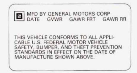
The other label is the Certification label, found on the rear edge of the driver's door. It tells you the gross weight capacity of your vehicle, called the GVWR (Gross Vehicle Weight Rating). The GVWR includes the weight of the vehicle, all occupants, fuel and cargo. Never exceed the GVWR for your vehicle, or the Gross Axle Weight Rating (GAWR) for either the front or rear axle.
