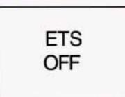
With the Enhanced Traction System (ETS), this warning light should come on briefly as you start the engine.
