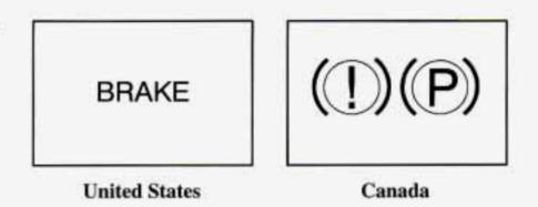
When your brake fluid falls to a low level, your brake warning light will come on. See "Brake System Warning Light" in the Index.
