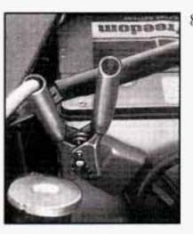
Don't let the other end touch metal. Connect it to the positive (+) terminal of the good battery. Use a remote positive (+) terminal if the vehicle has one.
