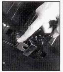
To turn the lockout on, slide the switch all the way to the right. To turn the lockout off, slide the switch all the way to the left.
