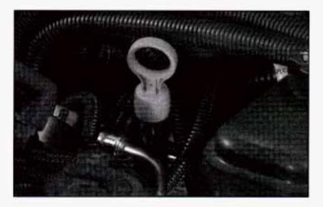
The automatic transaxle dipstick handle is red. Pull out the dipstick and wipe it with a clean rag or paper towel. Push it back in all the way, wait three seconds and then pull it back out again.
