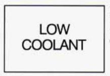
If the LOW COOLANT light comes on, it means you're low on engine coolant.
