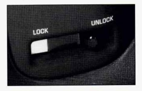
From the inside, to lock the door, slide the locking lever rearward.
