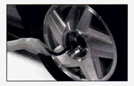
Then use the wheel wrench to *loosen* all the wheel nuts. Don't remove them yet.
