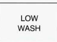
The LOW WASH light will come on when you turn on the ignition, and the fluid container is less than one-third full.
