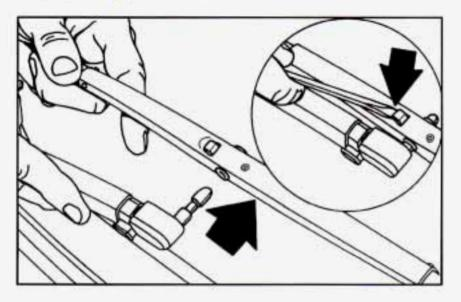
Replacement blades come in different types and are removed in different ways. Here's how to remove the type with a release clip:
