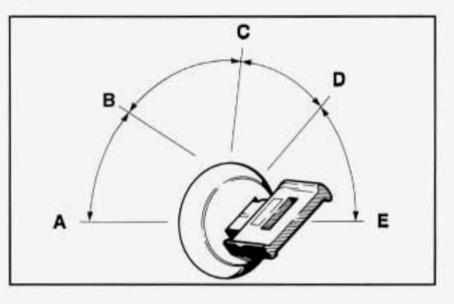
With the ignition key in the ignition switch, you can turn the switch to five positions.
