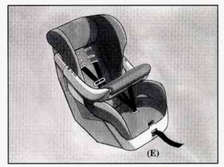
A forward-facing child restraint (C-E) positions a child upright to face forward in the vehicle. These forward-facing restraints are designed to help protect children who are from 20 to 40 lbs. (9 to 18 kg) and about 26 to 40 inches (66 to 102 cm) in height, or up to around four years of age. One type, a convertible restraint, is designed to be used either as a rear-facing infant seat or a forward-facing child seat.
