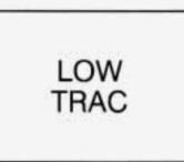
This light will come on when your Enhanced Traction System is limiting wheel spin. See "Enhanced Traction System Active Light" in the Index.
