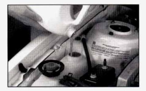
Then fill the coolant surge tank with the proper mixture, up to FULL COLD, or just above the small cylinder at the base of the opening.
