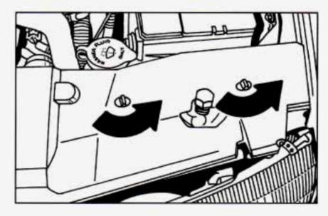
On the driver's side only, unscrew the butterfly fasteners. Then lift the plate.
