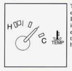
This gage shows the engine coolant temperature. If the gage pointer moves into the red area, your engine is too hot! It means that your engine coolant has overheated.
