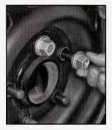
Replace the wheel nuts with the cone end of the nuts toward the wheel.
