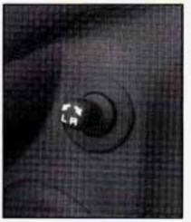
This selector knob, located on the driver's door, controls both outside rearview mirrors. Select the mirror you want to adjust by rotating the knob to the left or right. Adjust each mirror so that you can just see the side of your vehicle when you are sitting in a comfortable driving position.
