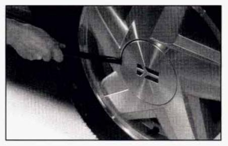
On some models, a cover plate must be removed to find the wheel nuts. Carefully use the wedge end of the wheel wrench to pry it off.
