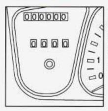
The trip odometer can tell you how far you have driven since you last reset it. To reset the trip odometer to zero, press the knob below it.
