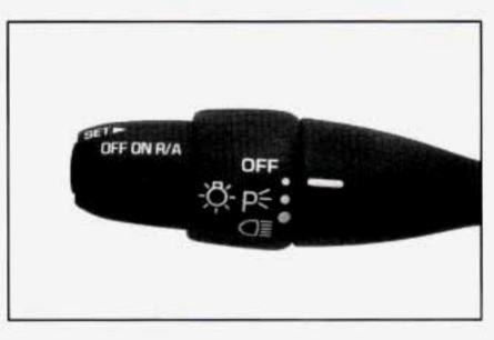
Rotate the turn signal lever middle ring up one position to turn on:
