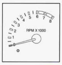
The tachometer shows your engine speed in revolutions per minute (rpm).
