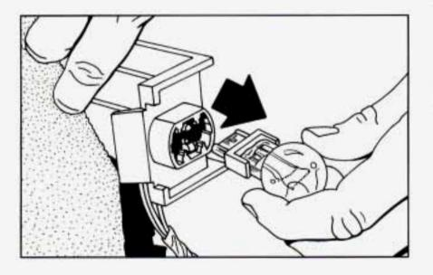
3. Wiggle the bulb out of the socket.
