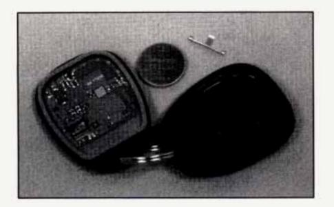
To replace the battery in the remote lock control:
