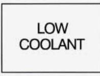
If this light comes on and stays on, the vehicle should promptly be pulled off the road and the coolant level checked.
