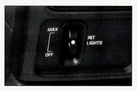
You can brighten or dim the instrument panel cluster lights by rotating the INT LIGHTS switch.
