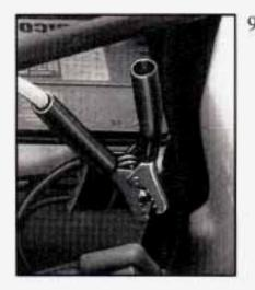
Now connect the black negative (-) cable to the good battery's negative (-) terminal. Don't let the other end touch anything until the next step. The other end of the negative cable *doesn't* go to the dead battery.
