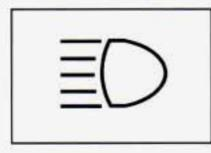
To change the headlamps from low beam to high or high to low, pull the turn signal lever all the way toward you. Then release it.
