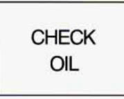
If you have a 3100 engine, this light should come on briefly when you start the engine. If the light doesn't come on, have it repaired.
