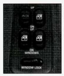
Switches on the driver's armrest control each of the windows when the ignition is on. In addition, each passenger door has a switch for its own window.
