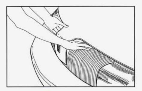
Before closing the hood, be sure all the filler caps are on properly. Then just let the hood down and close it firmly.
