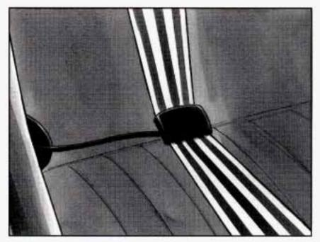
Be sure that the belt is not twisted and it lies flat. The elastic cord must be under the belt and the guide on top.
