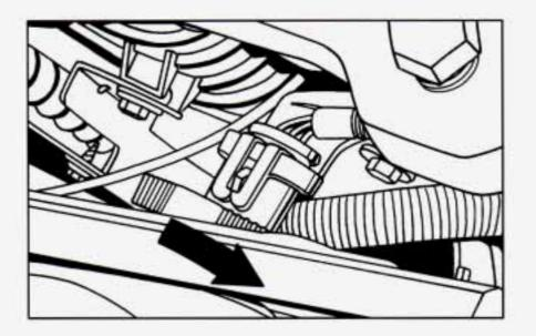
Twist the lock ring to the right one-sixth of a turn and pull out the bulb assembly.
