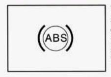
With the anti-lock brake system, this light will come on when you start your engine and it will stay on for three seconds. That's normal.
