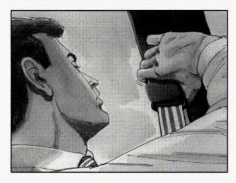
To move it down, squeeze the release button and move the adjuster to the desired position. You can move the adjuster up just by pushing up on the shoulder belt guide. After you move the adjuster to where you want it, try to move it down without squeezing the release button to make sure it has locked into position.
