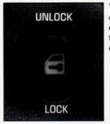
With power door locks, you can lock or unlock all the doors of your vehicle from the driver or front passenger door lock switch.
