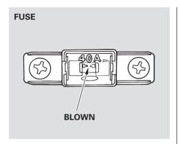
3. Check each of the large fuses in the under-hood fuse box by looking through the top at the wire inside. Removing these fuses requires a Phillips-head screwdriver. 4. Check the smaller fuses in the under-hood fuse box and all the fuses in the interior fuse box by pulling out each fuse with the fuse puller provided in the interior fuse box.
