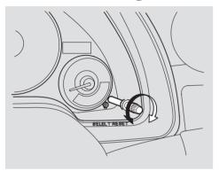
The knob on the instrument panel controls the brightness of the instrument panel. Turn the knob to adjust the brightness.
