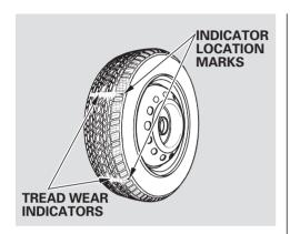
Your tires have wear indicators molded into the tread. When the tread wears down, you will see a band 1/2 inch (12.7 mm) wide across the tread. This shows there is less than 1/16 inch (1.6 mm) of tread left on the tire.
