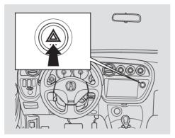
Push the red button to turn on the hazard warning lights (four-way flashers). This causes all four outside turn signals and both indicators in the instrument panel to flash. Use the hazard warning lights if you need to park in a dangerous area near heavy traffic, or if your vehicle is disabled.
