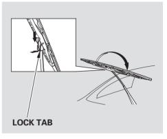
2. Disconnect the blade assembly from the wiper arm by pushing in the lock tab. Hold the lock tab in while you push the blade assembly toward the base of the arm.
