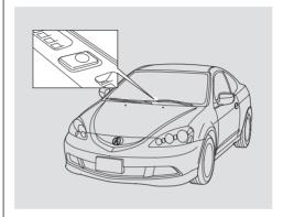
The heating and cooling system has temperature sensors next to the steering column and in the top of the dashboard. Do not cover the sensors or spill any liquid on them.
