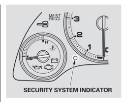
Once the security system is set, opening either door (without using the key or the remote transmitter), or the hood, will cause it to alarm. It also alarms if the radio is removed from the dashboard or the wiring is cut.
