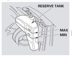
Look at the coolant level in the radiator reserve tank. Make sure it is between the MAX and MIN lines. If it is below the MIN line, see **Adding Engine Coolant** on page 165 for information on adding the proper coolant.
