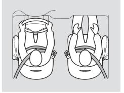
Your vehicle also has side airbags to help protect the upper torso of the driver or a front seat passenger during a moderate to severe side impact (see page 25 for more information on how your side airbags work).
