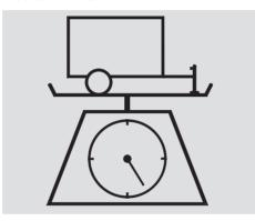
• Total Trailer Weight: The maximum allowable weight of the trailer and everthing in or on it must not exceed 1,000 lbs (450 kg). Towing a load that is too heavy can seriously affect your vehicle's handling and performance. It can also damage the engine and drivetrain.
