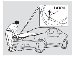
2. Put your fingers under the front edge of the hood just to left of center. Lift up the hood latch handle until it releases the hood. Lift up the hood.
