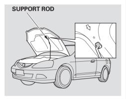
3. Pull the support rod out of its clip and insert the end into the designated hole in the hood.
