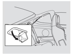
To use this coat hook, rotate the hook down. Close it with a firm push.
