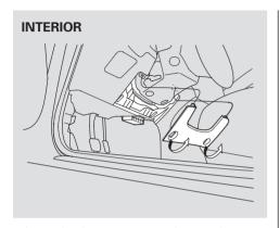
The vehicle's fuses are located in two fuse boxes. The interior fuse box is underneath the steering column.
