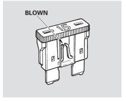
5. Look for a burned wire inside the fuse. If it is burned, replace it with one of the spare fuses of the same rating or lower.
