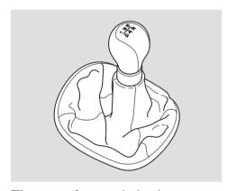
The manual transmission is synchronized in all forward gears for smooth operation. It has a lockout so you cannot shift directly from Fifth to Reverse. When shifting up or down, make sure you push the clutch pedal down all the way, shift to the next gear, and let the pedal up gradually. When you are not shifting, do not rest your foot on the clutch pedal. This can cause your clutch to wear out faster.
