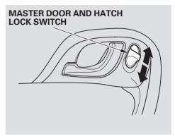
To lock both doors and the hatch, press the master door lock switch on either door, press the lock tab down on the driver's door, or use the key on the outside lock
