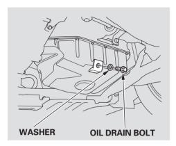
2. Open the hood and remove the engine oil fill cap. Remove the oil drain bolt and washer from the bottom of the engine. Drain the oil into an appropriate container.
