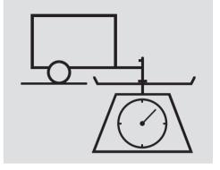
• Tongue Load: The weight that the tongue of a fully-loaded trailer puts on the hitch should be approximately 10 percent of the total trailer weight. Too much tongue load reduces front-tire traction and steering control. Too little tongue load can make the trailer unstable and cause it to sway.
