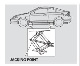
9. Place the jack under the jacking point. Turn the end bracket clockwise until the top of the jack contacts the jacking point. Make sure the jacking point tab is resting in the jack notch.
