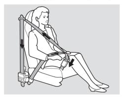
For added protection, the front seat belts are equipped with automatic seat belt tensioners. When activated, the tensioners immediately tighten the belts to help hold the driver and a front passenger in place. The tensioners are designed to activate primarily in frontal collisions, and they should activate in any collision severe enough to cause front-airbag inflation.
