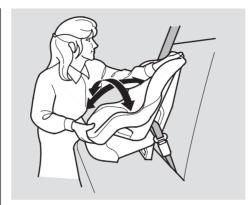
5. Push and pull the child seat forward and from side to side to verify that it is firmly secured during normal driving maneuvers. If the child seat is not secure, unlatch the belt, allow it to retract fully, then repeat these steps.
