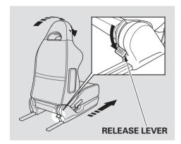
To get out from the rear seat on the passenger's side, push down on the release lever at the base of the seat-back. The seat-back will tilt forward, and the seat will slide forward.
