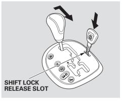
6. Remove the key from the Shift Lock Release slot. Press the brake pedal and restart the engine.
