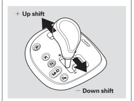
In Sequential SportShift mode, each time you push forward on the shift lever, the transmission will shift to a higher gear. Pull back on the lever to downshift. The number of the gear selected is displayed on the instrument panel (see page 139).
