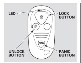
**LOCK** — Press this button to lock both doors and the hatch. You cannot lock the doors or the hatch if either door or the hatch is not fully closed or if the key is in the ignition switch.
