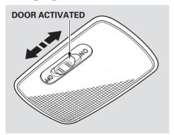
The ceiling light has a three-position switch. In the OFF position, the light does not come on. In the center position, the ceiling light comes on when you open either door. After the doors are closed tightly, the light dims slightly, then fades out in about 30 seconds. In the ON position, the ceiling light stays on continuously.
