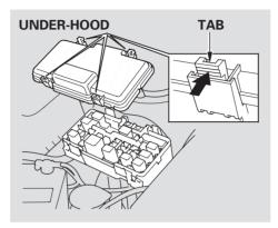
The under-hood fuse box is in the engine compartment next to the battery.
