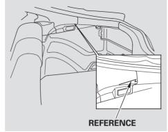
There is a reference line on the cargo area side panel. To avoid damaging the cargo cover, remove the cover if the cargo goes above that line.
