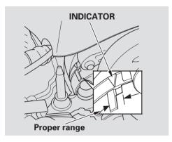
An auto-tensioner adjusts the tension of the drive belt. The indicator on the auto-tensioner should be in the proper range. It should be checked according to the time and distance recommendations in the maintenance schedule.
