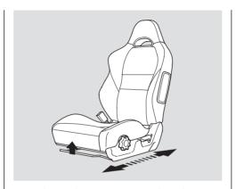
To adjust the seat forward and backward, pull up on the bar under the seat cushion's front edge. Then try to move the seat to make sure it is locked in position.
