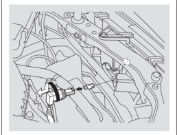
1. The front parking light bulb is above the high beam headlight bulb.
