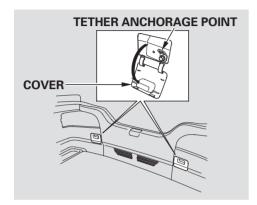
The tether anchorage points are located under plastic covers. Pivot the cover downward to access the anchorage point.
