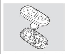
To replace the battery, place a cloth on the edge of the transmitter and remove the upper half by carefully prying on the edge with a small flattip screwdriver.
