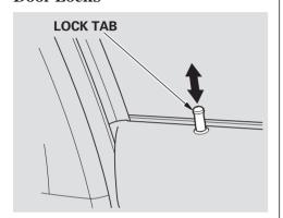
Each door has a lock tab at the top of the door. When you push down the lock tab on the driver's door, both doors and the hatch lock. The lock tab on the passenger's door locks and unlocks only that door. Pulling up on the driver's door lock tab only unlocks the driver's door To unlock the driver's door from the outside, turn the key and release it. If you turn and hold it, both doors and the hatch unlock. Both doors and the hatch unlock when you use the key in the passenger's door.
