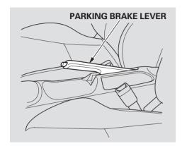
To apply the parking brake, pull the lever up fully. To release it, pull up slightly, push the button, and lower the lever. The parking brake light on the instrument panel should go out when the parking brake is fully released (see page 53).
