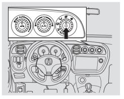
The rear window defogger will clear fog, frost, and thin ice from the window. Push the defogger button to turn it on and off. The indicator in the button comes on to show the defogger is on. If you do not turn it off, the defogger will shut itself off after about 25 minutes. It also shuts off when you turn off the ignition switch. You have to turn it on again when you restart the vehicle.
