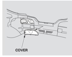
1. Open the hatch. Remove the light assembly cover by pulling on the tab on the outside edge.
