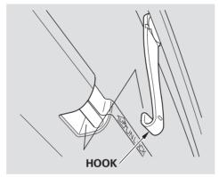
2. Push up on the sides of the cargo area cover to release the cover from the hooks.
