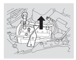
Then remove the bolt from the battery hold-down, and carefully push the battery toward the windshield to obtain enough working space.
