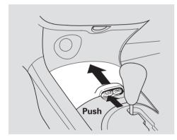
To open the beverage holder, push the left knob and slide the cover forward.
