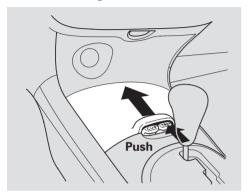
To open the console compartment, push the right knob and slide the cover forward.
