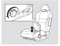
The height of your driver's seat is adjustable. Turn the dial on the outside of the seat cushion to change the height of the seat bottom.
