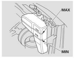
If the coolant level in the reserve tank is at or below the MIN line, add coolant to bring it up to the MAX line. Inspect the cooling system for leaks. Always use Honda All Season Antifreeze/Coolant Type 2. This coolant is pre-mixed with 50 percent antifreeze and 50 percent water. Never add straight antifreeze or plain water.
