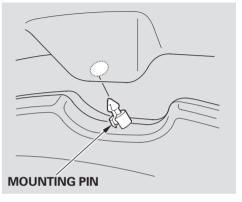
3. Pull down on the cover to remove the mounting pins from the holes in the hatch lining.
