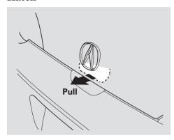
To open the hatch, pull the handle, then lift up the hatch.
