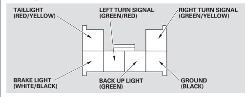
If you use a converter, you can get the connector and pins that mate with the connector in your vehicle from your dealer.
