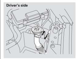
1. If you need to change the low beam headlight bulb on the driver's side, remove the neck of the windshield washer reservoir from the bracket by sliding it to the left.
