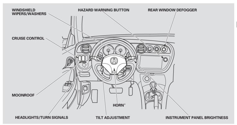
\* : To use the horn, press the center pad on the steering wheel.
