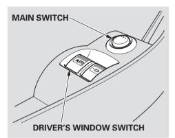
Turn the ignition switch to ON (II) to raise or lower either window. To open the window, push the switch down and hold it. Release the switch when you want the window to stop. Pull back on the switch and hold it to close the window.
