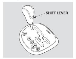
To shift from any position, move the shift lever. You cannot shift out of Park when the ignition switch is in LOCK (0) or ACCESSORY (I) position.
