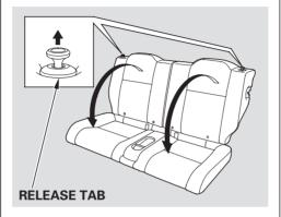
The back of the rear seat folds down to give you more cargo space. Each side folds down separately. With only half the seat folded, you can still carry a passenger in the back seat.
