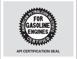
Make sure the API Certification Seal says "For Gasoline Engines".
