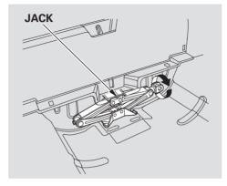
7. Turn the jack's end counterclockwise to loosen it, then remove the jack.
