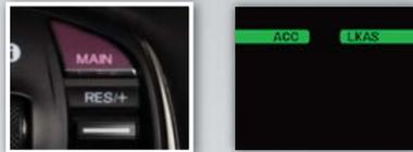
2. Press the LKAS button. Lane outlines appear in the MID. Dotted lane lines turn solid when the system operates.
