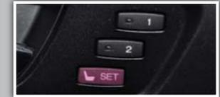
4. Press the memory button corresponding to the remote (1 or 2) you are using. You will hear two beeps.
