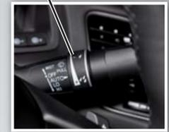
When driving in rainy weather, move the wiper lever down to the AUTO position. Adjust the rainfall sensor sensitivity with the intermittent time adjustment ring.
