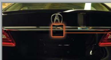
Press the trunk release button under the trunk handle when all doors are unlocked.
