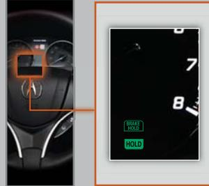
Depress the accelerator pedal to cancel brake hold and start moving.
