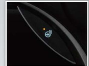
Press the heated steering wheel button to turn on heating. Press the button again to turn it off.
