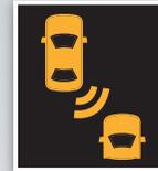
When your turn signal is on and a vehicle is detected, the blind spot indicator blinks and a beep sounds until the area is clear or the turn signal is off.
