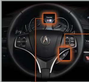
Press the Distance button to scroll through four ranges.
