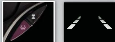
Press MAIN or the LKAS button to turn the system off.
