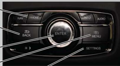
To reduce the potential for driver distraction, certain manual functions may be inoperable or grayed out while the vehicle is moving. Voice commands are always available.
