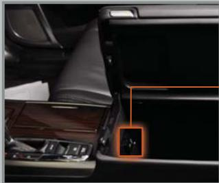
Open the center console to connect a USB flash drive or iPhone dock connector to the USB port.
