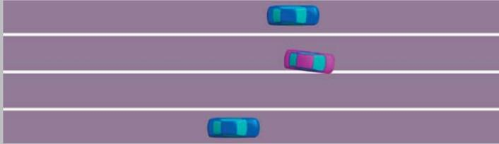
If you cross a detected lane line without using your turn signal, a message appears on the MID and a beep sounds. Steering torque is applied to keep your vehicle in the middle of the lane.
