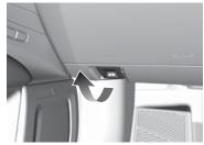
2 Locate the hood latch lever, push up the lever and lift the hood.
