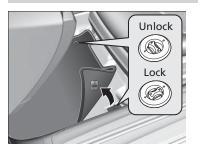
The floor mats hook over the floor anchors, which keep the mats from sliding forward. To remove the mats for cleaning, turn the anchor knobs to the unlock position. When reinstalling the mats after cleaning, turn the knobs to the lock position.
