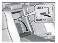
Pull the rear seat armrest down and push the button to open the cover.
