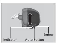
When driving after dark, the automatic dimming rearview mirror and power door mirrors\* reduce the glare from headlights behind you. Press the auto button to turn this function on and off. When activated, the auto indicator comes on.
