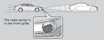
The CMBS™ activates when the speed difference between your vehicle and a vehicle detected in front of you becomes more than 10 mph (15 km/h) with a chance of a collision.
