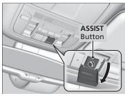
If you need to talk to the AcuraLink operator in an emergency situation, you can manually connect to them by pressing the **ASSIST** button with the power mode in ACCESSORY or ON.
