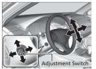
Push and hold the adjustment switch to move the steering wheel in, out, up or down.
