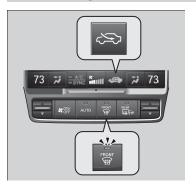
Pressing the button turns the air conditioning system on and automatically switches the system to fresh air mode.
