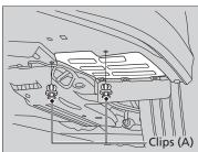
**1.** Remove the holding clips (A).
