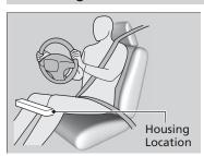
The driver's knee airbag is housed under the steering column for the driver.
