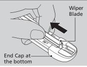
5. Pull the end of the wiper blade to the direction of the arrow in the image until it unfastens from the holder's end cap.
