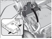
**1.** Open the fuse box cover on the positive  $\oplus$  terminal.
