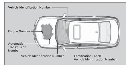
■ Vehicle Identification Number (VIN), Engine Number and Transmission Number
