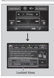
You can lock the glove box, trunk, and/or navigation\*/audio system, entering a PIN code from the On Demand Multi-Use Display<sup>TM</sup>.
