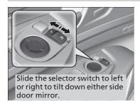
If activated, either side door mirror automatically tilts downward when you put the shift lever in  $\boxed{\mathbb{R}}$ ; this improves close-in visibility on the selected side of the vehicle when backing up. The mirror automatically returns to its original position when you shift out of  $\boxed{\mathbb{R}}$ .
