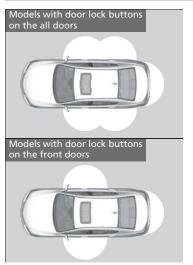
When you carry the keyless access remote, you can lock/unlock the doors and open the trunk.
