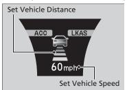
When ACC with LSF starts operating, the vehicle icon, distance bars and set speed appear on the multi-information display.
