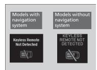
Warning buzzers may sound from inside or/ and outside the vehicle to remind you that the keyless access remote is out of the vehicle. If the buzzer continues even after the remote is put back inside, place it to be within its operational range.
