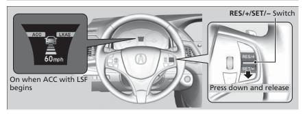
When driving at 25 mph (40 km/h) or above: Take your foot off the pedal and press down the RES/+/SET/– switch when you reach the desired speed. The moment you release the switch, the set speed is fixed, and ACC with LSF begins.
