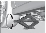
**3.** Raise the vehicle, using the jack handle bar and the jack handle, until the tire is off the ground.
