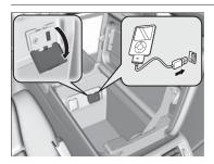
Install the iPod dock connector or the USB flash drive to the USB port.
