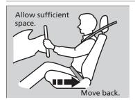
Adjust the driver's seat as far back as possible while allowing you to maintain full control of the vehicle. You should be able to sit upright, well back in the seat and be able to adequately depress the pedals without leaning forward, and grip the steering wheel comfortably. The passenger's seat should be adjusted in a similar manner, so that it is as far back from the front airbag in the dashboard as possible.
