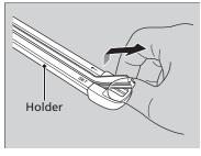
**6.** Pull the wiper blade to the opposite direction to slide it out from its holder.
