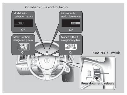
Take your foot off the pedal and press the **RES/+/SET/–** switch down when you reach the desired speed.
