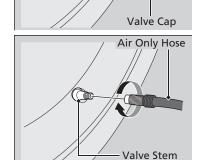
**6.** Attach the air only hose onto the tire valve stem. Screw it until it is tight.
