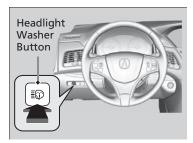
Turn the headlights on and press the headlight washer button to operate. The headlight washers also operate when you turn the windshield washers for the first time after the power mode sets to ON.
