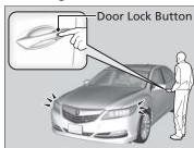
Press the door lock button on the front or rear\* door.
