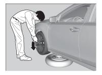
**6.** Loosen each wheel nut about one turn using the wheel nut wrench.
