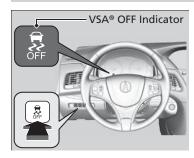
This button is on the driver's side control panel. To turn the VSA® system on and off, press and hold it until you hear a beep.
