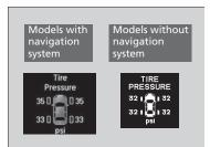
To select the tire pressure monitor, set the power mode to ON, and roll the right selector wheel until you see the tire pressure screen.
