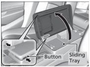
Your vehicle has a multi-function center console. It includes a storage compartment, an armrest, and a sliding tray.
