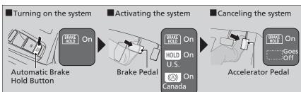
Fasten your seat belt properly, then start the engine. Press the automatic brake hold button.
