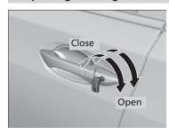
**To open:** Unlock the driver's door with the key. Within 10 seconds of returning the key to the central position, turn the key in the unlock direction and hold it there.
