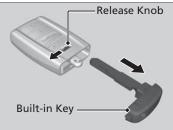
The built-in key can be used to lock/unlock the doors when the keyless access remote battery becomes weak and the power door lock/unlock operation is disabled.
