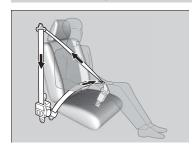
Are the motor-powered pretensioners that start to retract the front seat belts when the CMBS<sup>TM</sup>, brake assist system, or VSA® system is in operation. They may also activate when you steer the vehicle hard, or the vehicle is impacted. After retracted, the seat belts are slackened to their original positions.
