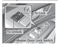
Press the master door lock switch in as shown to lock or unlock all doors.
