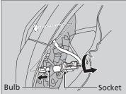
Turn the steering wheel all the way to the opposite side from the light being replaced.
