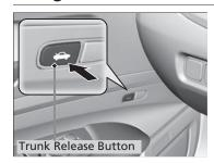
Pressing the trunk release button on the driver's door
