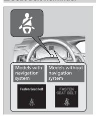
Your vehicle monitors front seat belt use. If the power mode is set to ON before the driver's seat belt is fastened, a beeper will sound and the indicator will blink. If the driver does not fasten the belt before the beeper stops, the indicator will remain on.
