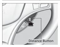
Press the (distance) button to change the ACC with LSF following distance. Each time you press the button, the following distance (the distance behind a vehicle detected ahead of you) setting cycles through short, middle, long, and extra long following distances.
