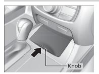
Slide the lid using release knob to use the center pocket.
