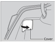
**1.** Open the trunk and remove the cover.
