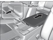
You can put small items in the sliding tray located in the console compartment lid. To use the tray, push the button, then slide the console compartment lid out fully. To close the lid, push the button. It is automatically slid back.
