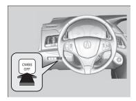
Press this button for about one second to turn on and off the system.
