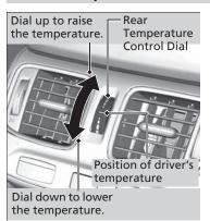
You can set the rear passenger compartment temperature different than the driver's, using the rear temperature control dial.
