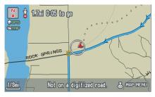
The map screen starts displaying a series of dots (breadcrumbs) to show the path you have taken if Off-road **Tracking** on the SETUP screen (Other) is set to **ON** (see page 112).
