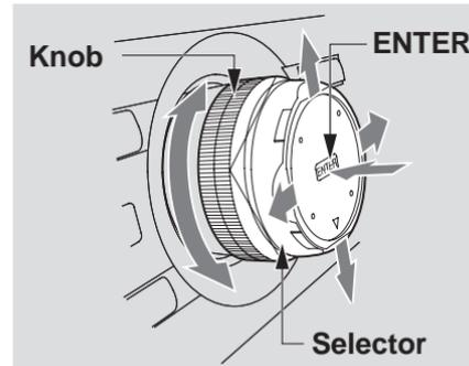
The **Interface Dial** moves left, right, up, and down. Use the **Interface Dial** to look around a displayed map. Moving the **Interface Dial** up or down can also be used to scroll up or down a page in a list. You can also rotate the **Interface Dial knob** to move the highlighting around the display or to scroll through a list. After making a selection in a menu or list, push in on the **Interface Dial (ENTER button)** to enter the selection into the system.
