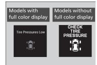
**CHECK TIRE PRESSURE/Tire Pressures Low** is displayed when a tire has significantly low pressure. The specific tire is displayed on the screen.
