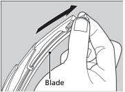
**2.** Slide the wiper blade out from the end with the indent.
