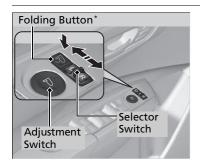
You can adjust the door mirrors when the power mode is in ON.
