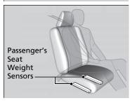
The passenger's advanced front airbag system has weight sensors.
