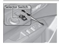
If activated, either side door mirror automatically tilts downward when you put the shift lever in  $\boxed{\mathbf{R}}$ ; this improves close-in visibility on the selected side of the vehicle when reversing. The mirror automatically returns to its original position when you shift out of  $\boxed{\mathbf{R}}$ .
