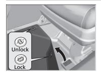
The front floor mats hook over the floor anchors, which keep the mats from sliding forward. To remove a mat for cleaning, turn the anchor knobs to the unlock position. When reinstalling the mat after cleaning, turn the knobs to the lock position.
