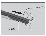
**4.** Slide the wiper blade out from its holder by pulling the tabbed end out.
