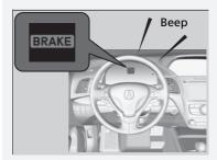
Depress the brake pedal, and keep an appropriate distance from the vehicle ahead
