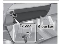
Press the button to open the glove box. You can lock the glove box with the built-in key.
