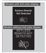
Warning buzzers may sound from inside or/ and outside the vehicle to remind you that the keyless access remote is out of the vehicle. If the buzzer continues even after the remote is put back inside, place it within its operational range.
