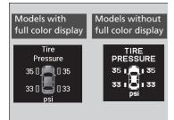
To select the tire pressure monitor, set the power mode to ON, and press the  $\boxed{\textcircled{1}}/\boxed{\textcircled{1}}$  (information) button until you see the tire pressure screen.
