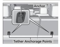
Two tether anchorage points are provided behind the rear outer seating positions and one in the ceiling for the rear center. A child seat that is installed with a seat belt and comes with a tether can use the tether for additional security.
