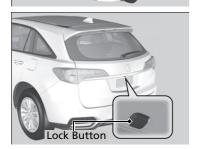
When you carry the keyless access remote, you can lock/unlock the doors and the tailgate.
