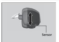
When driving after dark, the automatic dimming rearview mirror and power door mirrors\* reduce the glare from headlights behind you.
