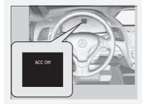
Even though ACC has been automatically canceled, you can still resume the prior set speed. Wait until the condition that caused ACC to cancel improves, then press the **DECEL/SET** button.
