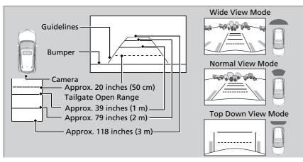
You can view three different camera angles on the rearview display. Press the selector knob to switch the angle.
