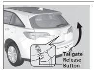
When all the doors are unlocked or press the tailgate unlock button on the remote transmitter, the tailgate is unlocked.
