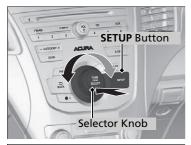
Press the **SETUP** button, and rotate  $\mathfrak{T}$  to select **Sound Settings**, then press  $\mathfrak{S}$ . Rotate  $\mathfrak{T}$  to scroll through the following choices:
