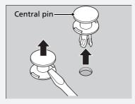
Insert the clip with the central pin raised, and push until it is flat.
