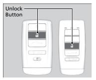
**To open:** Press the UNLOCK button twice within 10 seconds and hold it down for the second time. If the windows stop midway, repeat the procedure.
