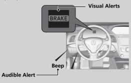
At system's earliest collision alert stage, you can change the distance (**Long/Normal/Short**) between vehicles at which alerts will come on through multi-information display setting options.
