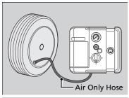
**4.** Recheck the air pressure using the air only hose on the compressor.
