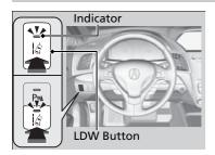
Press the LDW button to turn the system on and off.
