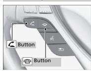
Press the (pick-up) button on the steering wheel to receive a call when *Bluetooth* Audio is playing.
