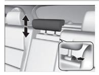
A passenger sitting in a center back seating position should adjust the height of their head restraint to an appropriate position before the vehicle begins moving.
