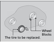
**5.** Place a wheel block or rock in front and rear of the wheel diagonal to the flat tire.
