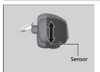
When driving after dark, the automatic dimming rearview mirror and power door mirrors\* reduce the glare from headlights behind you.
