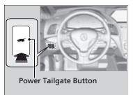
To open or close the power tailgate, press the power tailgate button on the dashboard for about one second. The beeper sounds and some exterior lights flash.
