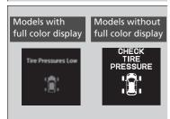
**CHECK TIRE PRESSURE/Tire Pressures Low** is displayed when a tire has significantly low pressure. The specific tire is displayed on the screen.
