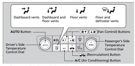
Use the system when the engine is running.
