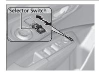
If activated, either side door mirror automatically tilts downward when you put the shift lever in  $\boxed{\mathbf{R}}$ ; this improves close-in visibility on the selected side of the vehicle when reversing. The mirror automatically returns to its original position when you shift out of  $\boxed{\mathbf{R}}$ .
