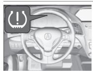
Monitors the tire pressure while you are driving. If your vehicle's tire pressure becomes significantly low, the low tire pressure/TPMS indicator comes on and a message appears on the multi-information display.
