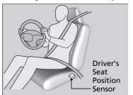
The driver's advanced front airbag system includes a seat position sensor.
