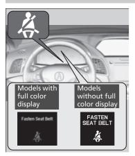
Your vehicle monitors front seat belt use. If the power mode is set to ON before the driver's seat belt is fastened, a beeper will sound and the indicator will blink. If the driver does not fasten the belt before the beeper stops, the indicator will remain on.
