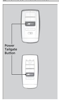
Press the power tailgate button for more than one second to operate.
