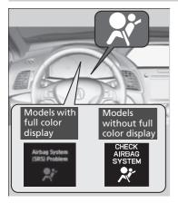
When the power mode is set to ON The indicator comes on for a few seconds, then goes off. This tells you the system is working properly.
