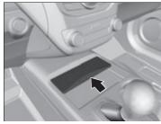
Slide the lid using the release knob to open or close the console compartment.
