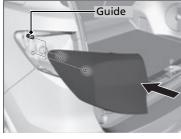
**6.** Reinstall the light assembly by sliding it on to the guide on the body.
