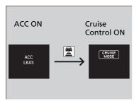
Press and hold the (distance) button for one second. **Cruise Mode Selected** appears on the driver information interface for two seconds, and then the mode switches to Cruise.
