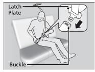
**3.** Insert the latch plate into the buckle. Properly fasten the seat belt the same way you fasten the lap/shoulder seat belt.
