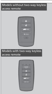
Use the keyless access remote to start and stop the engine, and to lock and unlock all the doors and tailgate. You can also use the keyless access system to lock and unlock the doors and tailgate.
