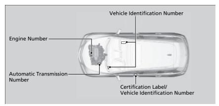
■ Vehicle Identification Number (VIN), Engine Number and Transmission Number
