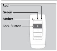
You can remotely check if your vehicle's doors are all locked or any are unlocked using the keyless access remote from extended distances
