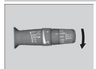
When you push the lever down to **AUTO**, the windshield wipers sweep once, and go into the automatic mode.
