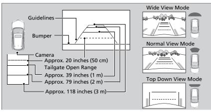
You can view three different camera angles on the rearview display. Press the selector knob to switch the angle.
