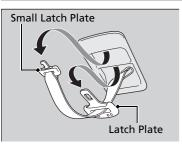
**1.** Pull out the seat belt's small latch plate and the latch plate from each holding slot in the ceiling.
