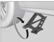
image) clockwise until the top of the jack contacts the jacking point.
