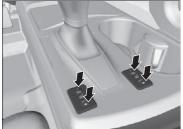
While in HI, the heater cycles on and off.
