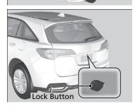
When you carry the keyless access remote, you can lock/unlock the doors and the tailgate.
