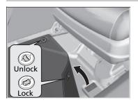
The front floor mats hook over the floor anchors, which keep the mats from sliding forward. To remove a mat for cleaning, turn the anchor knobs to the unlock position. When reinstalling the mat after cleaning, turn the knobs to the lock position.
