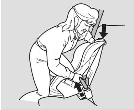
4. Confirm that the belt is locked, then grab the shoulder part of the belt near the buckle, and pull up to remove any slack from the lap part of the belt. Remember, if the lap part of the belt is not tight, the child seat will not be secure.
