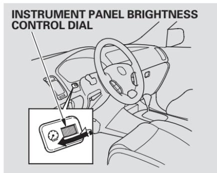
The dial on the instrument panel controls the brightness of the instrument panel lights. Turn the dial to adjust the brightness.
