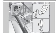
Install the iPod® or iPhone® dock connector or the USB flash drive to the USB port.
