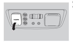
Open the outlet cover and insert the cable.
