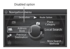
Certain manual functions are disabled or inoperable while the vehicle is in motion. You cannot select a grayedout option using the Interface Dial until the vehicle is stopped.
