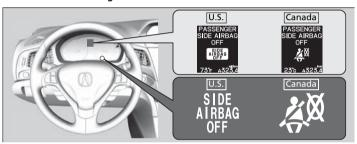
This indicator comes on if the passenger's side airbag has been turned off because the passenger is too small to be sitting in the front seat, is slouching or not sitting upright, or has leaned into the airbag's deployment path.
