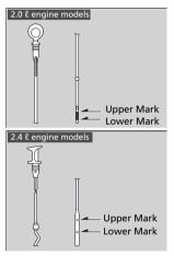
**4.** Remove the dipstick again, and check the level. It should be between the upper and lower marks. Add oil if necessary.
