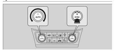
You can set the temperature synchronously for the driver side and the passenger side in synchronized mode.
