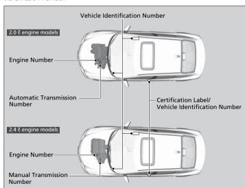
The interior vehicle identification number (VIN) is located under the cover.
