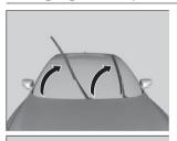
**1.** Lift the driver side wiper arm first, then the passenger side.
