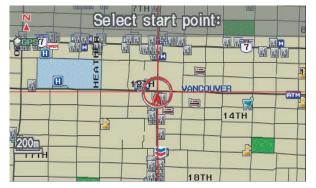
Use the **ZOOM** buttons to select the map scale (available scales are 80, 200, and 400 metre scales). Use the joystick to move the crosshairs (red circle) to the desired start point and push in the joystick to "set" the start point. Then move the joystick in a straight or diagonal direction to encompass the area to be avoided
