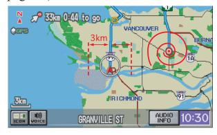
For "Places Along the Route," the system looks in front of you within a corridor width specified by your values for "On Highways" or "On Surface Street." The system checks the upcoming area, based on your input.
