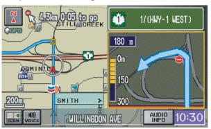
On the map screen, the location of the manoeuvre is marked with a small yellow square. The guidance window is simply an enlargement of the area indicated by the yellow square. After you complete the manoeuvre, the display returns to a full map screen when the single-screen mode is set, or to a map and direction list screen when the split-screen mode is set.
