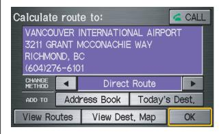
Say or select **OK**. The system calculates the route using the method shown on the screen (see *Map Screen* on page 48).
