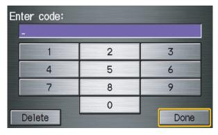
Enter the four-digit security code, then select **Done**. If you have entered it correctly, the display changes to the Disclaimer screen. If you make a mistake, the system will display "incorrect PIN." Re-enter your 4-digit security code. You have 10 chances to enter the correct code. If all 10 are incorrect, turn the ignition to OFF, then back to ON (II) to have 10 more chances to enter the correct code.
