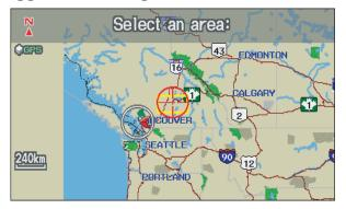
Use the joystick to move the crosshairs to the area of the province close to your intended destination. If desired, use the **ZOOM** buttons to change the map scale. When you have the crosshairs in the desired area, push in on the joystick. The address of the location you have selected will appear at the top of the screen.
