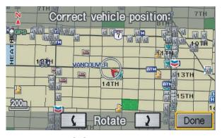
3. Use the **ZOOM** buttons and the joystick to move the location arrowhead to the correct location. Touch the arrow buttons on the bottom of the screen to rotate the direction arrows so the vehicle position is pointing in the correct direction.
