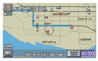
The map screen starts displaying a series of dots (breadcrumbs) to show the path you have taken if **Off-road Tracking** on the Setup screen (second) is set to **On** (see page 90).
