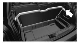
Fold up the cargo floor panel in the lower position and push it behind the locks on the left and right, arrow. You've reached the maximum cargo height.
