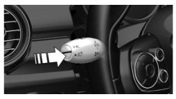
The High-beam Assistant can be activated when the low beams are activated.
