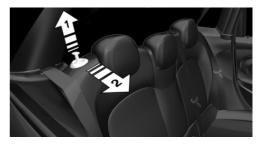
Pull the release upward and fold the backrest toward the front.
