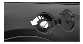
Place the tank lid in the bracket attached to the fuel filler flap.
