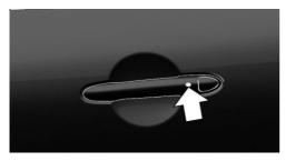
Press and hold down the handle of the driver or the front seat passenger.
