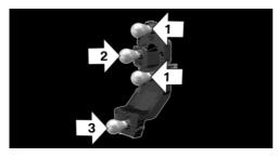
Proceed in the reverse order to insert the new bulb and attach the bulb holder. Make sure that the bulb holder engages in all fasteners.
