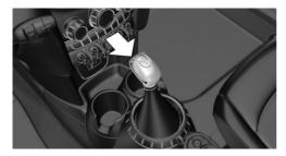
Press button on the front of the selector lever, arrow.
