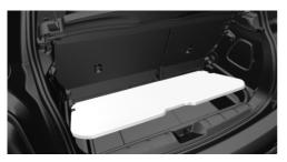
Grasp the cargo floor panel in the rear and fold slightly upward. Next, pull it backward from the supports.
