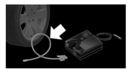
3. Attach the connection hose to the connector of the sealant container, ensuring that it engages audibly.
