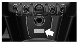
The USB interface is located in the front of the center console.
