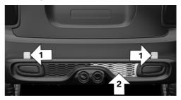
The anchorage points, arrow 1, and the socket, arrow 2, are located below the covers in the bumper.
