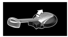
3. Slide the key in the cover of the battery compartment and raise the cover, arrow.
