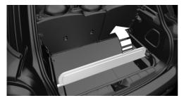
On 5-door models: To change the position of the cargo floor panel, first fold up the rear part of the cargo floor panel.
