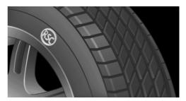
RSC label on the tire sidewall.
