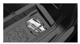
The onboard vehicle tool kit is located in the trough under the cargo area floor.
