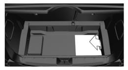
The screw-in tow fitting should always be carried in the vehicle. It can be screwed in at the front or rear of the MINI. It is located under the
