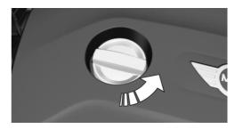
Only replenish the maximum engine oil amount of 1 US quart/liter if the signal is displayed in the instrument cluster.
