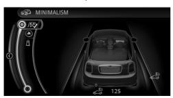
Color code green, arrow 1: distance traveled in the Coasting driving condition. Symbol, arrow 2: coasting driving condition.
