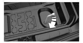
Unlock the locking hexagon of the emergency wheel well using the hexagon attached to retaining plate.
