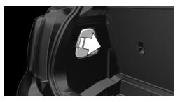
Through the opening, loosen the plug connector, arrow 2 on the bulb holder.
