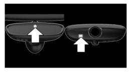
Photocells are used for control:
