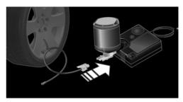
4. Slide the sealant container upright into the holder on the compressor housing, ensuring that it engages audibly.
