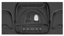
The indicator lamp for the front-seat passenger airbags indicates the operating state of the front-seat passenger airbags.
