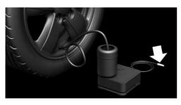
6. With standby state switched on or the engine running, switch on the compressor.
