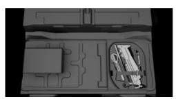
The onboard vehicle tool kit is located in the trough under the trunk floor.
