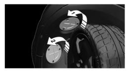
Unscrew the inner lid counterclockwise, and remove it.
