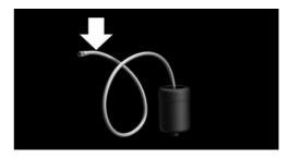
Slide the sealing container into the holder on the compressor housing, ensuring that it engages audibly.
