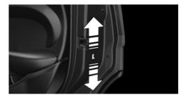
Push the locking lever on the rear doors up. The door can now be opened from the outside only.
