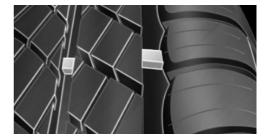
Wear indicators are distributed around the tire's circumference and have the legally required minimum height of 0.063 inches/1.6 mm.
