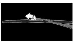
Pull the wiper blade down first out of the holder on the wiper arm, arrow 1.
