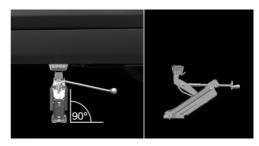
Crank up the vehicle jack until the entire surface of the jack is in contact with the ground and the wheel in question is raised a maximum of 1.2 inches/3 cm off the ground.
