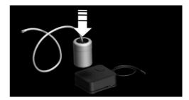
Screw the filling hose of the sealant container onto the tire valve of the nonworking wheel.
