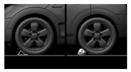
If you need to change a wheel on a slight downhill gradient, place chocks or other suitable objects, for example a rock, under the wheels of both the front and rear axles.
