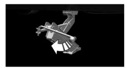
4. When extending the vehicle jack, ensure that the foot of the vehicle jack is posi-
