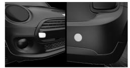
Threaded holes for the tow fitting are located in the front and rear of the vehicle on the right side with respect to the direction of travel.
