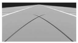
Turning circle lines can be superimposed on the image of the rearview camera.
