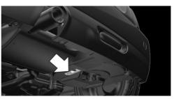
Located behind the bumper on the underside of the vehicle is an opening for checking the tire inflation pressure.
