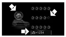
The display of the MINIMALISM Analyser consists of a fish, which is riding along in a glass of water on the roof of the MINI and a table of values that rates the driving style in various categories. The bonus range achieved by driving style that minimizes fuel consumption is displayed below the table of values.
