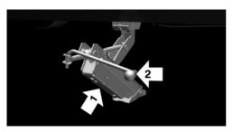
Insert the vehicle jack into the rectangular recess of the jacking point which is nearest to the wheel that you are changing.
