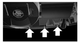
Push the heat shield forward and the bumper back in order to be able to reach the fog lamp. Turn the bulb socket counterclockwise and remove.
