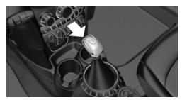
To release the lock: with the brake pedal depressed, press the button on the front of the selector lever, see arrow.
