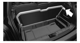
Fold up the cargo floor panel in the lower position and push it behind the locks, arrow.
