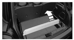
On 5-door models: To change the position of the cargo floor panel, first fold up the rear part of the cargo floor panel.
