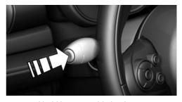
Press and hold button on blinker lever.
