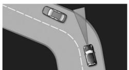
If the desired speed is too high for a curve, the speed is reduced slightly, although curves can-
