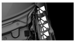
3. Turn the bulb holder counterclockwise and remove.
