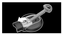
Using a pointed object, press battery in direction of arrow and lift it out.
