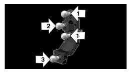
Proceed in the reverse order to insert the new bulb and attach the bulb holder. Make sure that the bulb holder engages in all fasteners.
