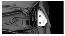
Loosen nuts of the cover by hand and remove the cover.
