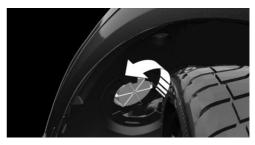
Pull bulb holder out of the bulb housing; if needed, loosen it with small tilting movements if possible.
