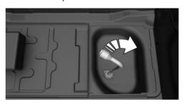
Unlock the locking hexagon of the emergency wheel well using the hexagon attached to retaining plate.
