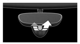
To reduce the blinding effect of the interior rear view mirror, flip the lever forward.
