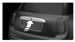
Without Comfort Access: unlock the vehicle.Press button next on tailgate.
