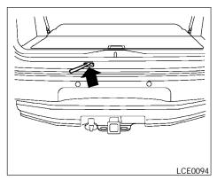
4. Assemble the two pieces of the jack rod. Find the oval-shaped opening above the middle of the license plate. Pass the T-shaped end of the jack rod through the opening and direct it toward the spare tire winch, located directly above the spare tire.
