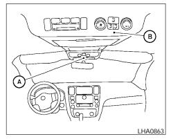
Rear seat temperature and fan speed can be controlled from both the front seat overhead console controls (a) or the rear seat overhead console controls (b).
