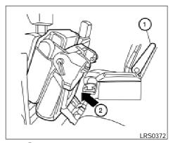
Then (2) lift up on the lower corner of the seat base and tip the 2nd row captain's chair forward. To exit the 3rd row bench seat, lift up on the same latch and fold the seatback forward onto the seat base. Then lift up on the seat base and tip it forward.
