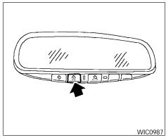
3. Using both hands, simultaneously press and hold both the HomeLink® button you want to program and the hand-held transmitter button.
