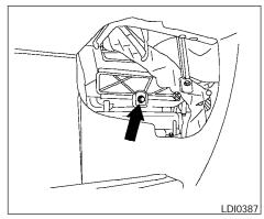
Remove the filter cover bolt and remove the filter cover.
