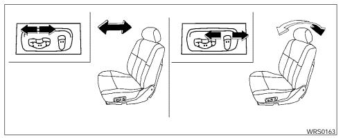
belt fit (see "Precautions on seat belt usage" later in this section). Also, the seatback can be reclined to allow occupants to rest when the vehicle is stopped and the transmission is in P (Park).
