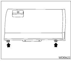
1. Remove the 2 lower glove box screws.
