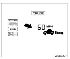
To set cruising speed, accelerate your vehicle to the desired speed, push the COAST/SET switch and release it. (Vehicle ahead detection indicator, set distance indicator and set vehicle speed indicator come on.) Take your foot off the accelerator pedal. Your vehicle will maintain the set speed. The CRUISE indicator light in the vehicle information display remains on.
