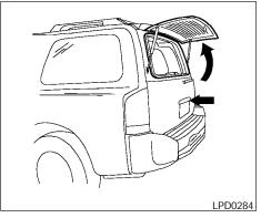
To open, push the button up on the smaller outside handle to release the glass hatch, then pull up on the glass hatch. To close, lower and push the glass hatch down securely.
