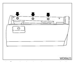
Open the glove box, then remove the three upper glove box screws. Remove the glove box assembly from the instrument panel to access the in-cabin microfilter cover.
