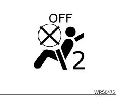
7. If the booster seat is installed in the front passenger seat, turn the ignition switch to the ON position. The front passenger air bag status light a may or may not illuminate, depending on the size of the child and the type of booster seat being used. See "Front passenger air bag and status light" later in this section.
