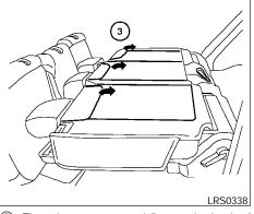
There is a carpet panel flap on the back of each seat that can be folded toward the back of the vehicle.
