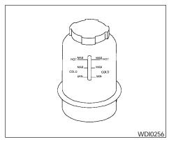
The fluid level should be checked using the HOT MAX range on the power steering fluid reservoir at fluid temperatures of 122° - 176°F (50° - 80°C) or using the COLD MAX range on the power steering fluid reservoir at fluid temperatures of 32° - 86°F (0° - 30°C).
