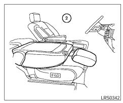
② Once the seatback is released it will enable you to fold the front passenger seatback flat over the seat cushion. To return the front passenger's seat to a seating position, move the recline switch backward until the desired angle is obtained.
