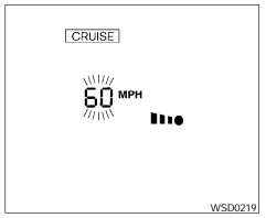
When passing another vehicle, the set speed indicator will flash when the vehicle speed exceeds the set speed. The vehicle detect indicator will turn off when the area ahead of the vehicle is open. When the pedal is released, the vehicle will return to the previously set speed. The CRUISE indicator light will appear on the vehicle information display.
