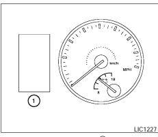
The vehicle information display (1) is located to the left of the speedometer. It displays such items as:
