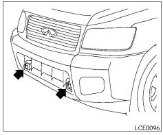
VEHICLE RECOVERY (freeing a stuck vehicle)
