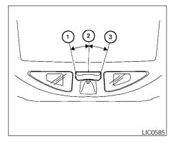
The interior light has a three-position switch and operates regardless of ignition switch position.
