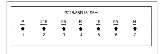
7. H: Tire speed rating. You should not drive the vehicle faster than the tire speed rating.
