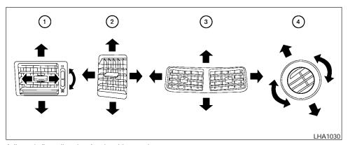
Adjust air flow direction for the driver and passenger side ①, center ②, and rear passenger 3 and 4 vents by moving the vent slide and/or vent assemblies.
