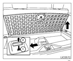
To access the floor storage area, push down (1) to raise the handle, then pull up on the handle (2) to lift the luggage board.
