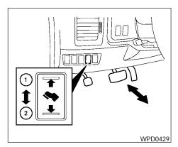
The accelerator and brake pedals can be adjusted for driving comfort.
