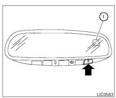
Push the  $-\stackrel{\$}{N}$ - button for about 1 second when the ignition switch is in the ON position to toggle the compass display ① on or off. The display will indicate the direction of the vehicle's heading.
