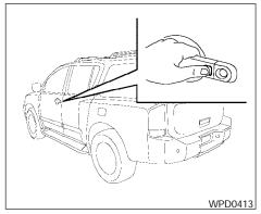
If a door handle is pulled while unlocking the doors, that door may not be unlocked. Returning the door handle to its original position will unlock the door. If the door does not unlock after returning the door handle, push the door handle request switch to unlock the door.
