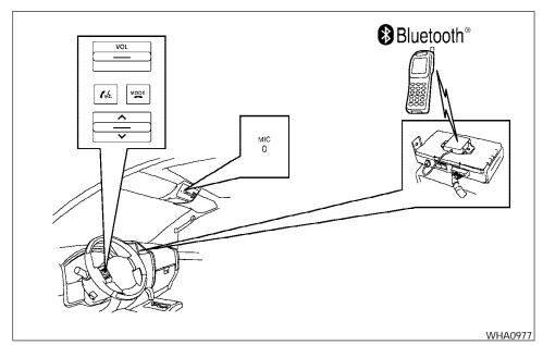
Your INFINITI is equipped with the Bluetooth® Hands-Free Phone System. If you have an approved Bluetooth® enabled cellular phone, you can set up the wireless connection between your cellular phone and the in-vehicle phone module. With Bluetooth® wireless technology, you can
