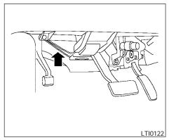
2. Apply the parking brake to access the jumper harness connector.
