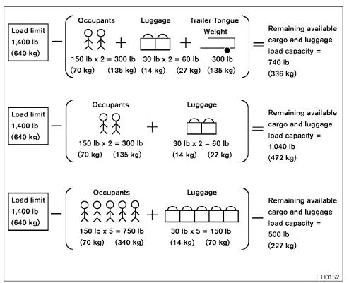
Steps for determining correct load limit
