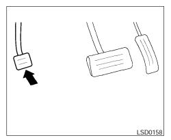
**To engage:** Firmly depress the parking brake.
