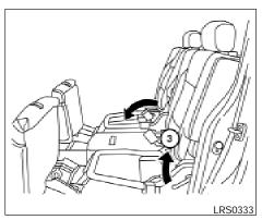
Then lift up on the recline lever to fold the seatback flat forward.
