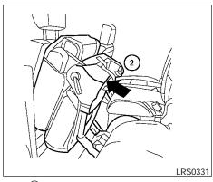
Then ② lift up on the lower corner of the seat base and tip the outboard seating position of the 2nd row bench seat forward. To exit the 3rd row bench seat, lift up on the same latch and fold the seatback forward onto the seat base. Then lift up on the seat base and tip it forward.
