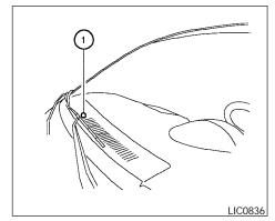
Be sure you do not put anything on top of the autolight sensor (1) located in the top side of the instrument panel. The autolight sensor controls the autolight: if it is covered, the autolight sensor reacts as if it is dark out and the headlights will illuminate. If this occurs while parked with the engine off and the key in the ON position, your vehicle's battery could become discharged.
