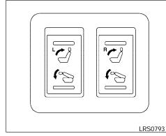
To fold down the 3rd row seats, press and hold the bottom portion of the switch.
