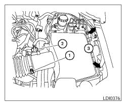
The air cleaner filter should not be cleaned and reused. Replace it according to the maintenance log shown in your "INFINITI Service and Maintenance Guide." When replacing the filter, wipe the inside of the air cleaner filter housing and the cover with a damp cloth.
