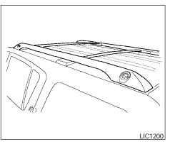
The crossbars can be adjusted forward and backward. Loosen the thumbwheel (1) and adjust the crossbar to the desired position. Tighten the thumbwheel. Place your luggage on the bars and secure the luggage with rope to the utility loops (2). Do not place luggage on the side rails or tie rope directly to the side rails. Always be sure the thumbwheels are fully tightened to keep the crossbar in place. Do not use utility loops for any purpose other than securing luggage.
