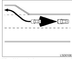
When driving on some roads, such as winding, hilly, curved, narrow, or roads which are under construction, the ICC sensor may detect vehicles in a different lane, or may temporarily not detect a vehicle traveling ahead. This may cause the ICC system to decelerate or accelerate the vehicle.
