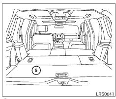
The carpet panel flaps provide a level cargo floor when the 3rd row seats are also folded flat. Reverse this process to return the 2nd row captain's chairs to a seating position. Make sure to properly raise the seatback to an upright position and push the seat cushion down into place.
