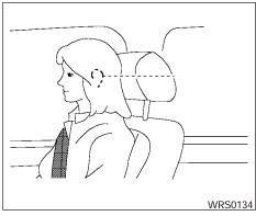
Adjust the head restraint so the center is level with the center of your ears.
