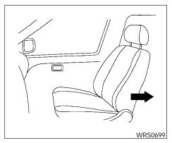
If you must install a booster seat in the front seat, move the seat to the rearmost position.
