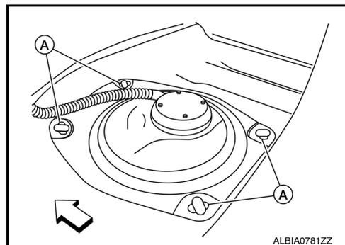
10. Disconnect the fuel level sensor, fuel filter, and fuel pump assembly harness connector (A), EVAP hose connector (C), and the fuel feed hose connector (B) from the fuel level sensor unit, fuel filter, and fuel pump assembly.
