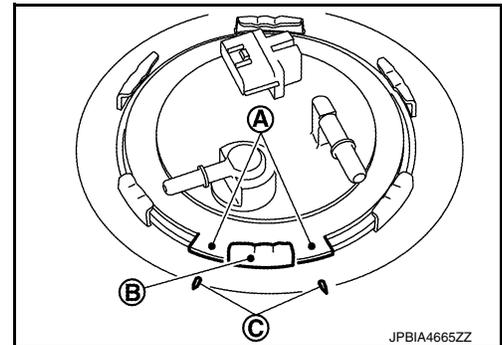
12. Raise the fuel level sensor, fuel filter, and fuel pump assembly high enough to gain access and disconnect the transfer tube connector (A).
