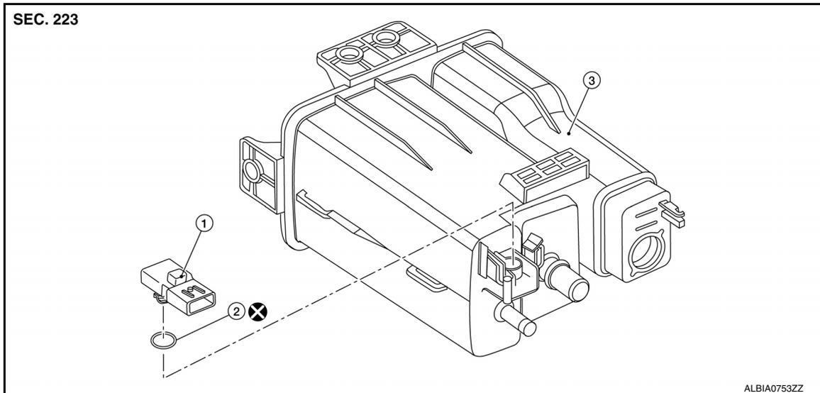
1. EVAP control system pressure sensor 2. O-ring 3. EVAP canister
