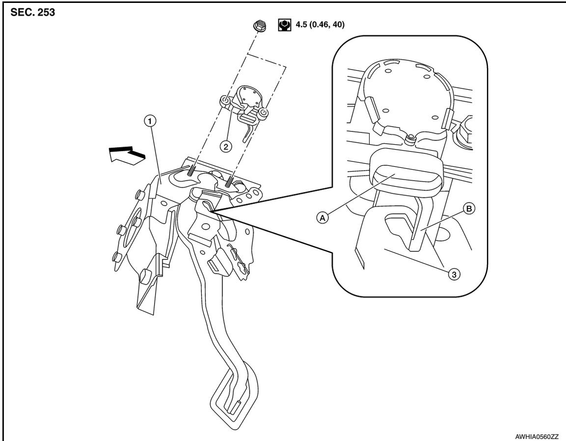
1. Brake pedal assembly      2. Brake pedal stroke sensor      3. Brake pedal sensor bracket
