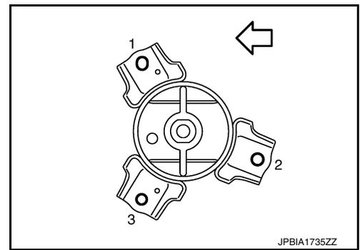
15. Remove the engine mount insulator (front).
