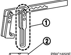
Disassembling valve mechanism<br>Part (1) is a component of KV10116200 (J-26336-A), but part (2) is not.                                                                                                                                               |
