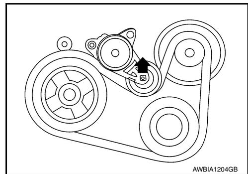
4. Insert a rod approximately 6 mm (0.24 in) in diameter through the rear of drive belt auto-tensioner into retaining boss to lock drive belt auto-tensioner pulley.
