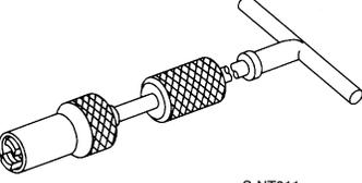
Removing valve oil seal                                                                                                                                                                                                                                |
