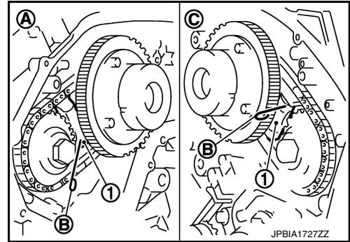
6. Install the crankshaft sprocket on the crankshaft.
