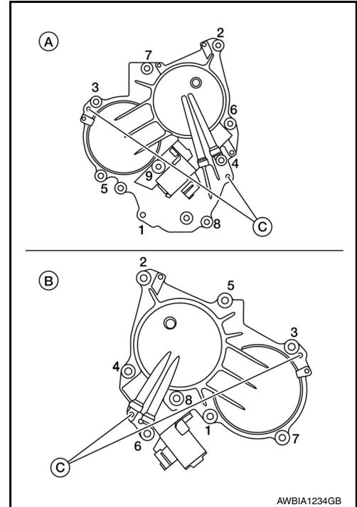
9. Install the water pump. Refer to [CO-19, "Removal and Installation"](#).
