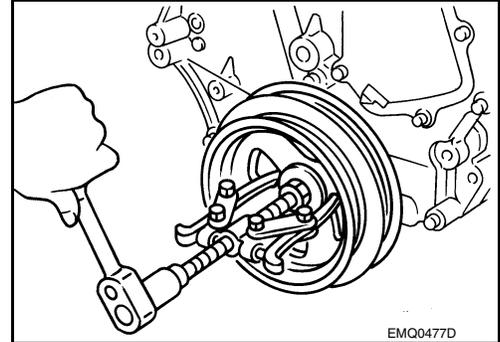
4. Remove front oil seal from front cover using a suitable tool.
