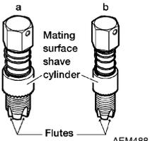
Reconditioning the exhaust system threads before installing a new oxygen sensor (Use with anti-seize lubricant shown below.)<br><b>a: J-43897-18 (18 mm dia.) for zirconia oxygen sensor</b><br><b>b: J-43897-12 (12 mm dia.) for titania oxygen sensor</b> |
