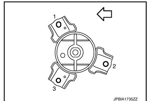
3. Install the engine mount bracket (front) to the engine block.
