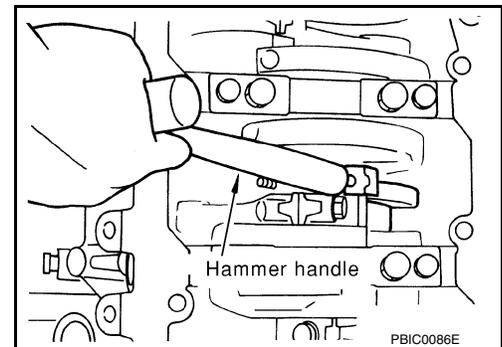
13. Remove the connecting rod bearings.
