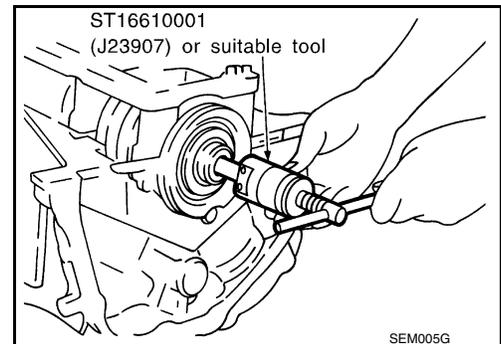
4. Cut away liquid gasket and remove rear oil seal retainer using Tool. Refer to [EM-4, "Precaution for Liquid Gasket"](#).
