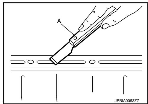
3. Attach the liquid gasket tube to the suitable tool.
