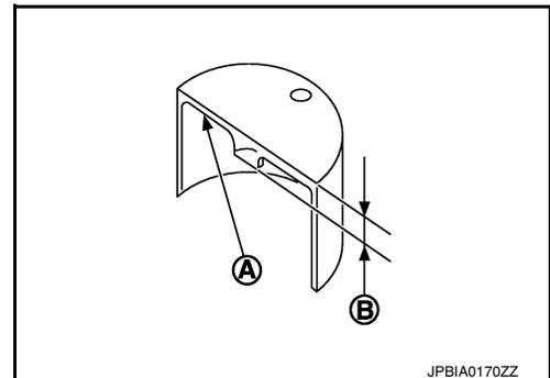
5. Install the selected replacement valve lifter.
