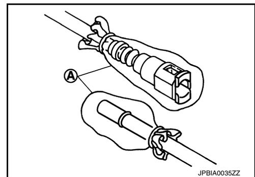
6. Disconnect harness connector from fuel injector.
