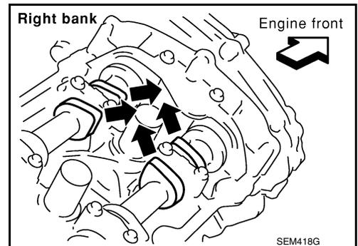
11. Remove the water pump. Refer to [CO-19. "Removal and Installation"](#).
