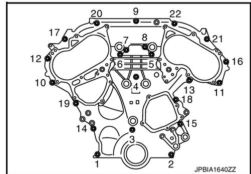
8. Install intake valve timing control cover RH and intake valve timing control cover LH.
