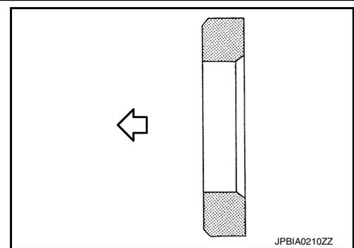
23. Install the rear oil seal retainer using Tool (A).
