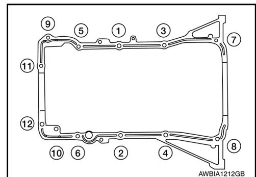
7. Install the lower oil pan. Refer to [EM-36. "Removal and Installation \(Lower Oil Pan\)"](#).
