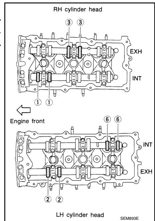
a. Using a feeler gauge, measure the clearance between the valve lifter and camshaft.
