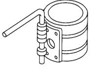
Installing piston assembly into cylinder bore                                                                                                                                                                                                        |
