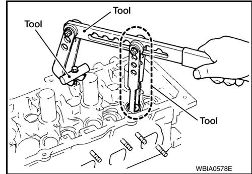
5. Remove valve oil seal using Tool.
