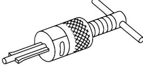
Removing crankshaft pilot bushing                                                                                                                                                                                                                    |
