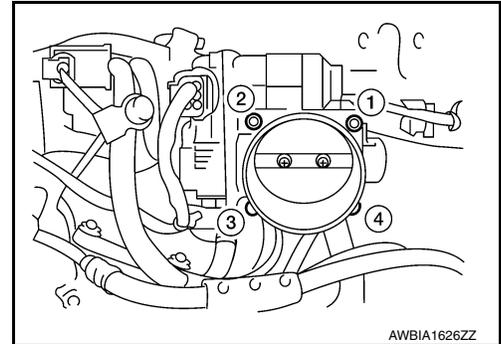
12. Remove the VIAS control solenoid valve as necessary.
