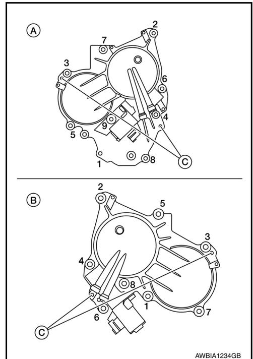
21. Remove the front timing chain case.
