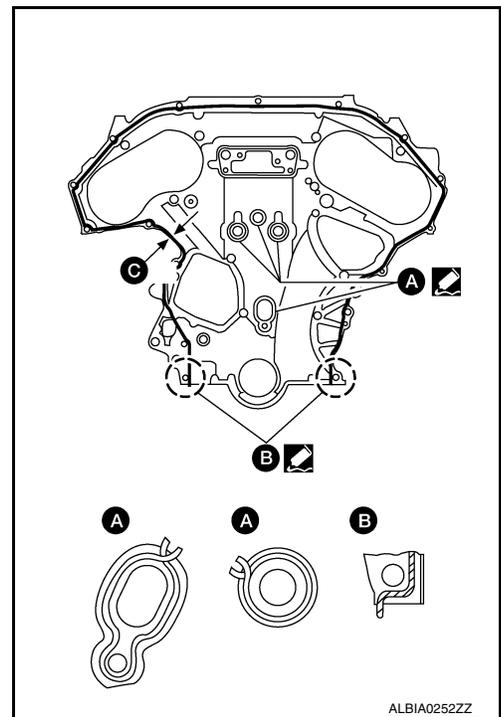
5. Install the front timing chain case by aligning the dowel pin on the rear timing chain case with the dowel pin hole in front timing chain case.
