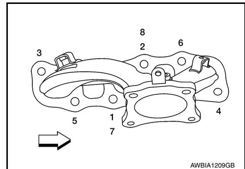
14. Remove the exhaust manifold (RH).
