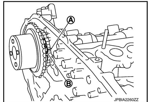
4. After confirming the mating marks are aligned, tighten the camshaft sprocket bolts.
