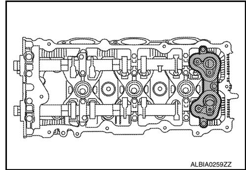
3. Remove the intake and exhaust camshaft brackets and the camshafts.
