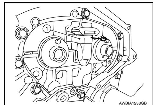
5. Install valve lifter, if removed.
