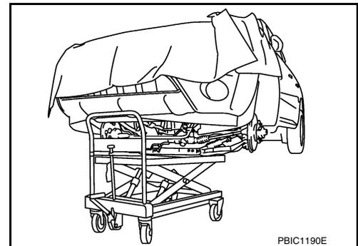
2. Remove front suspension member mounting nuts and bolts. Refer to [FSU-7, "Exploded View"](#).
