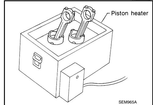
c. Push out the piston pin with a suitable tool with an outer diameter of approximately 20 mm (0.8 in).
