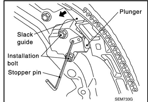
8. Remove internal chain guide, tension guide and slack guide.
