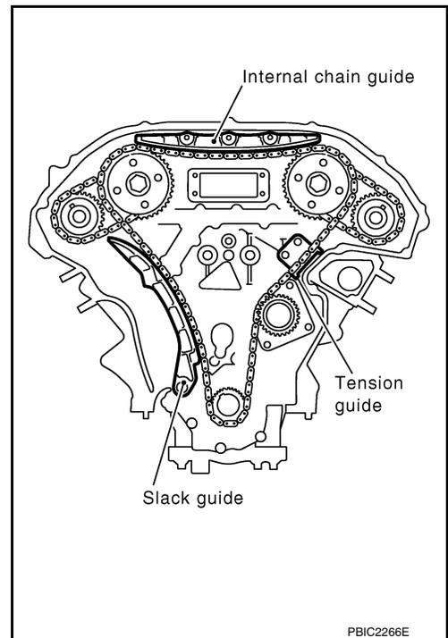
9. Remove timing chain (primary) and crankshaft sprocket.
