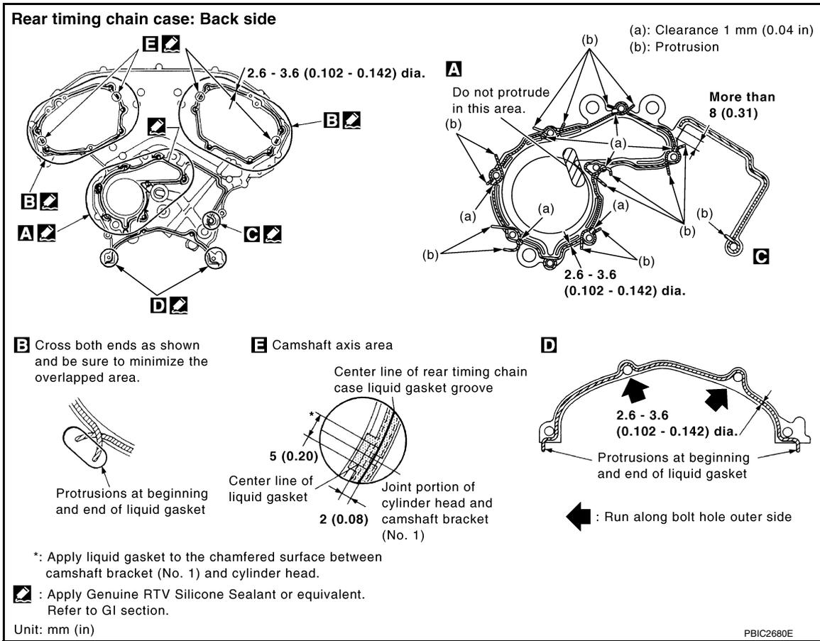
3. Align the rear timing chain case and water pump assembly with the dowel pins (RH and LH) on the cylinder block and install the case. Make sure the O-rings stay in place during installation.
