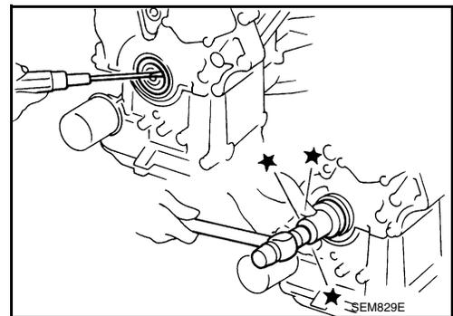
24. Remove all old liquid gasket from all the bolt holes and bolts.
