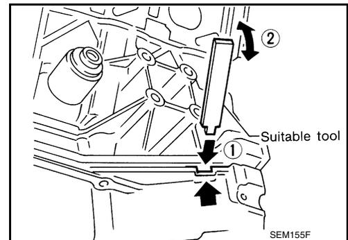
13. Remove the O-ring seals from the bottom of the cylinder block and oil pump housing. Use new O-rings for installation.
