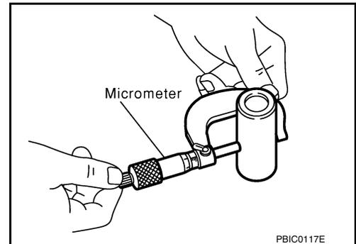
Connecting Rod Bushing Oil Clearance (Small End)
