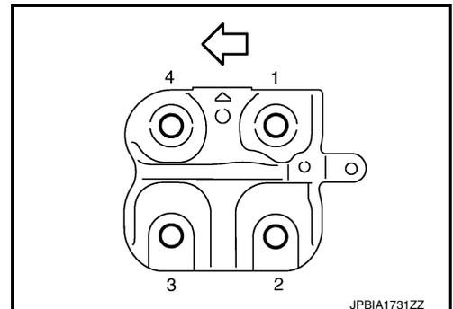
13. Remove the engine mount bracket (front).
