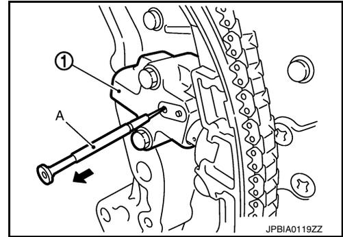
10. Reconfirm that the matching marks on the sprockets and the timing chain have not slipped out of alignment.
