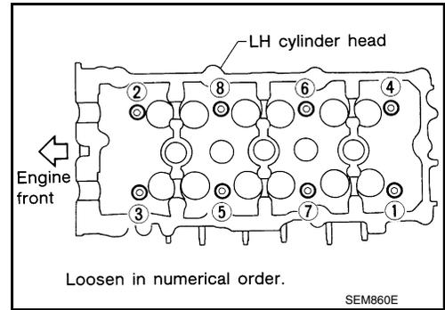
8. Remove cylinder heads and gaskets.
