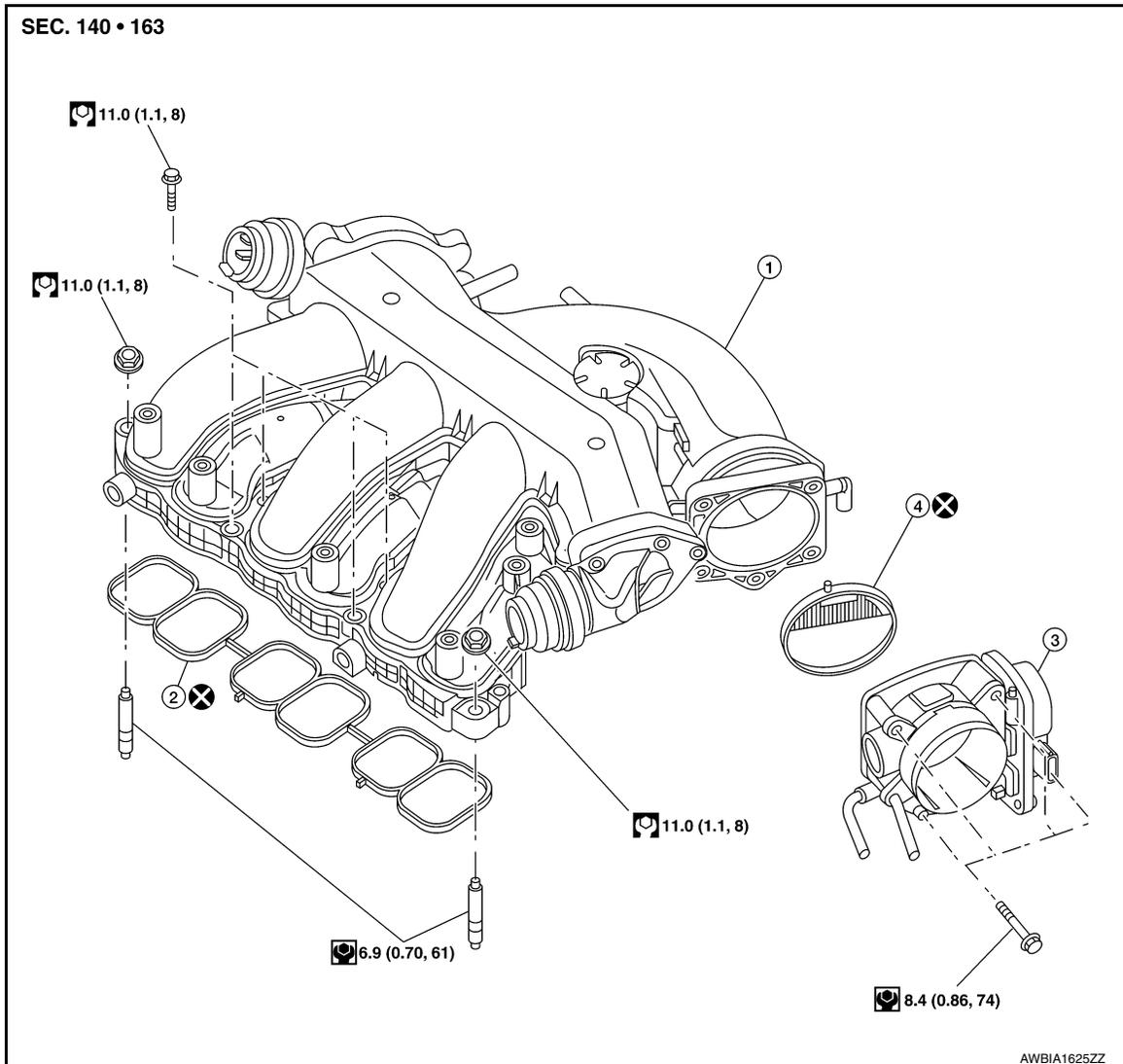
1. Intake manifold collector
