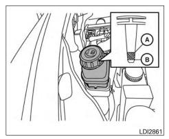
Check the fluid level in the reservoir.
