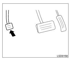
**To engage:** Firmly depress the parking brake.
