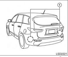
The BSW system uses radar sensors (1) installed near the rear bumper to detect other vehicles in an adjacent lane.
