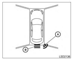
When the corner of the vehicle moves closer to an object, the corner sonar indicators (A) appears. When the center of the vehicle moves close to an object, the center sonar (if so equipped) indicator (B) appears.
