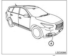
The FEB system uses a radar sensor (A) located behind the lower grille of the front bumper to measure the distance to the vehicle ahead in the same lane.
