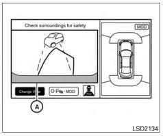
If the radar detects an approaching vehicle from the side, the system chimes a sound (single beep), the Blind Spot Warning indicator light on the side of the approaching vehicle flashes and a yellow rectangular frame appears in display (A).
