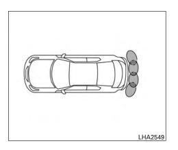
The Camera Aiding Sonar (parking sensor) sounds a tone to inform the driver of obstacles. near the bumper.
