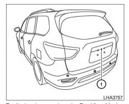
To display the rear view, the RearView Monitor system uses a camera located just above the vehicle's license plate  $\widehat{\mathbb{T}}$ .
