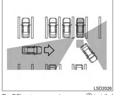
The BCI system uses radar sensors (1) installed on both sides near the rear bumper to detect an approaching vehicle and sonar sensors to detect objects in the rear.
