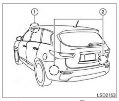
The BSI system uses a camera 1 installed behind the windshield to monitor the lane markers of your traveling lane and radar sensors 2 installed near the rear bumper to detect other vehicles in an adjacent lane.
