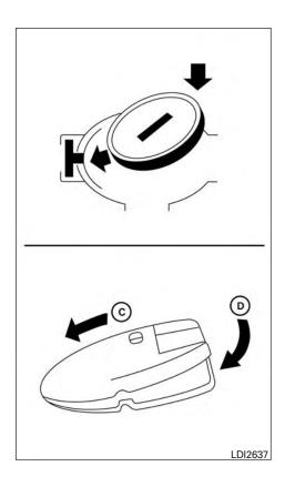
3. Replace the battery with a new one.
