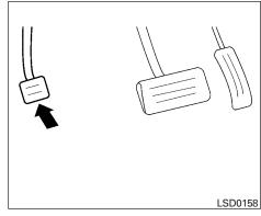
To engage: Firmly depress the parking brake.
