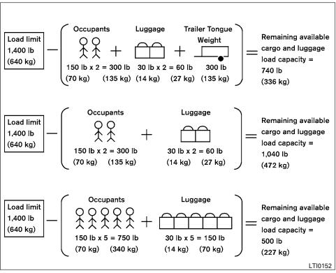
Steps for determining correct load limit
