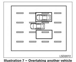
Illustration 7: If the BSI system is on and your vehicle approaches a lane marker while another vehicle is in the detection zone the system chimes a sound (three times) and the BSW indicator light flashes. Then, the BSI system slightly applies the brakes on the appropriate side to help return the vehicle back to the center of the driving lane.
