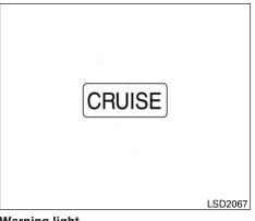
If it is not possible to set or the indicator stays on, it may indicate that the system is malfunctioning. Although the vehicle is still driveable under normal conditions, have the vehicle checked. It is recommended that you visit an INFINITI retailer for this service.
