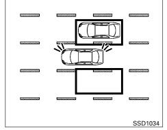
Illustration 6 - Overtaking another vehicle Illustration 6: If the driver activates the turn signal while another vehicle is in the detection zone. then the system chimes a sound (twice) and the BSW indicator light flashes.
