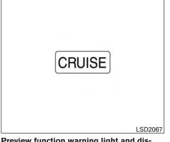
If the indicator stays on, it may indicate that the Preview Function is malfunctioning (the brake is operative). Although the vehicle is still driveable under normal conditions, have the vehicle checked. It is recommended that you visit an INFINITI retailer for this service.
