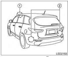
The BSI system uses a camera 1 installed behind the windshield to monitor the lane markers of your traveling lane and radar sensors (2) installed near the rear bumper to detect other vehicles in an adiacent lane.
