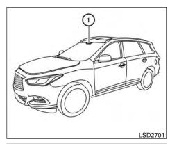
cated above the inside mirror. When the camera unit detects that the vehicle is traveling close to either the left or the right of the traveling lane, the LDW indicator light on the instrument panel blinks in orange and a warning chime sounds.
