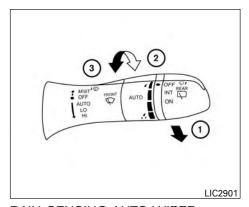
RAIN-SENSING AUTO WIPER SYSTEM (if so equipped)
