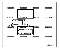
Illustration 2 - Approaching from behind Illustration 2: If the driver activates the turn signal then the system chimes a sound (twice) and the Blind Spot Warning indicator light flashes.
