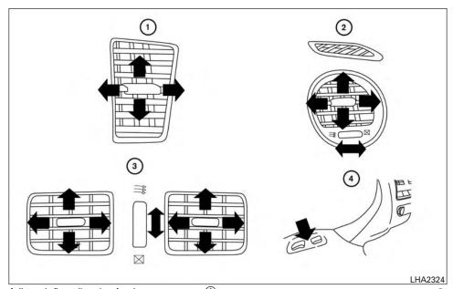
Adjust air flow direction for the center vents (1), driver's and passenger's side vents 2, and rear vents (3) by moving the vent slide and/or vent assemblies.
