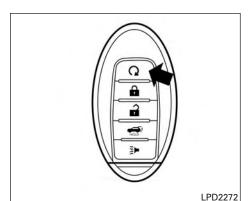
button will be on the INFINITI Intelligent Key if the vehicle has remote engine start. This feature allows the engine to start from outside the vehicle.
