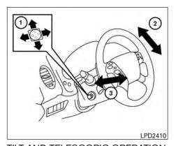
TILT AND TELESCOPIC OPERATION To adjust the steering wheel move the switch (1) in the following directions:
