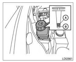
Check the fluid level in the reservoir.
