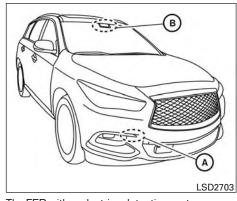
The FEB with pedestrian detection system uses a radar sensor (A) located behind the lower grille of the front bumper to measure the distance to the vehicle ahead in the same lane. For pedestrians, the FEB system uses a camera (B) installed behind the windshield in addition to the radar sensor.
