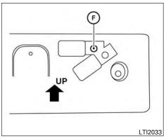
Mark the center of the hole  $\bigcirc$  on both sides with a felt-tip pen. Remove the bracket from the bumper, and then open 0.79 in (20 mm) diameter holes on the bumper using the marks  $\bigcirc$  as a center.
