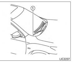
Be sure you do not put anything on top of the autolight sensor located in the top side (1) of the instrument panel. The autolight sensor controls the autolight; if it is covered, the autolight sensor reacts as if it is dark out and the headlights will illuminate. If this occurs while parked with the engine off and the ignition switch placed in the ON position, your vehicle's battery could become discharged.
