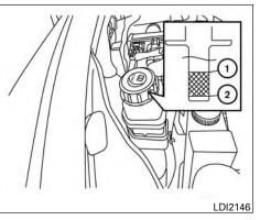
Check the fluid level in the reservoir.
