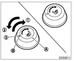
The front seats are warmed by built-in heaters. The switches are located on the center console and can be operated independently of each other.
