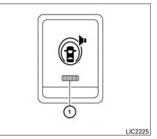
The Warning Systems switch is used to turn on and off the warning systems (Forward Collision Warning (FCW), Lane Departure Warning (LDW) and Blind Spot Warning (BSW) systems) that are activated using the settings menu on the vehicle information display.
