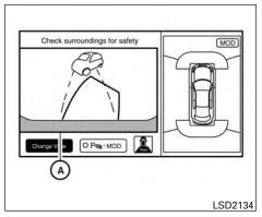
The system does not operate if the object is very close to the bumper.
