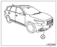
The IBA system uses a distance sensor (A) located behind the front bumper to measure the distance to the vehicle ahead. When the system judges that your vehicle is getting close to the vehicle ahead in the traveling lane, the vehicle ahead detection indicator light on the information display blinks and a warning chime sounds.
