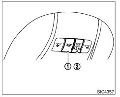
When the ON switch ① is pressed, the footwell lights, step lights, map lights and rear personal lights will automatically turn on and stay on for a period of time when:
