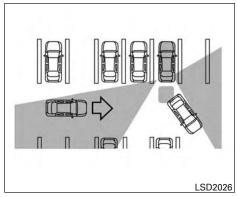
The BCI system uses radar sensors ① installed on both sides near the rear bumper to detect an approaching vehicle and sonar sensors to detect objects in the rear.
