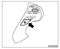
The BSI system turns on when the dynamic driver assistance switch on the steering wheel is pushed when the "Blind Spot Intervention" is enabled in the settings menu on the vehicle information display. The BSI ON indicator light on the instrument panel illuminates when the BSI system is turned on.
