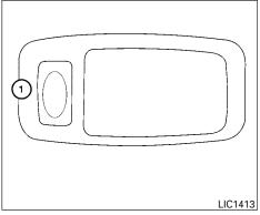
To turn on the personal lights, press and release the switch (1).
