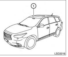
The Lane Departure Warning (LDW) system/ Lane Departure Prevention (LDP) system will operate when the vehicle is driven at speeds of approximately 45 MPH (70 km/h) and above, and only when the lane markings are clearly visible on the road.
