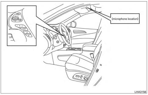
Your INFINITI is equipped with the Bluetooth® Hands-Free Phone System. If you have a compatible Bluetooth® enabled cellular phone, you can set up the wireless connection between your cellular phone and the in-vehicle phone module. With Bluetooth® wireless technology, you can make or receive a hands-free telephone call with your cellular phone in the vehicle.
