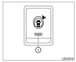
When the warning systems switch is turned off, the indicator ① on the switch is off. The indicator will also be off if the BSW, the Lane Departure Warning (LDW) and the Forward Collision Warning (FCW) systems are deactivated.
