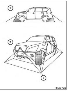
There are some areas where the system will not show objects and the system does not warn of moving objects. When in the front or rear view display, an object below the bumper or on the ground may not be viewed ①. When in the bird's-eye view, a tall object near the seam (3) of the camera viewing areas will not appear in the monitor (2).
