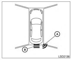
When the corner of the vehicle moves closer to an object, the corner sonar indicators ( $\hat{A}$ ) appears. When the center of the vehicle moves close to an object, the center sonar indicator ( $\hat{B}$ ) appears.
