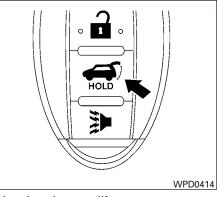
Releasing the rear liftgate
