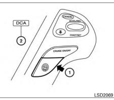
LDP system will also turn on or off simultaneously. The DCA system can be individually set to on or off on the display. If the system is set to off, the system will not turn on even if the dynamic driver assistance switch is pushed to on. To set the system to on or off on the display, refer to "Setting DCA system to ON/OFF" in this section.
