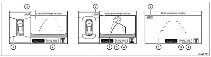
When the MOD system detects a moving object near the vehicle, the yellow frame will be displayed on the view where the objects are detected and a chime will sound once. While the MOD system continues to detect moving objects, the yellow frame continues to be displayed.
