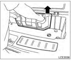
2. Remove the jack and tool kit cover by lifting up using the handles.
