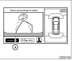
If the radar detects an approaching vehicle from the side, the system chimes a sound (single beep), the Blind Spot Warning indicator light on the side the approaching vehicle flashes and a yellow rectangular frame appears in display (A).
