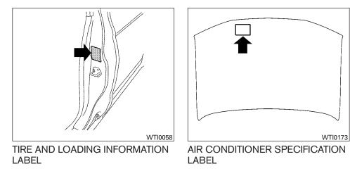
The cold tire pressure is shown on the Tire and Loading Information label. The label is located as shown.
