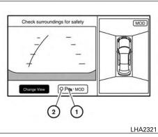
When the switch ① is selected, the indicator ② will turn off and the sonar will be turned off temporarily. The MOD system will also be turned off at the same time. When the switch is selected again, the indicator will turn on and the sonar will turn back on.
