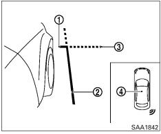
The corner sonar indicator (4) can be turned off. For additional information, refer to "Around View® Monitor" in this section.
