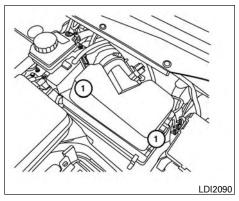
Clean and replace the air cleaner filter according to the maintenance log shown in the "INFINITI Service and Maintenance Guide." When replacing the filter, wipe the inside of the air cleaner filter housing and the cover with a damp cloth.
