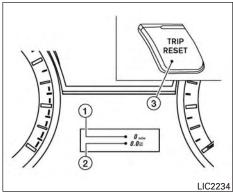
Odometer/Twin trip odometer
