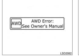
If the AWD error warning message is displayed, there may be a malfunction in the Intelligent AWD system. Reduce vehicle speed and have your vehicle checked by an INFINITI retailer as soon as possible.
