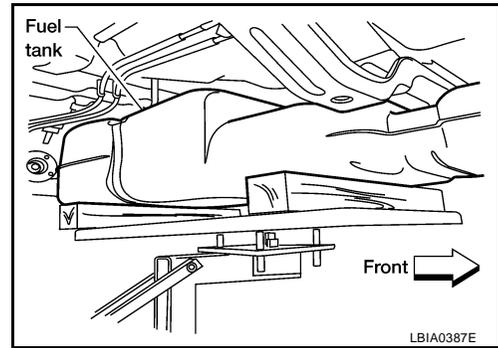
20. Disconnect the EVAP hose from the molded clip in the top of the fuel tank while lowering the fuel tank.
