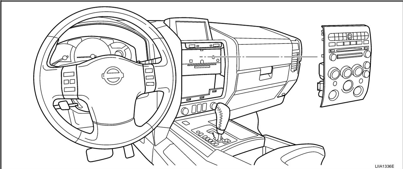
1. Remove center console. Refer to [IP-10, "INSTRUMENT PANEL ASSEMBLY"](#) .
