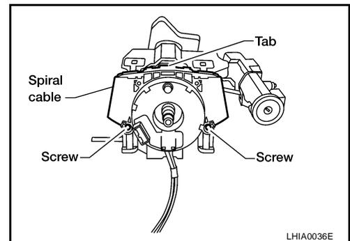
9. Remove the spiral cable connectors.
