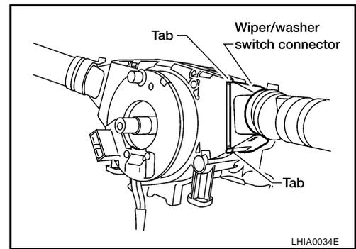
7. While pressing tabs, pull lighting and turn signal switch toward driver door and disconnect from base.
