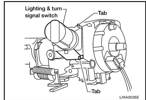
8. Remove the screws, release the clip, and remove the spiral cable.
