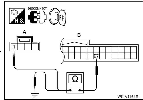
3. Check continuity between combination meter harness connector M24 terminal 27 (O/B) and ground.
