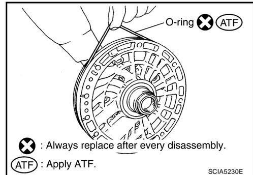
2. Install O-ring to oil pump housing.
