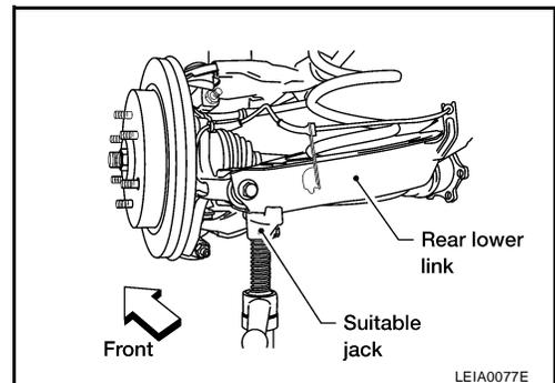
5. Loosen the rear lower link adjusting bolt and nut connected to the rear suspension member, using power tool.
