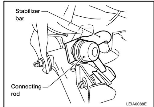
2. Remove the stabilizer bar clamps using power tool, and remove the stabilizer bar bushings.
