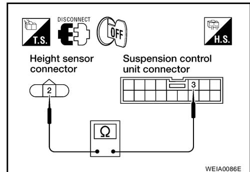
3. Check resistance between height sensor connector C8 terminal 2 (W) and ground.
