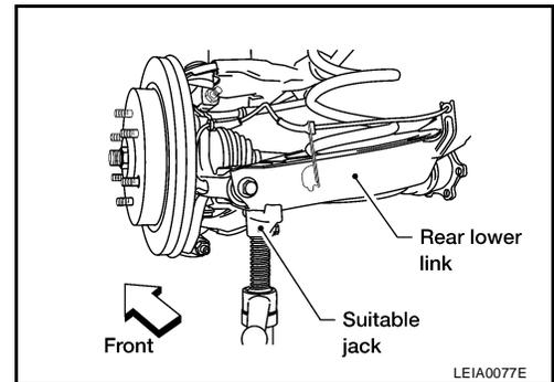
14. Remove both of the rear lower link outer bolts and lower the jack to remove the rear coil springs.
