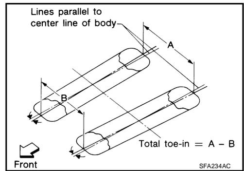
7. If the toe-in is outside the specified value, adjust the toe-in using the adjusting bolt in the rear lower link.
