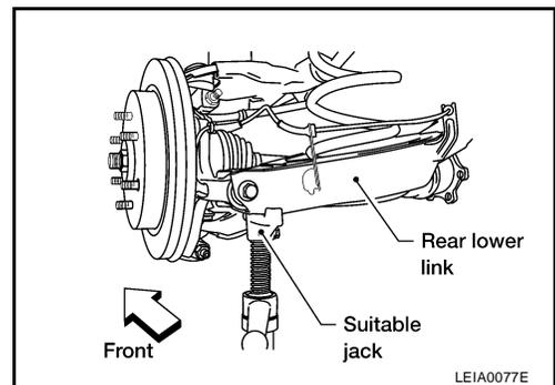
7. Slowly lower the suitable jack to release the coil spring tension. Then remove the upper rubber seat, coil spring, and lower rubber seat from the rear lower link.
