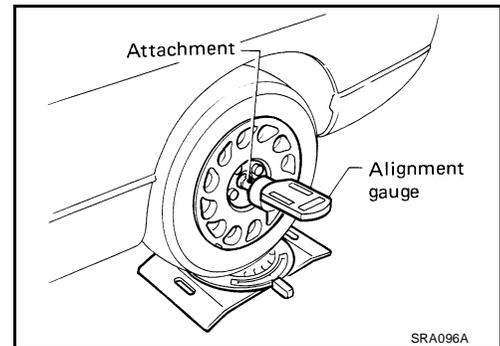
2. If outside of the specified value, adjust the camber using the adjusting bolt in the front lower link.
