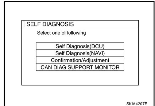
5. When "Confirmation/Adjustment" is selected on the initial self-diagnosis screen, the operation will enter the CONFIRMATION/ADJUSTMENT mode. In this mode, check and adjustment of each item will become possible.
