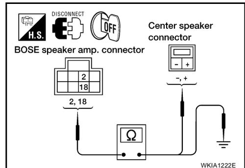
3. Check continuity between BOSE speaker amp. harness connector M112 terminals and ground.
