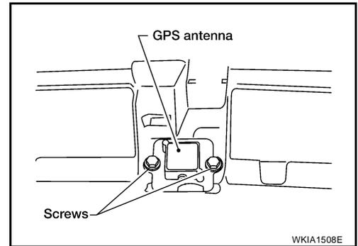
4. Disconnect GPS antenna connector and remove GPS antenna and feeder assembly out the top.
