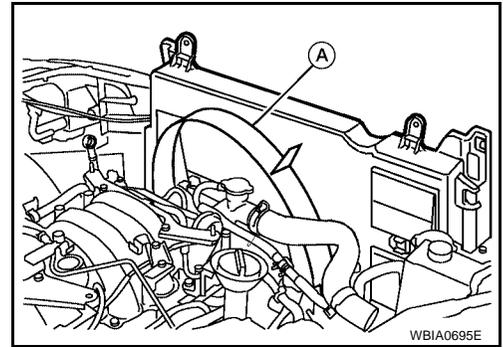
8. Remove the A/C condenser bolts and brackets.
