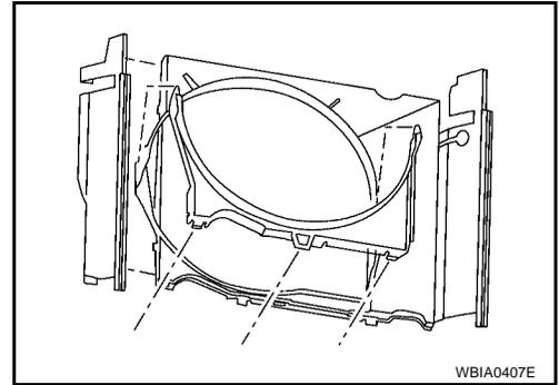
7. Remove the radiator shroud upper bolts and remove the radiator shroud upper A.
