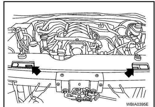
9. Remove A/T oil cooler bolts and oil cooler from radiator and position aside.
