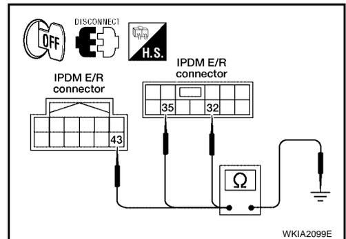
5. Check continuity between IPDM E/R harness connector terminal and ground.
