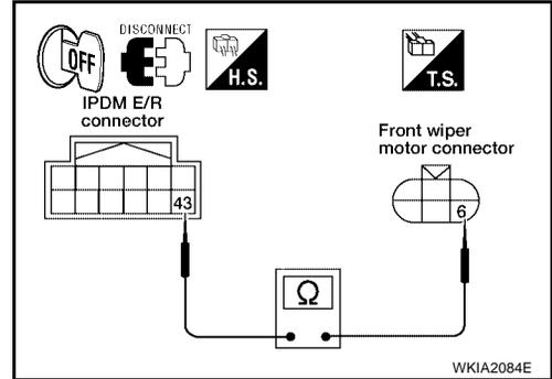
4. Check continuity between IPDM E/R harness connector terminal and ground.
