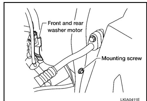
2. Remove front and rear washer motor connector.
