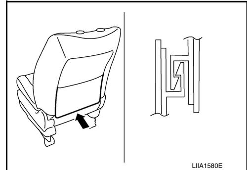
3. From inside of the seatback, squeeze the headrest holder tabs at the base of the stay pipe and pull up to remove.
