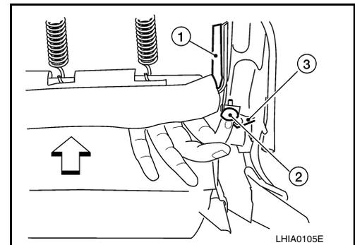
5. Partially lift seatback upright, then remove seat belt buckle (2) from between hinge cover (1) and seat cushion side facing (3).
