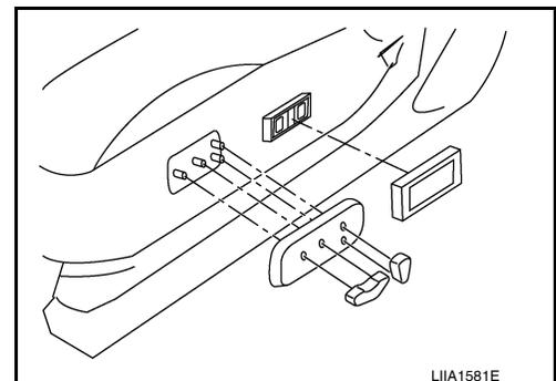
2. Remove the power seat and power lumbar switches.
