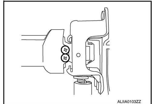
4. Starting at the right side, snap the cable and conduit into the power seat cross-beam retainers.
