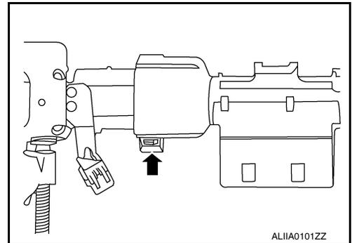
9. Remove the power motor cross-beam screws.
