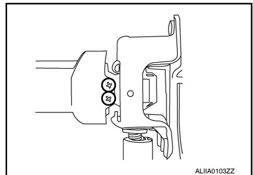
10. Remove the power motor cross-beam.
