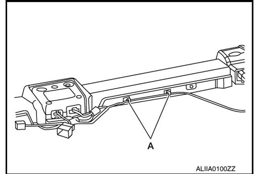
8. Release the power motor cross-beam clip (A) and open the hinged strap.
