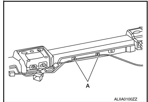
8. Install the seat control unit and connect the seat control unit harness connectors.
