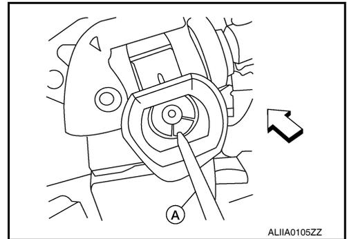
3. Install the power motor cross-beam right side screws
