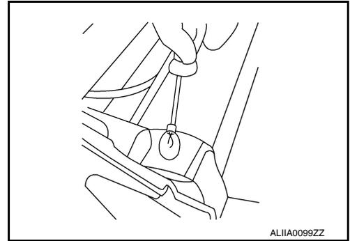
7. Install the seat harness to the power seat motor cover connectors.
