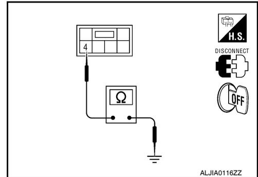
4. Check continuity between any third row power folding seat switch driver side harness connector B164 or B165 terminal 2, 3 and third row power folding seat control unit harness connector B401 terminals 4, 12.
