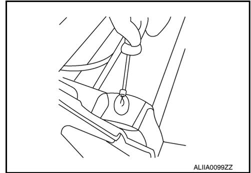
6. Disconnect the wiring harness from the power seat motor cover clips.
