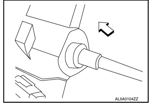
2. Install the cable into the RH seat motor.
