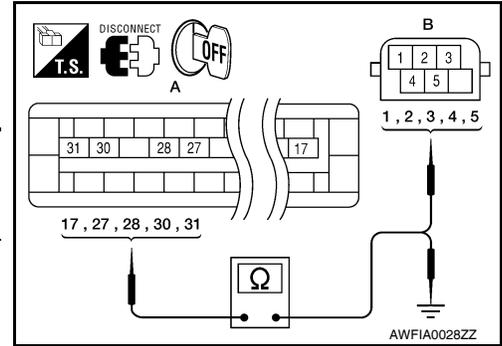
2. Measure the continuity between ABS actuator and electric unit (control unit) harness connector E125 (A) and body ground.
