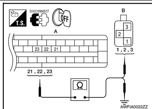
2. Measure the continuity between the ABS actuator and electric unit (control unit) harness connector E125 (A) and body ground.
