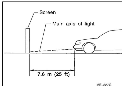
3. Adjust front fog lamps using adjusting screw so that the top edge of the high intensity zone is 200 mm (7.9 in) below the height of the fog lamp centers as shown.
