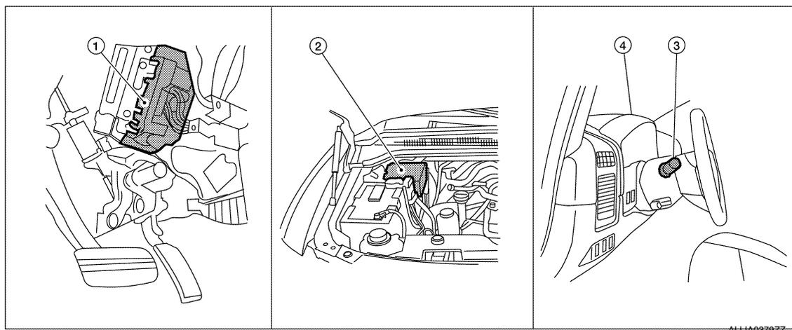
1. BCM M18, M20 (view with instrument panel removed)
