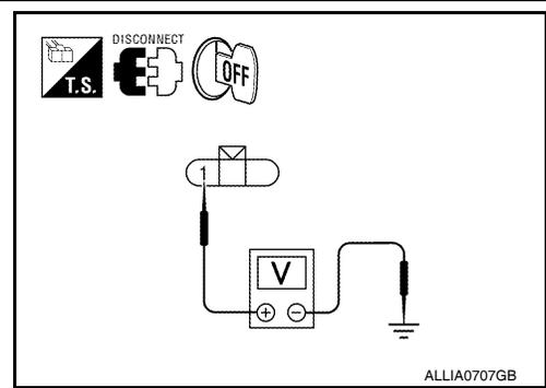
7. With the parking lamps ON, check voltage between the license plate lamp connector and ground.
