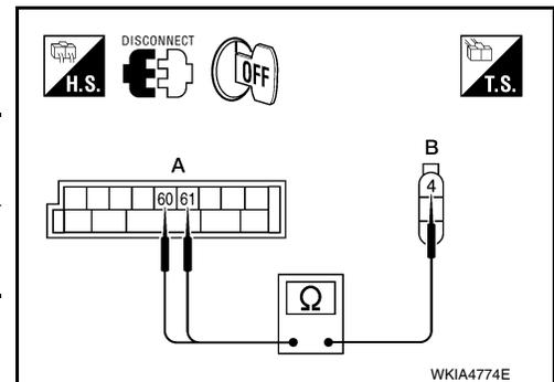
5. Check continuity between the BCM harness connector M20 and the door mirror connectors.
