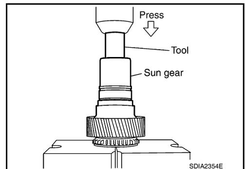
31. Remove the metal bushing from the sun gear using Tools.
