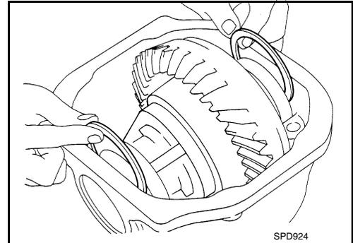
3. Align the matching mark on the side bearing cap with the matching mark on the gear carrier.
