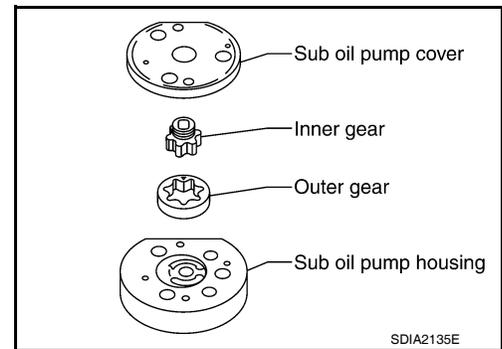
6. Align the dowel pin hole and bolt hole of the sub oil pump assembly with the center case. Install the sub oil pump cover. Then tighten to the specified torque. Refer to [DLN-140, "Disassembly and Assembly"](#).
