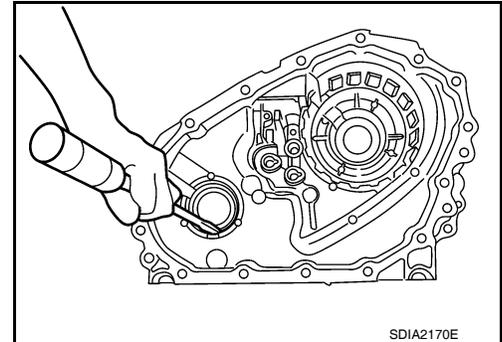
24. Remove the snap ring from the front case.
