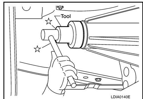
2. Apply petroleum jelly to the circumference of the new dust cover. Position the new dust cover using the identification mark as shown.
