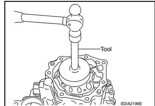
32. Install the mainshaft assembly using a press.
