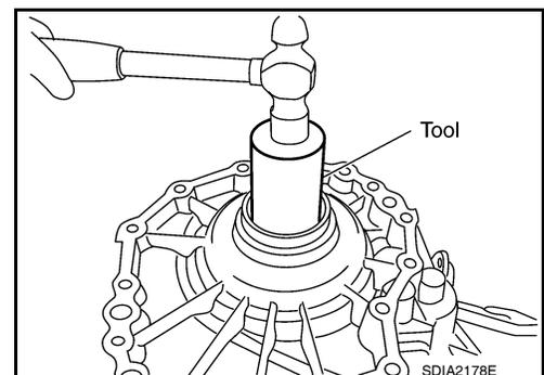
26. Remove the snap ring from the planetary carrier assembly using suitable tool.
