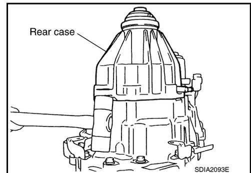
3. Remove the dust cover using suitable tool.
