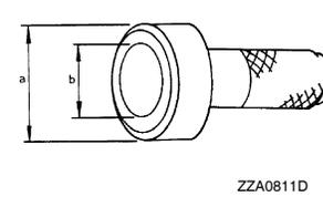
ZZA0811D    | <ul style="list-style-type: none"> <li>• Installing rear oil seal</li> <li>• Installing mainshaft front bearing and oil seal</li> </ul> a: 77 mm (3.03 in) dia.<br>b: 55.5 mm (2.185 in) dia. |
