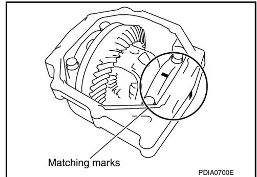
13. Tighten each side bearing adjuster alternately turning drive gear.
