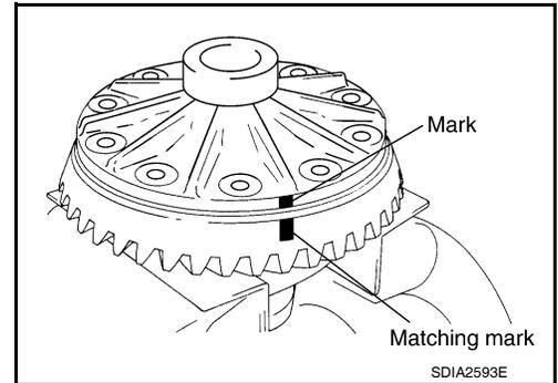
8. Install and tighten the new drive gear bolts to the specified torque. Refer to "[DLN-214, "Disassembly and Assembly"](#)".
