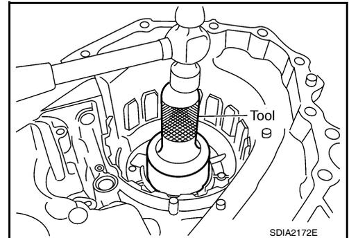
8. Install the new snap ring into the front case.
