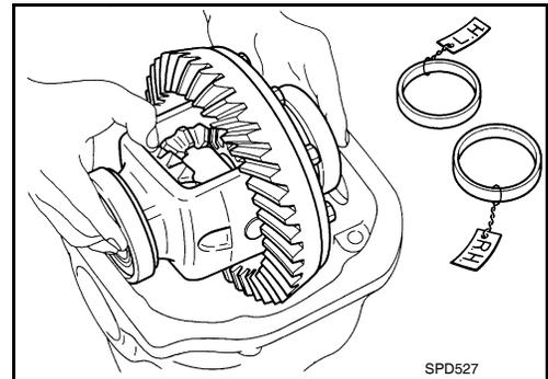
2. Insert the left and right original side bearing adjusting washers in place between side bearings and gear carrier.
