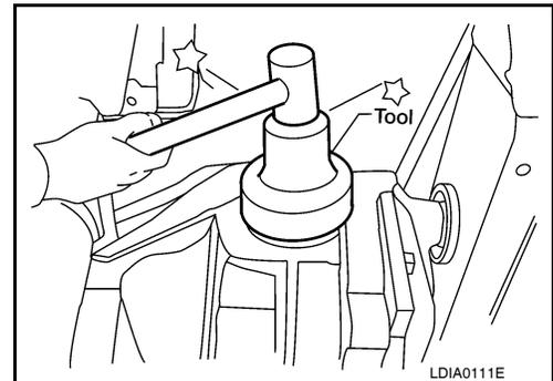
2. Install the side flange using Tool.
