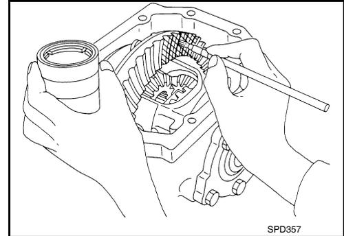
2. Rotate the drive gear back and forth several times. Then check for correct drive pinion to drive gear tooth contact as shown.
