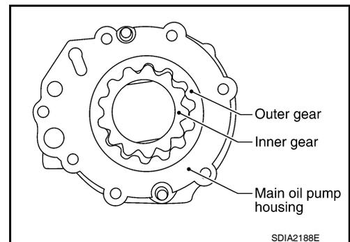
39. Install the main oil pump cover to the center case, and tighten to the specified torque. Refer to [DLN-140](#), "[Disassembly and Assembly](#)".
