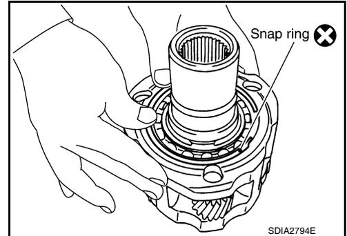
7. Set the input bearing into the front case and install using suitable tool.
