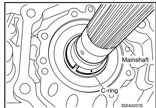
34. Set the washer holder on the mainshaft, and secure it with a new snap ring.
