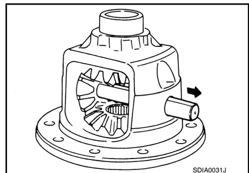
17. Turn the pinion mate gear, then remove the pinion mate gear, pinion mate thrust washer, side gear and side gear thrust washer from the differential case.
