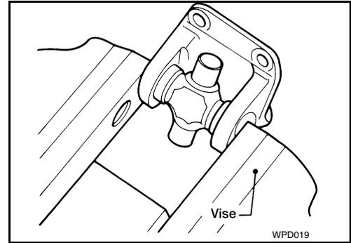
2. Select new snap rings that will provide the specified play in an axial direction of the journal, and install them. Refer to [DLN-188](#), "[Snap Ring](#)".
