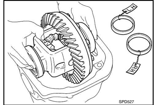
12. Install the side bearing caps with the matching marks aligned.
