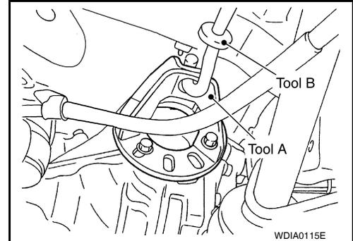
3. Remove the side oil seal using suitable tool.
