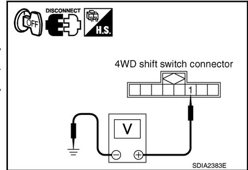
4. Turn ignition switch ON. (Do not start engine.)
