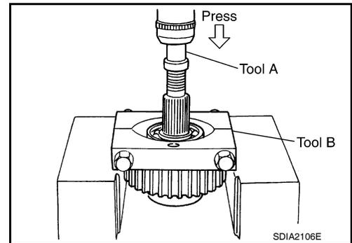
5. Remove the front drive shaft rear bearing using Tools.
