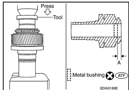
4. Apply ATF to the new needle bearing and install it to the sun gear assembly using Tool.
