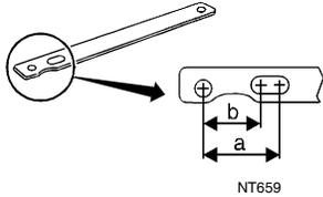
NT659     | <ul style="list-style-type: none"> <li>• Removing self-lock nut</li> <li>• Installing self-lock nut</li> </ul> a: 85 mm (3.35 in)<br>b: 65 mm (2.56 in)                                       |
