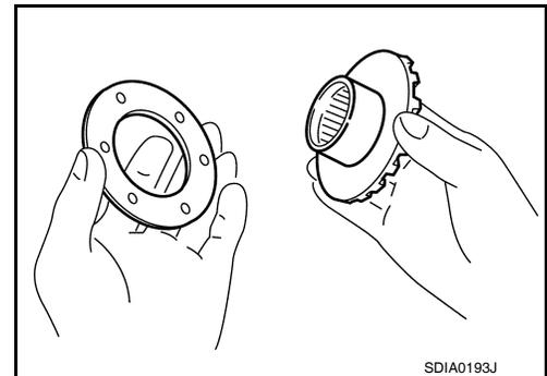
2. Install the side gears and side gear thrust washers into the differential case.
