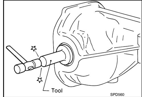
2. Install the side flange using Tool.
