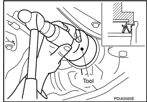
2. Install the companion flange to the drive pinion while aligning the matching marks.
