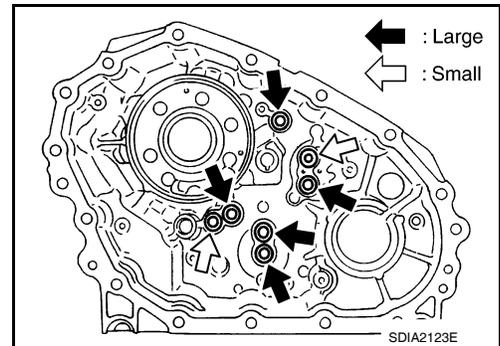
11. Install the control valve assembly to the center case, and tighten to the specified torque. Refer to [DLN-140, "Disassembly and Assembly"](#).
