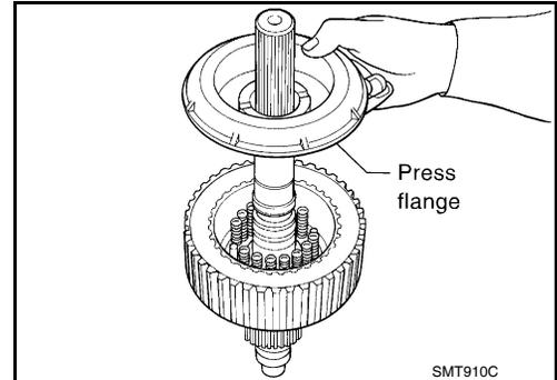
19. Remove the return spring assembly from the clutch hub.
