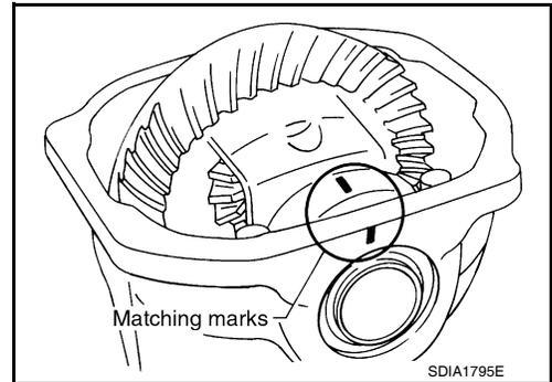
6. To determine side bearing preload torque, measure the pulling force of the differential assembly at the drive gear bolt using Tool.
