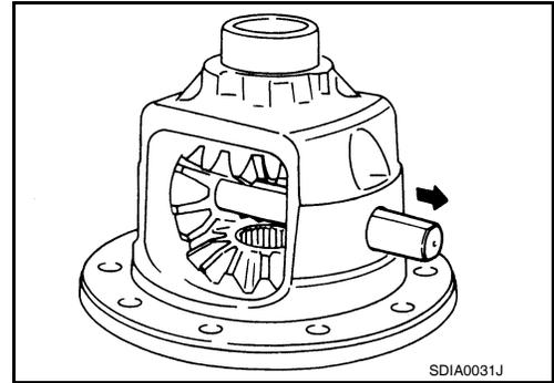
14. Turn the pinion mate gear, then remove the pinion mate gear, pinion mate thrust washer, side gear and side gear thrust washer from the differential case.
