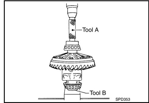
11. Install the differential case assembly with the side bearing outer races into the gear carrier.
