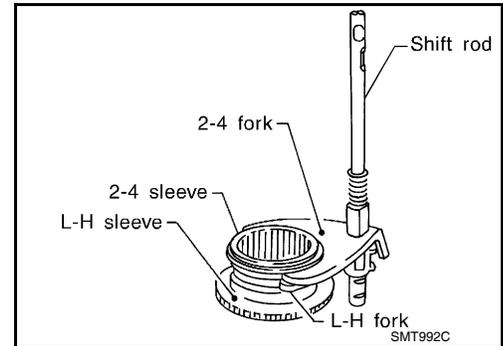
17. While aligning the L-H sleeve with the planetary carrier, install the shift rod assembly (A) to the front case.
