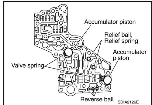
e. Install the lower body and separator plate to the upper body.
