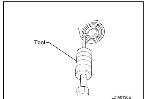
6. Remove the carrier cover bolts and separate the carrier cover from the gear carrier using Tool.
