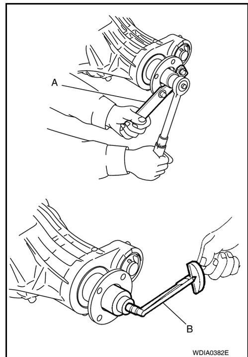
11. Check companion flange runout. Refer to [DLN-231, "Inspection and Adjustment"](#).
