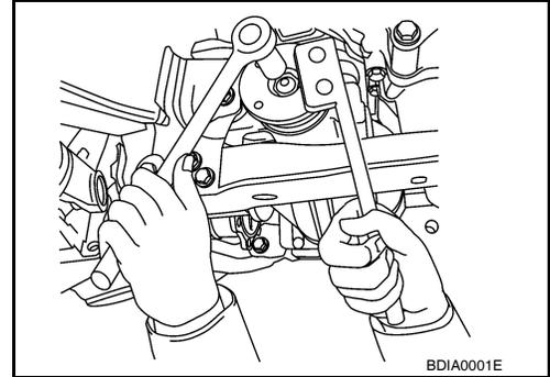
6. Remove companion flange using suitable tool.
