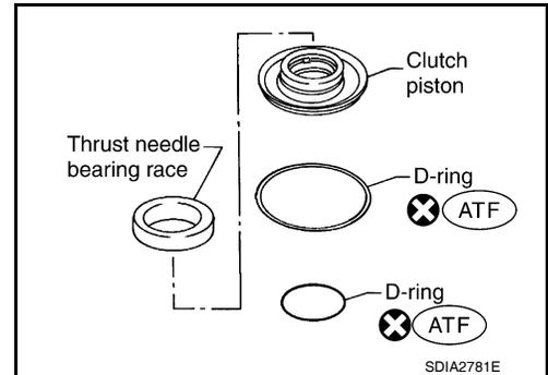
17. Install the thrust needle bearing race to the clutch piston.
