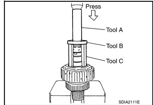
28. Install the new snap ring to the mainshaft using suitable tool.
