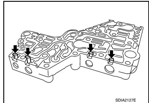
d. Install the reverse balls, relief balls and relief springs, accumulator pistons and valve springs to the upper body.
