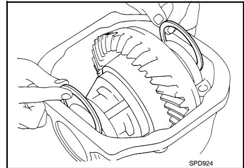
14. Install the side bearing caps with the matching marks aligned and tighten the side bearing cap bolts to the specified torque. Refer to "COMPONENTS".
