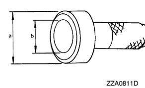
ZZA0811D        | <ul style="list-style-type: none"> <li>• Installing front oil seal</li> </ul> a: 80 mm (3.15 in) dia.<br>b: 60 mm (2.36 in) dia.                                                              |
