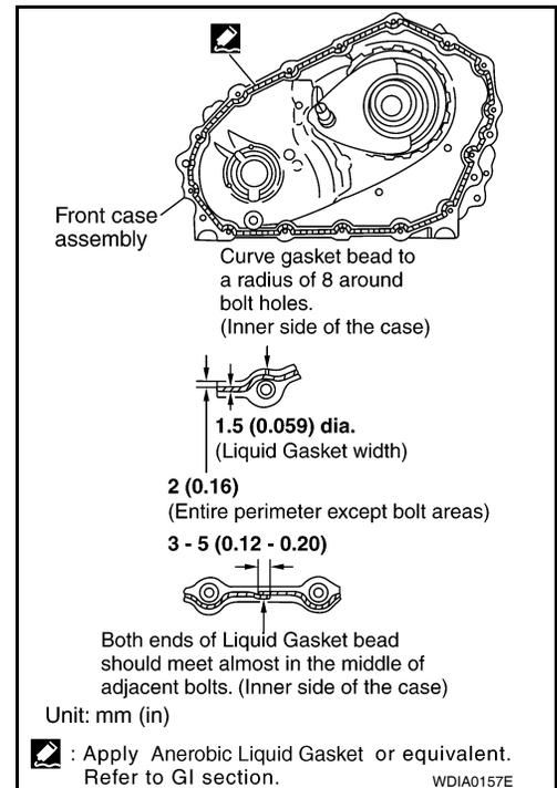
19. Install the center case assembly to the front case assembly.
