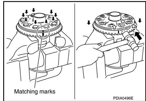
12. Remove the lock pin of the pinion mate shaft from the drive gear side using suitable tool.
