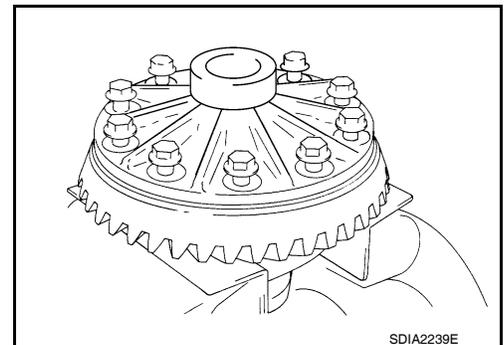
9. Press the new side bearing inner races to the differential case using Tools (A) and (B).
