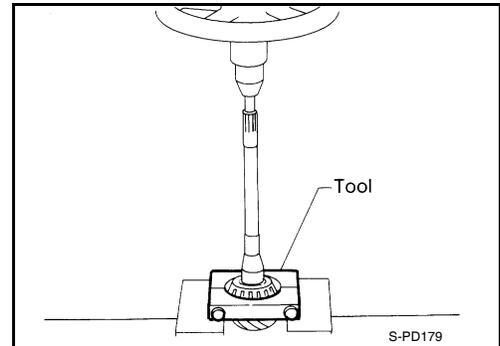
9. Remove the drive pinion front and rear bearing outer races by tapping them uniformly using suitable tool.
