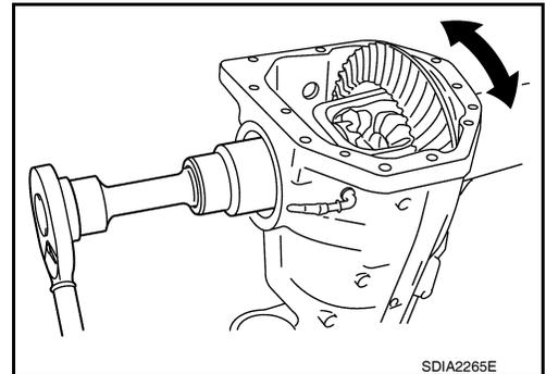
14. Check and adjust tooth contact, backlash, drive gear runout and total preload torque. Refer to [DLN-231, "Inspection and Adjustment"](#).
