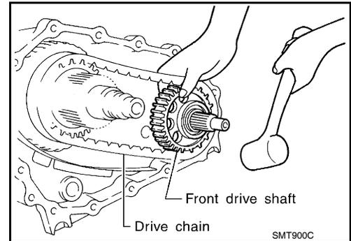
4. Remove the front drive shaft front bearing using Tools.
