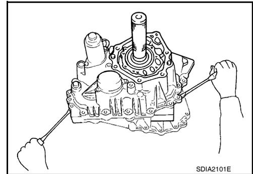
14. Remove the shift rod components together with the 2-4 sleeve and L-H sleeve.
