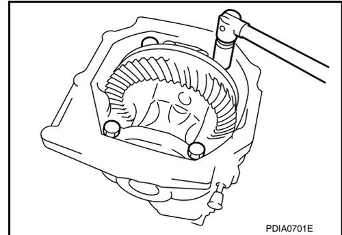
9. Remove the side bearing adjuster.
