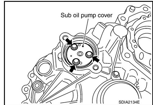
39. Thread two bolts (M4 x 0.8) into the holes of sub oil pump cover as shown, and pull out to remove the sub oil pump assembly.
