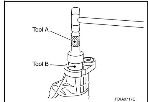
9. Install the companion flange to the drive pinion while aligning the matching marks. Tap the companion flange until fully seated using suitable tool.
