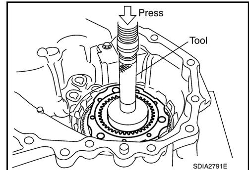
12. Install the new snap ring to the sun gear.
