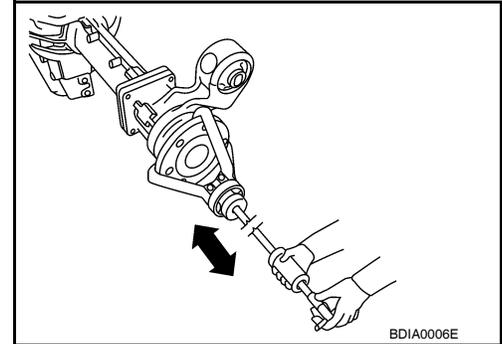
3. Place a small hole in the side oil seal case using suitable tool.
