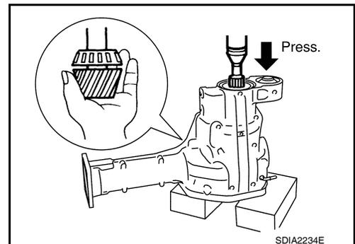
6. Remove the drive pinion rear bearing inner race and drive pinion height adjusting washer using Tool.
