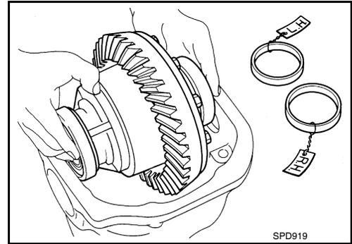
8. Remove the side bearing inner races using Tools.
