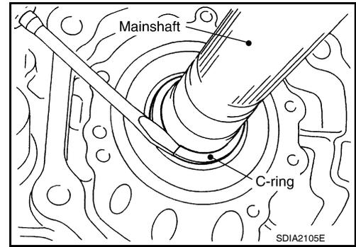
13. Set the center case on the press stand. Remove the mainshaft from the center case.
