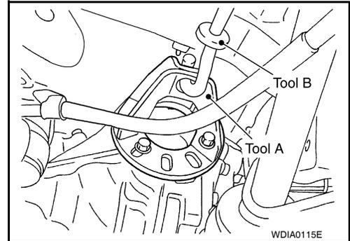
3. Remove the side oil seal using suitable tool.
