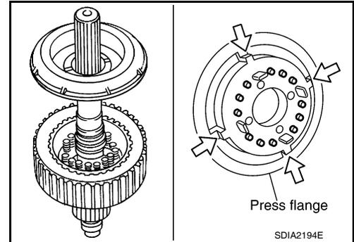
27. Press the press flange to install the new snap ring into snap ring groove on mainshaft using Tools.
