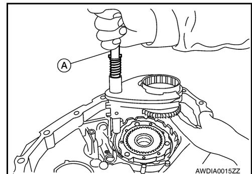
16. Remove the 2-4 sleeve and L-H sleeve from the 2-4 fork and L-H fork respectively.
