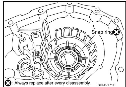
25. Remove the input bearing from the front case using Tool.
