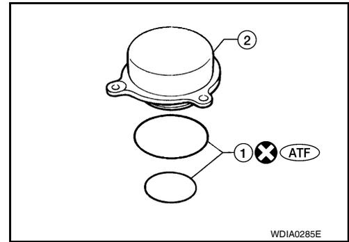
4. Install the oil filter to the transfer assembly. Tighten the bolts to the specified torque. Refer to [DLN-125, "Removal and Installation"](#).
