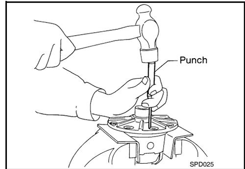
16. Remove the pinion mate shaft.
