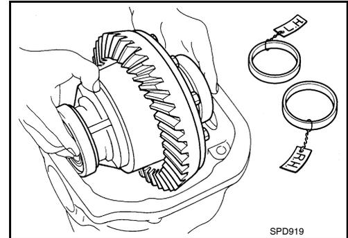
13. Insert the selected left and right side bearing adjusting washers in place between the side bearings and gear carrier.
