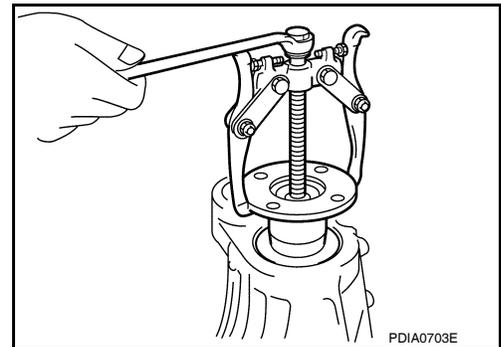
5. Press the drive pinion assembly (with rear inner bearing race and collapsible spacer) out of the gear carrier.
