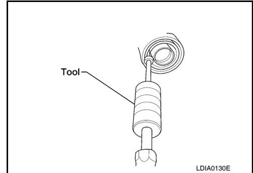
9. Remove the drive pinion front bearing inner race.
