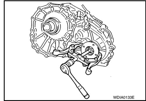
11. Remove the center case bolts, harness bracket and air breather.
