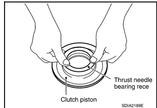
18. Install the clutch piston to the center case as shown.
