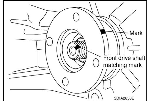
3. Install the new self-lock nut. Tighten to the specified torque using Tool. Refer to [DLN-140, "Disassembly and Assembly"](#).
