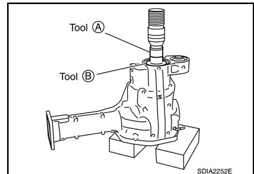
3. Select drive pinion height adjusting washer. Refer to [DLN-231, "Inspection and Adjustment"](#).
