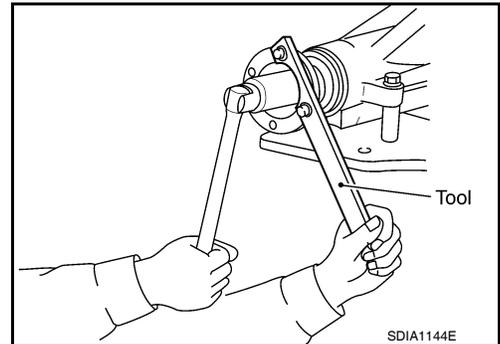
4. Remove the companion flange using suitable tool.
