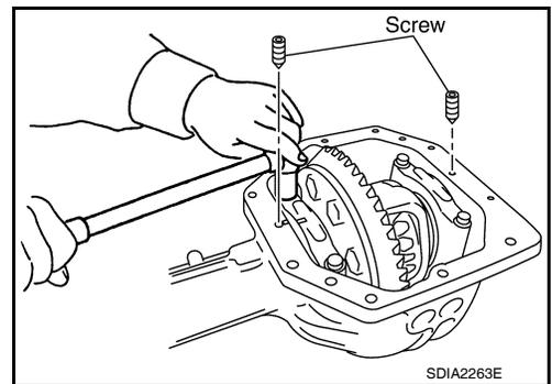
15. Apply multi-purpose grease to the lips of the new side oil seal. Then drive the new side oil seal in evenly to the gear carrier using suitable tool.
