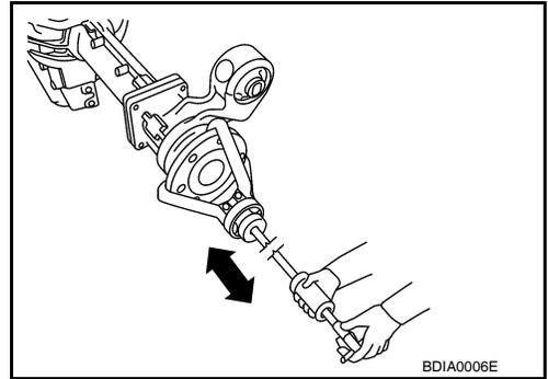
3. Remove the extension tube and O-ring from the gear carrier.
