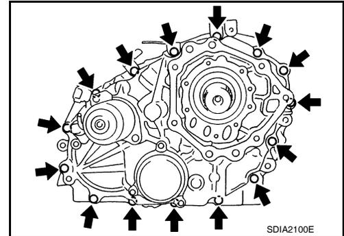
13. Separate the center case from the front case. Then remove the center case from the front case by prying it up using suitable tool.
