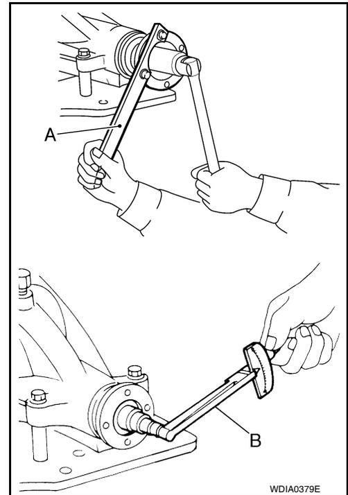
11. Check companion flange runout. Refer to "Companion Flange Runout".
