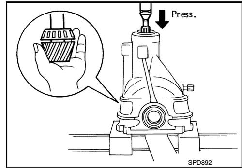
8. Remove the drive pinion rear bearing inner race and drive pinion height adjusting washer using Tool.
