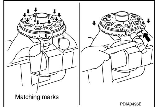
15. Remove the lock pin of the pinion mate shaft from the drive gear side using suitable tool.
