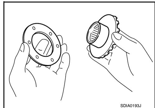
2. Install the side gears and side gear thrust washers into the differential case.
