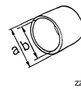
ZZA1003D        | <ul style="list-style-type: none"> <li>• Installing dust cover</li> </ul> a: 89 mm (3.50 in) dia.<br>b: 80.7 mm (3.17 in) dia.                                                                |
