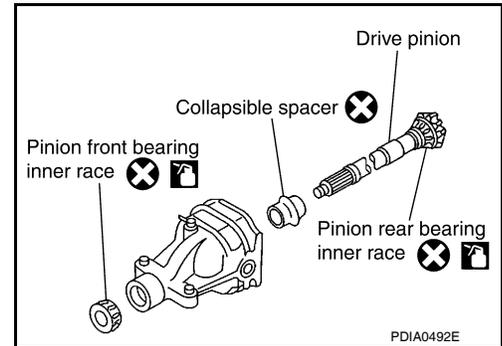
7. Press the drive pinion front bearing inner race to the drive pinion as far as drive pinion lock nut can be tightened using suitable spacer.
