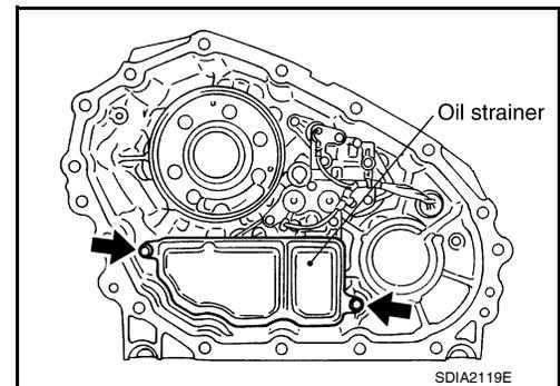
31. Remove the two O-rings from the oil strainer.
