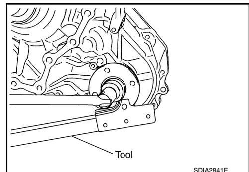
9. Put a matching mark on top of the front drive shaft thread in line with the mark on the companion flange.
