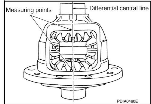
2. Using feeler gauges, measure the clearance between the side gear back and differential case at three different points, while rotating the side gear. Average the three readings to calculate the clearance. (Measure the clearance of the other side as well.)
