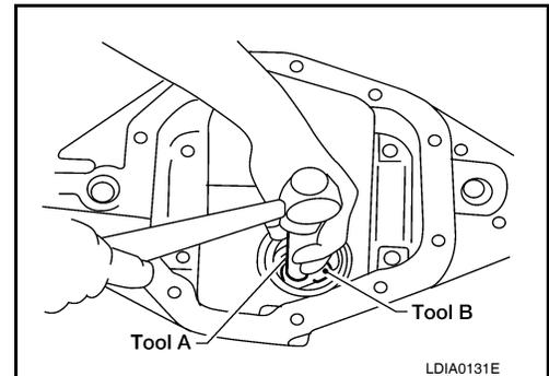
11. Remove the drive pinion rear bearing outer race using Tool as shown. Locate the driver on the back edge of the drive pinion rear bearing outer race, then drive the drive pinion rear bearing outer race out.
