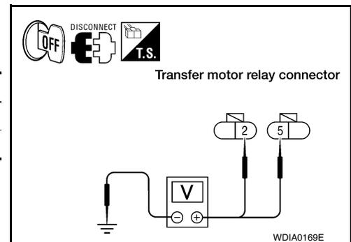
5. Turn ignition switch ON. (Do not start engine.)
