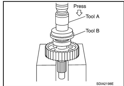
43. Install the front drive shaft to the front bearing using Tools.
