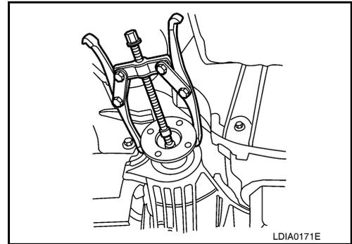
7. Place a small hole in the front oil seal case using suitable tool.
