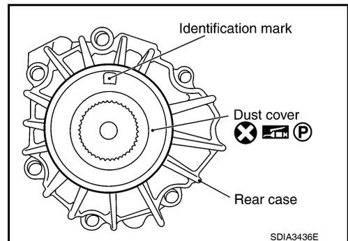
3. Install the new dust cover using Tool.
