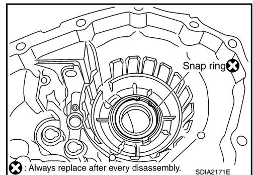
9. Install the internal gear with its groove facing the snap ring into the front case. Then secure it with the new snap ring.
