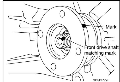
24. Install a new companion flange self-lock nut. Tighten to the specified torque using Tool. Refer to [DLN-140, "Disassembly and Assembly"](#).
