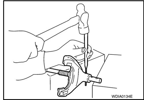
18. Remove the L-H fork, 2-4 fork, shift fork spring and fork guide from the shift rod.
