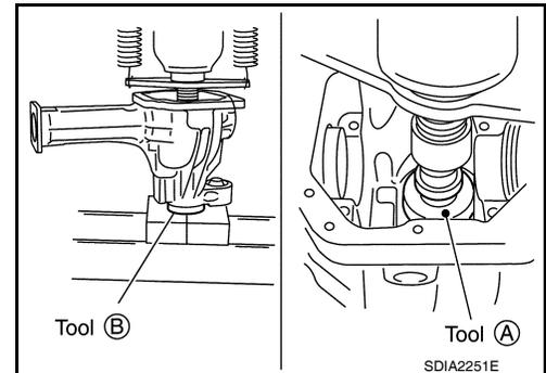
2. Install drive pinion front bearing outer race using Tools.
