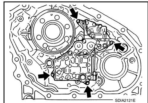
12. Install the connector assembly into the center case, and secure with a snap ring.
