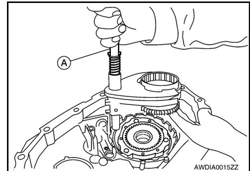
18. Apply liquid gasket to the entire center case mating surface of the front case assembly as shown.
