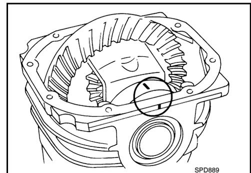
15. Check and adjust the drive gear runout, tooth contact, drive gear to drive pinion backlash, and total preload torque. Refer to "Drive Gear Runout", "Tooth Contact", "Backlash" and "Total Preload Torque". Recheck the above items.
