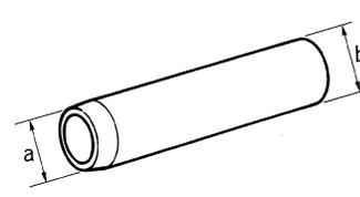
ZZA1091D | <ul style="list-style-type: none"> <li>• Installing side oil seal</li> </ul> a: 23 mm (0.91 in) dia.<br>b: 32 mm (1.26 in) dia.                                                               |
