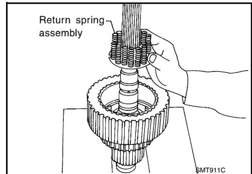
20. Remove each plate from the clutch drum.
