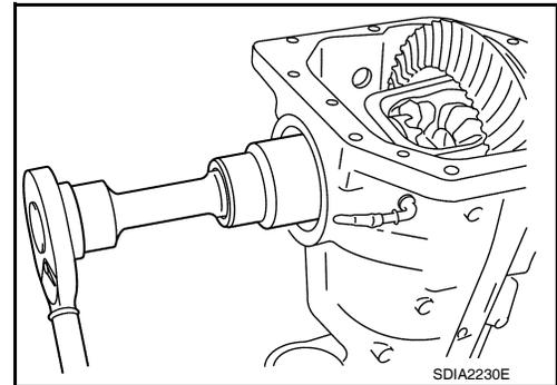
10. Lift the differential case assembly out of the gear carrier.
