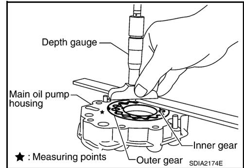
38. Install the main oil pump housing, outer gear and inner gear to the center case.
