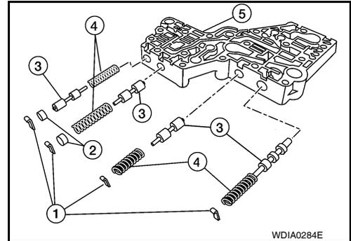
c. Install each control valve (3), springs (4), and plugs (2) to the upper body (5), and install retainer plates (1) to hold them in place.
