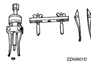
ZZA0601D     | <ul style="list-style-type: none"> <li>• Removing front oil seal</li> <li>• Removing rear oil seal</li> <li>• Removing metal bushing</li> </ul>                                               |
