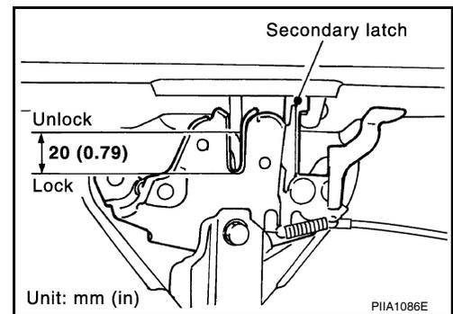
4. Check the hood lock lubrication condition. If necessary, apply "body grease" to the points shown in the figure.
