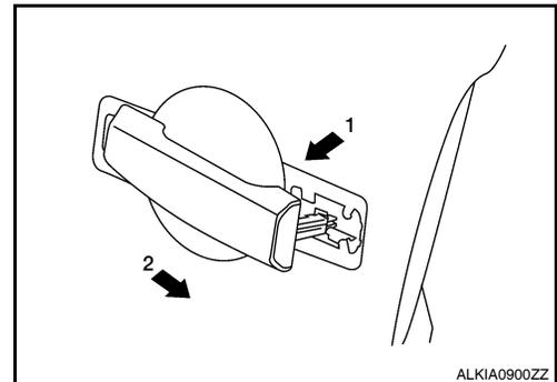
7. Remove the front gasket (1) and rear gasket (2).
