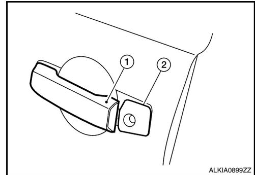
5. Separate the key cylinder rod from the door key cylinder assembly (if equipped).
