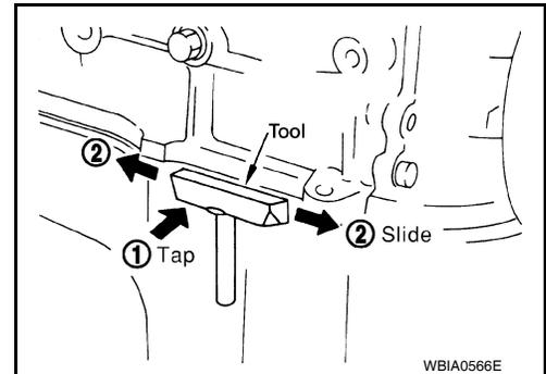
4. Remove the oil strainer from the oil pan (upper).
