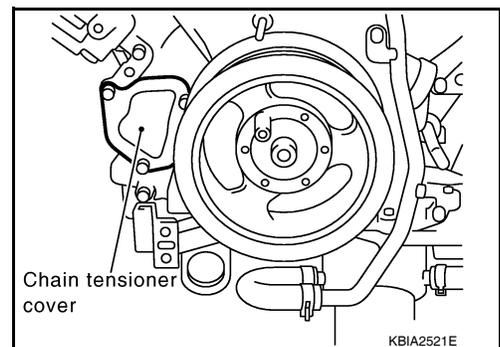
13. Remove the chain tensioner (RH) using the following steps.
