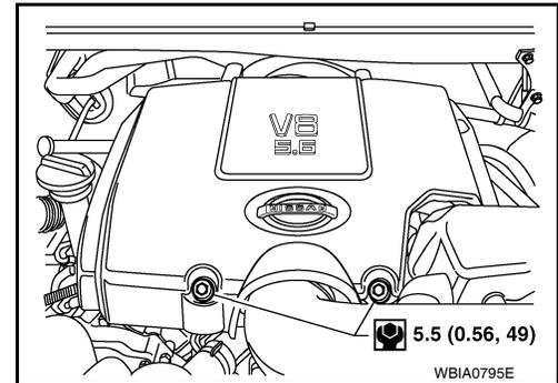
9. Remove the air duct and air cleaner case assembly. Refer to [EM-25, "Removal and Installation"](#).
