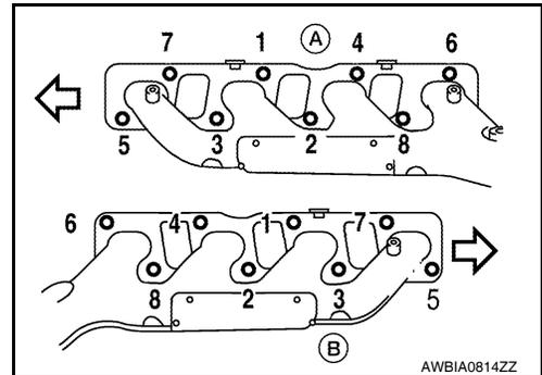
10. Remove the exhaust manifold (RH) (B) following the steps below.
