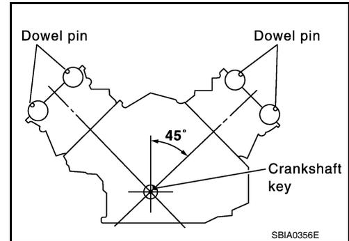
2. Install the camshaft sprockets.
