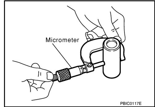
Connecting Rod Bushing Oil Clearance (Small End)
