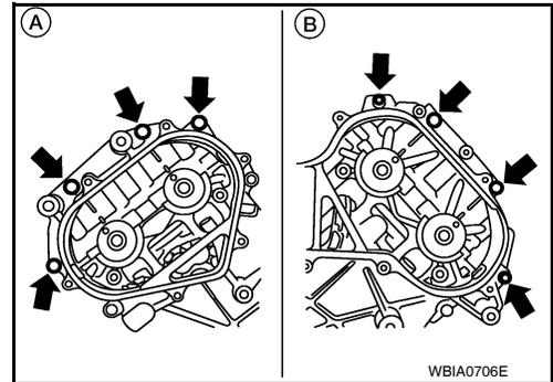
16. Remove RH (A) camshaft bracket bolts and LH (C) camshaft bracket bolts in the reverse of order shown to remove camshaft brackets.
