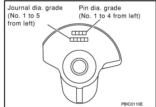
3. Read the symbol at the cross point of the selected row and column in the "Main Bearings Selection Table".
