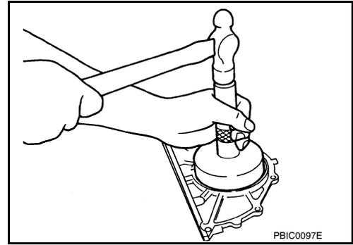
9. Install rear oil seal retainer.
