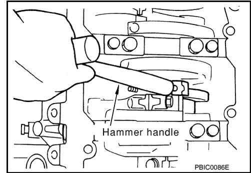
8. Remove connecting rod bearings.
