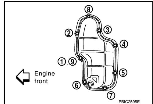
4. Install the oil pan drain plug.
