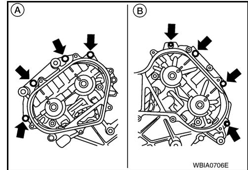
4. Tighten the camshaft bracket bolts as follows:
