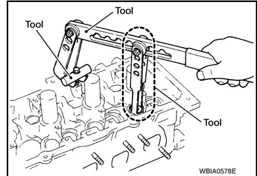
9. Install the valve lifters.
