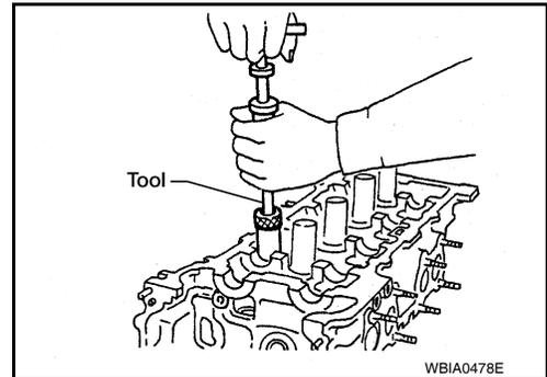
8. Replace the valve seat if necessary. Refer to [EM-72. "Inspection After Disassembly"](#).
