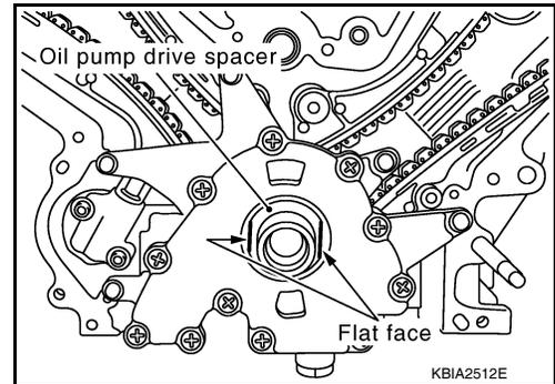
12. Remove the oil pump. Refer to [LU-14. "Removal and Installation"](#).
