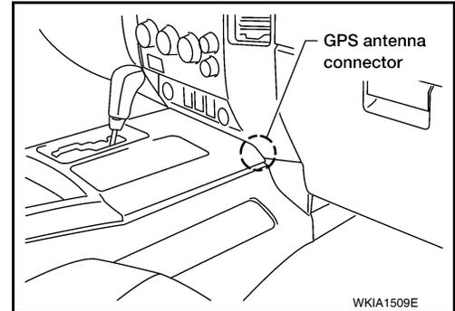
5. Remove the GPS antenna.
