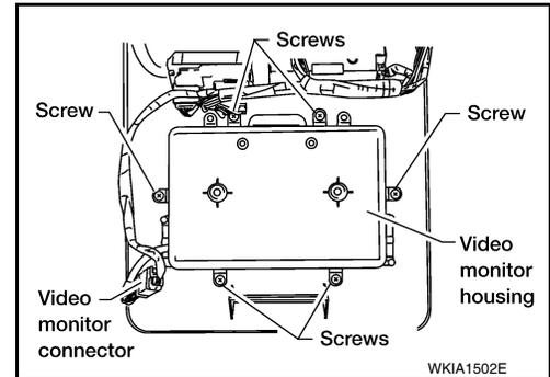
4. Remove the video monitor hinge screws.
