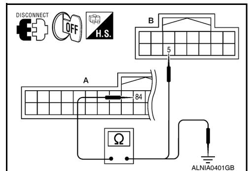
3. Check continuity between AV control unit harness connector M45 (A) terminal 84 and ground.
