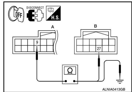
4. Check continuity between display unit harness connector M93 (A) terminal 9 and ground.
