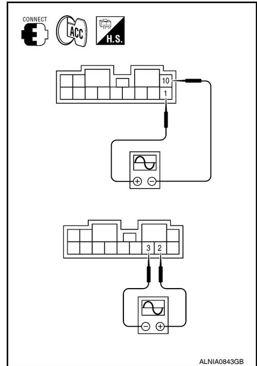
Are audio signal voltage readings as specified?
