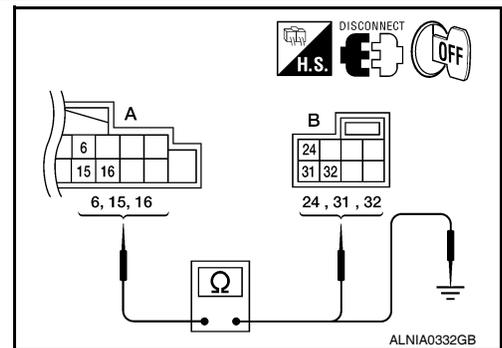
4. Check continuity between AV control unit connector M42 (A) and ground.
