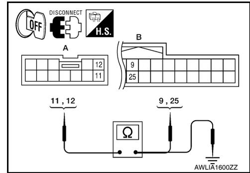
4. Check continuity between video monitor harness connector R202 (A) and ground.
