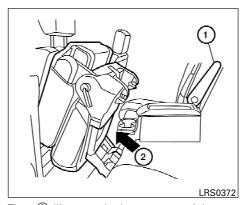
Then (2) lift up on the lower corner of the seat base and tip the 2nd row captain's chair forward. To exit the 3rd row bench seat, lift up on the same seatback latch and fold the seatback forward onto the seat base. Then lift up on the seat base and tip it forward.
