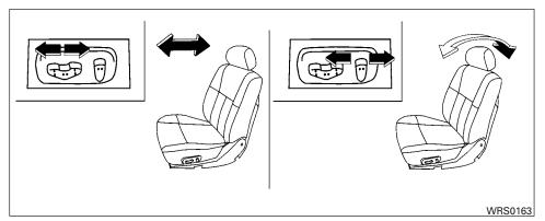
belt fit (see "Precautions on seat belt usage" later in this section). Also, the seatback can be reclined to allow occupants to rest when the vehicle is stopped and the shift selector is in P (Park).
