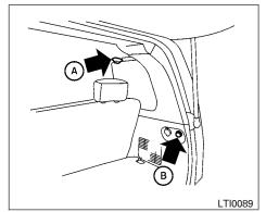
Cargo area ceiling tie-down hooks SECURING THE LOAD
