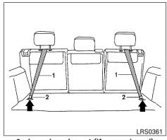
2nd row bench seat (if so equipped) **INSTALLING TOP TETHER STRAP** (2nd row captain's chairs or 2nd row bench seat [if so equipped])
