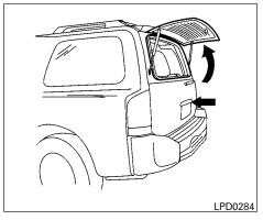
To open, press the button up on the smaller outside handle to release the glass hatch, then pull up on the glass hatch. To close, lower and push the glass hatch down securely.
