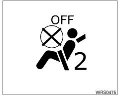
7. If the booster seat is installed in the front passenger seat, place the ignition switch in the ON position. The front passenger air bag status light \* may or may not illuminate, depending on the size of the child and the type of booster seat being used. See "Front passenger air bag and status light" later in this section.
