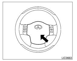
To sound the horn, push the center pad area of the steering wheel.
