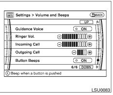
To access the settings, press the SETTING button, then highlight "Volume and Beeps" using the INFINITI controller and press the ENTER button.
