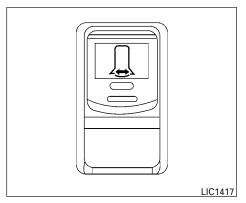
The power vent windows operate when the ignition switch is in the ON position, or for about 45 seconds after the ignition switch is placed in the OFF position. If the driver's or passenger's door is opened during this 45 second period, power to the vent windows is cancelled.
