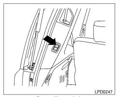
Rear pillar switch OPERATING THE POWER LIFT **GATE**
