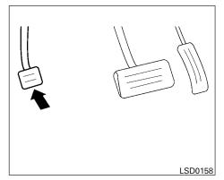
To engage: Firmly depress the parking brake.
