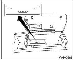
This vehicle is equipped with the INFINITI Mobile Entertainment System, which enables you to play a Digital Versatile Disc (DVD), providing the images and sounds both in the front and rear display screens.
