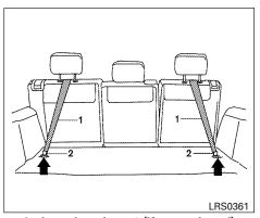
2nd row bench seat (if so equipped) REAR-FACING CHILD RESTRAINT INSTALLATION USING LATCH
