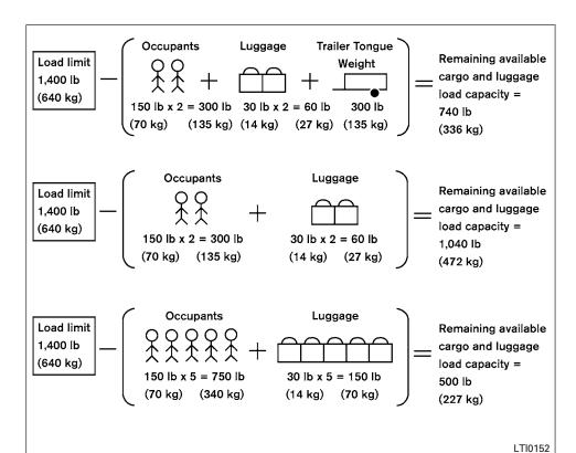
Steps for determining correct load limit
