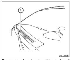
Be sure you do not put anything on top of the autolight sensor ① located in the top side of the instrument panel. The autolight sensor controls the autolight; if it is covered, the autolight sensor reacts as if it is dark out and the headlights will illuminate. If this occurs while parked with the engine off and the ignition switch placed in the ON position, your vehicle's battery could become discharged.
