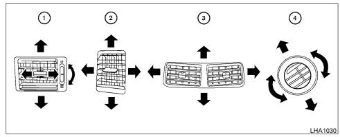
Adjust air flow direction for the driver's and passenger's side vents (1), center vents (2), and rear passengers' vents (3) and (4) by moving the vent slide and/or vent assemblies.
