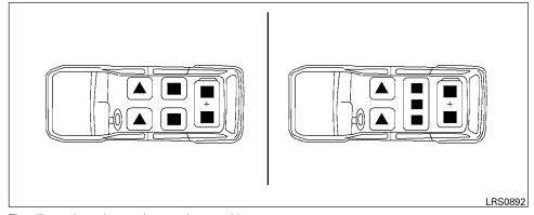
The illustration shows the seating positions equipped with adjustable headrests. All of the headrests are adjustable.
