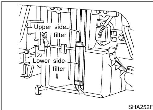
4. Take out the lower side ventilation air filter from cooling unit.
