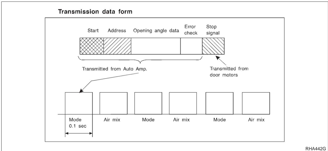
**Air Mix Door Control (Automatic Temperature Control)**
