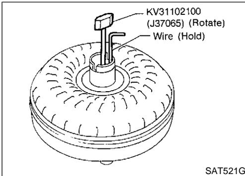
4. Check torque converter one-way clutch.
