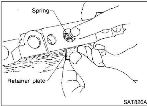
b. Remove retainer plates while holding spring.
