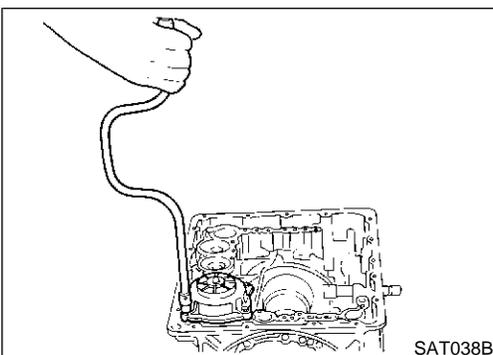
24. Remove band servo and accumulator components.
