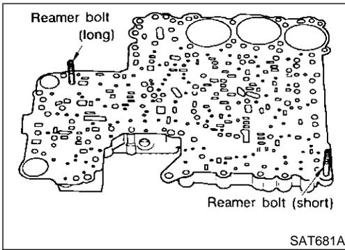
b. Install reamer bolts from bottom of upper body.
