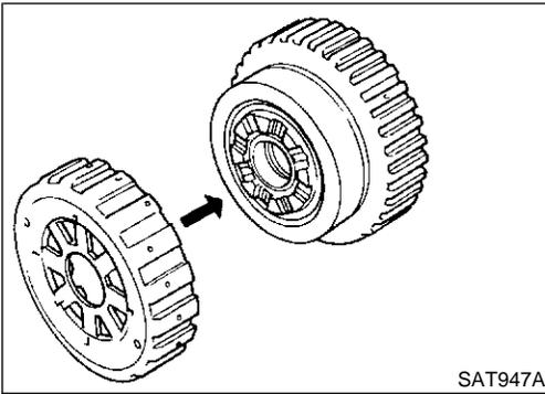
e. Install overrun clutch hub onto rear internal gear assembly.
