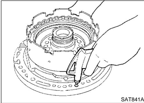
8. Check operation of reverse clutch. Refer to "DISASSEMBLY" of Reverse Clutch, AT-312.
