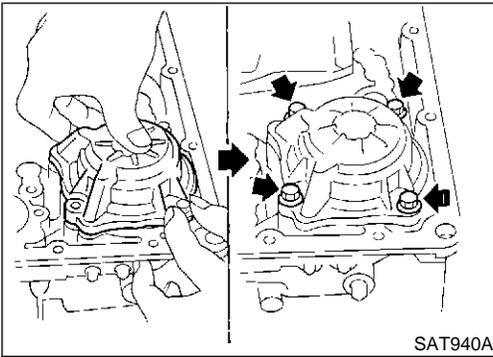
d. Install band servo retainer onto transmission case.
