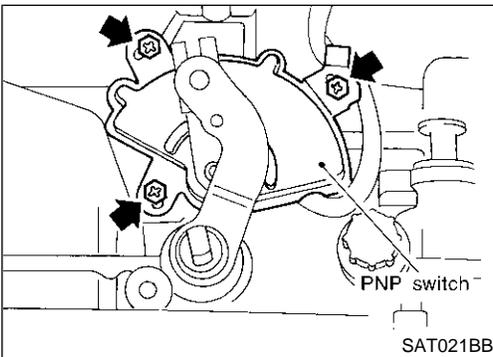
5. Remove PNP switch from transmission case.
