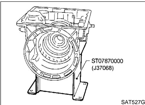
h. Place transmission case into horizontal position.
