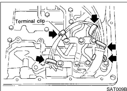
11. Remove control valve assembly.
