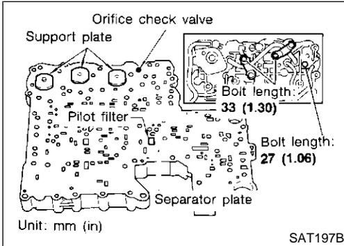
d. Install lower separator plate on lower body.
