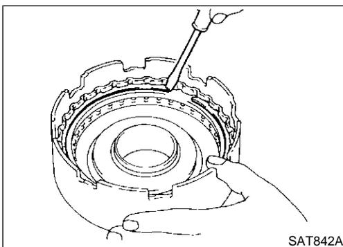
5. Install drive plates, driven plates, retaining plate and dish plate.
