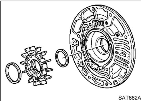
3. Install rotor, vanes and vane rings.
