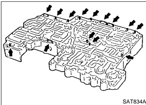
2. Install parallel pins and retainer plates.
