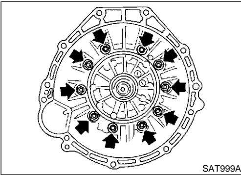
13. Remove converter housing from transmission case.
