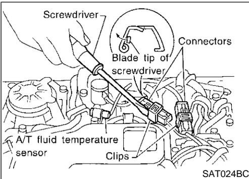
9. Remove torque converter clutch solenoid valve and A/T fluid temperature sensor connectors.
