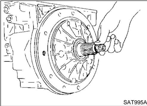
14. Remove O-ring from input shaft.
