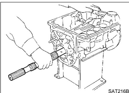
6. Install output shaft and parking gear (4WD model only).
