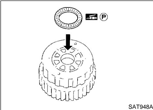
f. Install needle bearing onto rear of overrun clutch hub.
