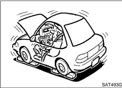
5. Start engine and measure line pressure at idle and stall speed.
