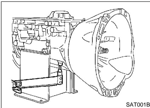
7. Install turbine revolution sensor.
