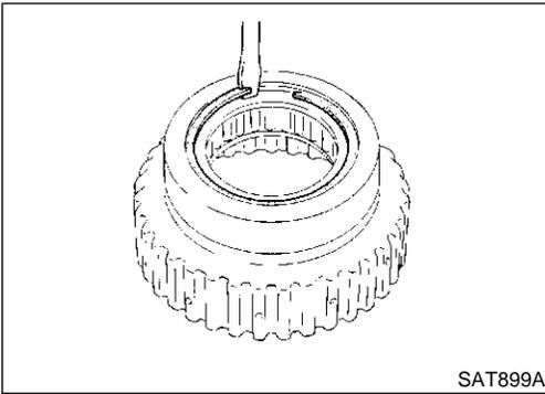
3. Remove snap ring from forward clutch hub.
