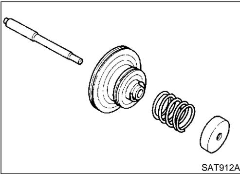
5. Install servo piston spring retainer, return spring C and piston stem onto band servo piston.
