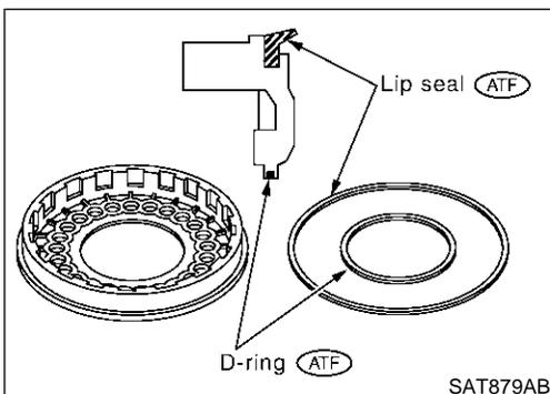
2. Install lip seal and D-ring onto piston.
