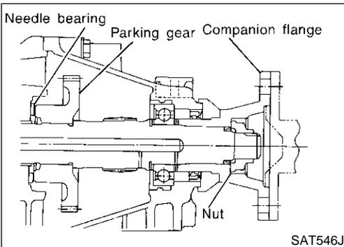
5. Install rear extension assembly on transmission case (2WD model only).
