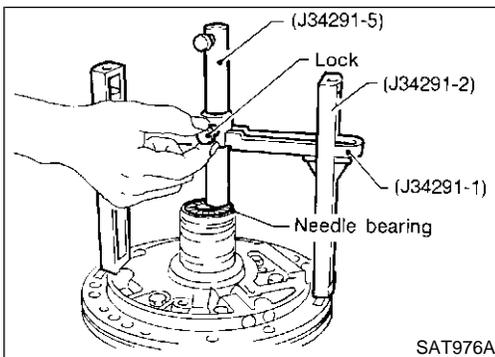
a. With needle bearing installed, place J34291-1 (bridge), J34291-2 (legs) and the J34291-5 (gauging cylinder) onto oil pump. The long ends of legs should be placed firmly on machined surface of oil pump assembly. The gauging cylinder should rest on top of the needle bearing. Lock gauging cylinder in place with set screw.
