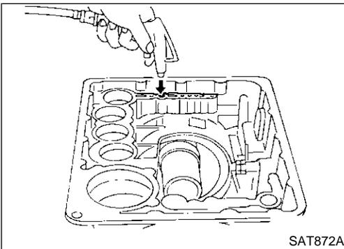
7. Check operation of low and reverse brake clutch piston. Refer to "DISASSEMBLY", AT-322.
