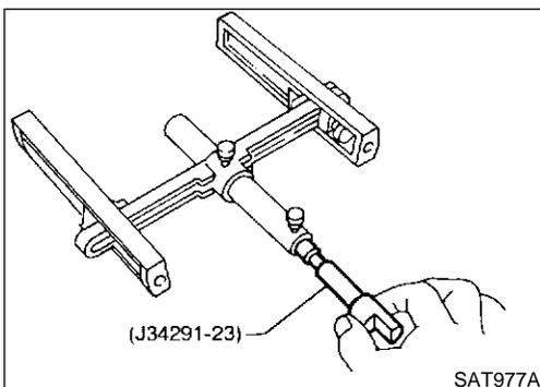
b. Install J34291-23 (gauging plunger) into gauging cylinder.
