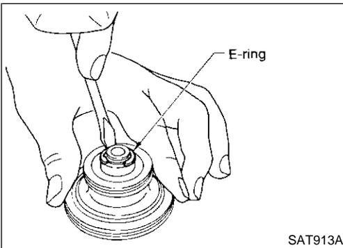
7. Remove E-ring from band servo piston.
