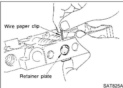
2. Remove valves at retainer plates.
