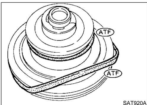
4. Install D-rings onto band servo piston.
