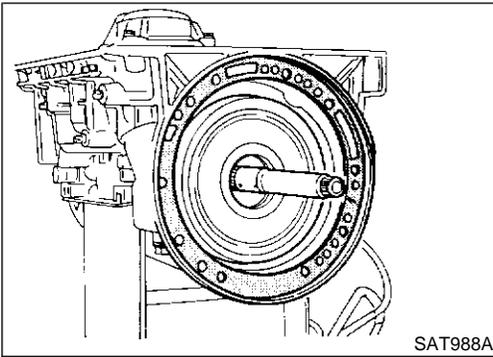
16. Remove input shaft and oil pump gasket.
