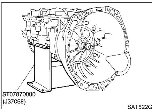
7. Place transmission into Tool with the control valve facing up.
