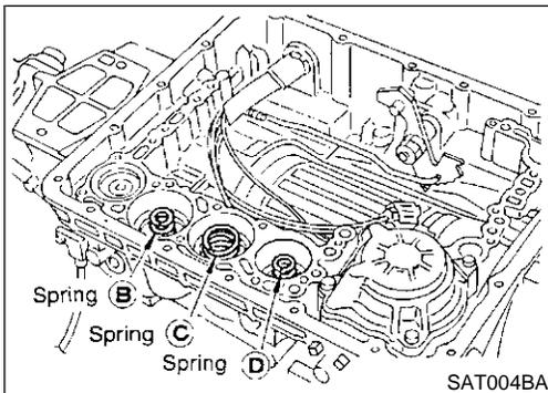
10. Install control valve assembly.
