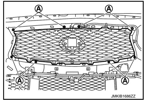
4. Disengage fixing pawls from back side while pulling front grille toward vehicle front, and then remove front grille.
