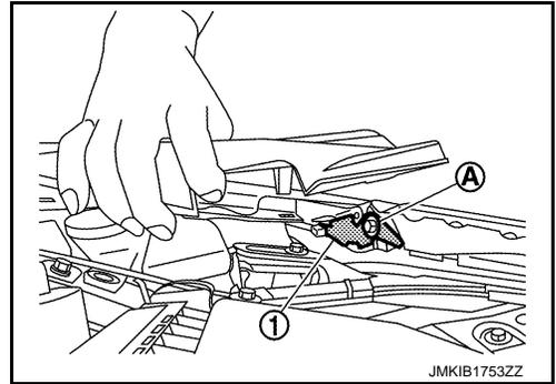
6. Remove front bumper fascia assembly mounting bolts ① of bumper lower side.
