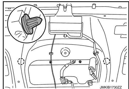
5. Remove the following parts after removing trunk lid finisher.
