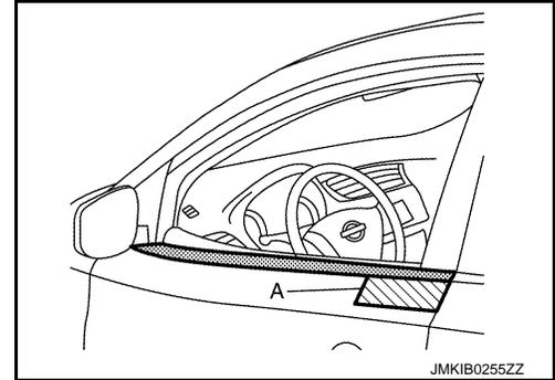
4. Disengage rear end of front door outside molding fixing pawl using remover tool (A) and (B).
