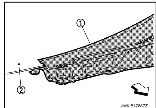
12. Remove the following parts after removing cowl top cover (LH and RH) and hoodledge cover (LH and RH).
