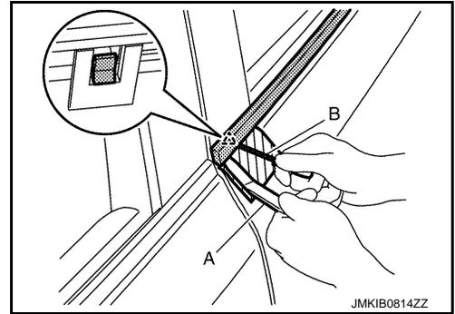
4. Twist rear door outside molding toward the direction of the arrow, and then lift up and remove it.
