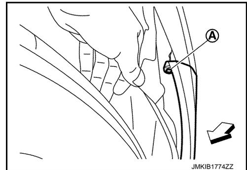
5. Remove rear bumper fascia assembly fixing screws Ⓐ of bumper lower side (LH and RH).
