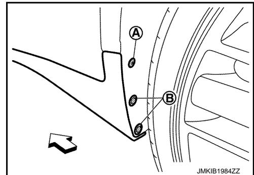
3. Remove sill cover fixing screws of sill cover lower side.
