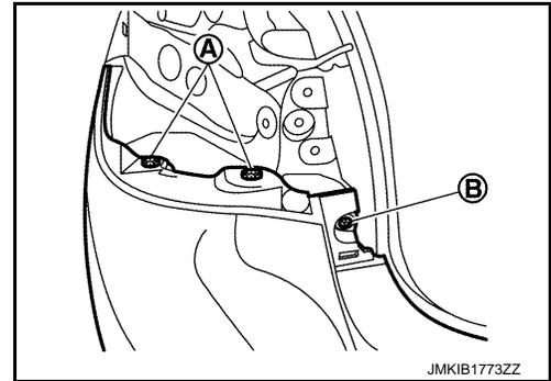
4. Remove rear bumper fascia assembly fixing screws Ⓐ (LH and RH).
