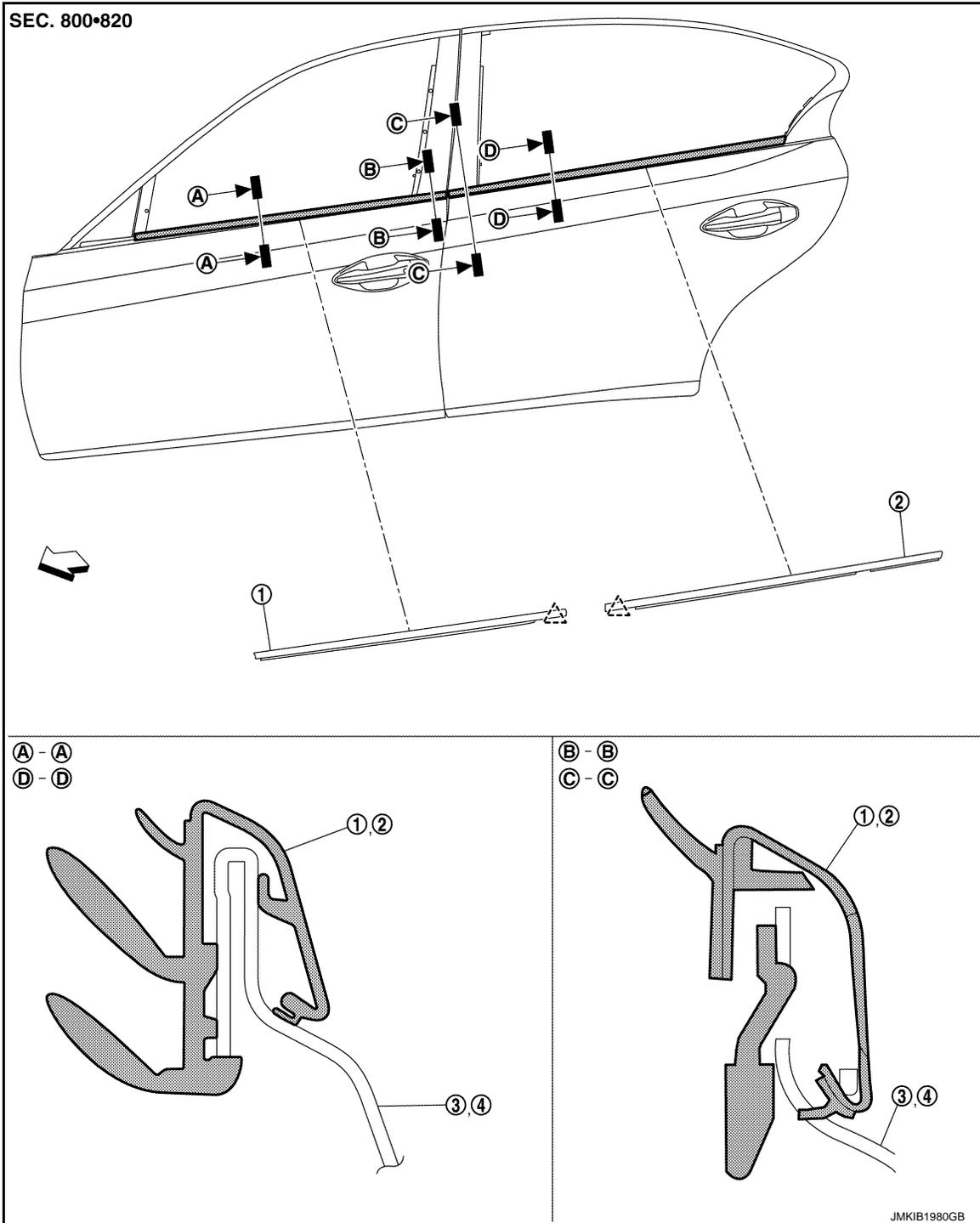
① Front door outside molding      ② Rear door outside molding      ③ Front door panel
