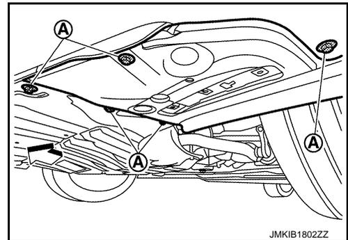
7. Remove fender protector front fixing clips.
