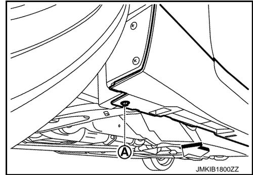
3. Remove front fender protector rear fixing screws (A) from rear side of front fender protector rear.
