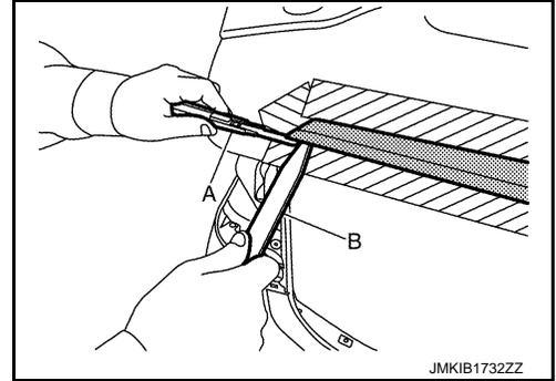
3. Disengage trunk lid molding fixing clips, using a remover tool (A), and then remove trunk lid molding.
