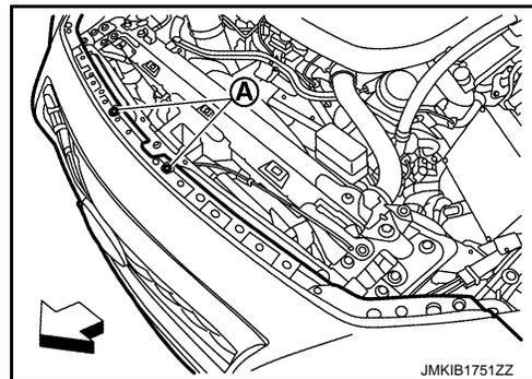
4. Remove fender side seal assembly fixing clip of fender side seal assembly front side (LH and RH).
