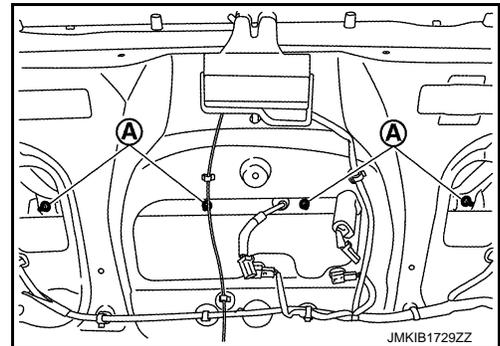
4. Disengage fixing clips of trunk lid finisher from inside of trunk lid, and then remove trunk lid finisher.
