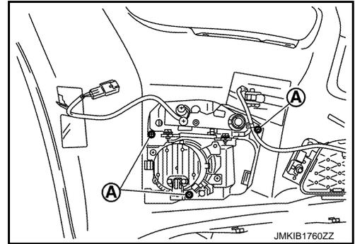
2. Disengage front bumper finisher fixing pawls, and then remove front bumper finisher (LH and RH) as shown by the arrows in the figure.
