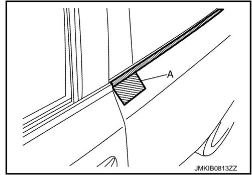
3. Disengage fixing pawl of rear door outside molding front and rear end, using remover tool (A) and (B).
