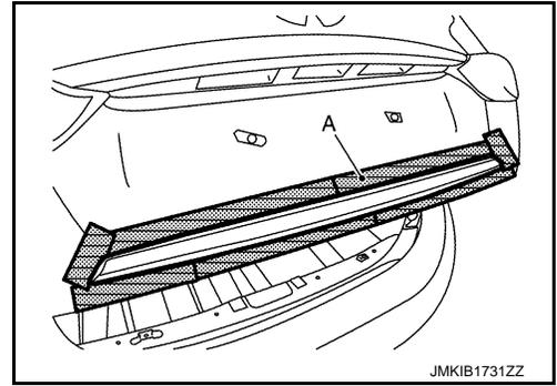
2. Insert a remover tool (A) between trunk lid molding and trunk lid panel, cut double-sided tape using a cutter (B) while lifting trunk lid molding.
