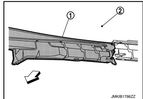
10. Push down pawl (A) as shown by the arrow in the figure to disengage the fitting of cowl top cover LH (1) and windshield glass (2).
