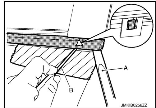
5. Twist front door outside molding toward the direction of the arrow, and then lift up and remove it.
