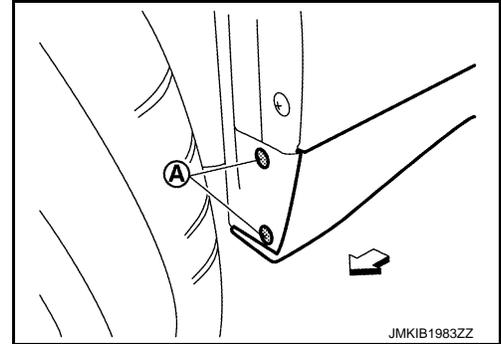
2. Remove sill cover fixing screw (A) and clips (B) of sill cover rear end.
