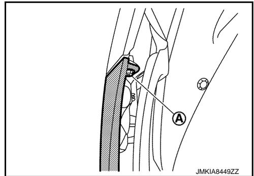
9. Apply protective tape (A) on the part to protect it from damage.
