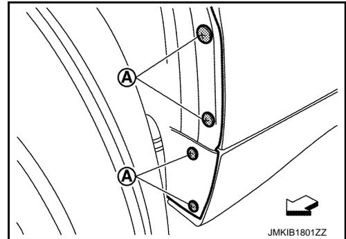
4. Remove front fender protector rear fixing clips.
