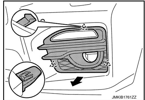
19. Remove front bumper fascia bracket fixing screws, and then remove front bumper fascia bracket (LH and RH).
