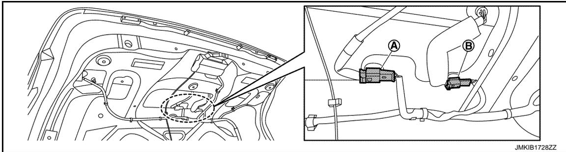
3. Remove trunk lid finisher mounting nuts (A).
