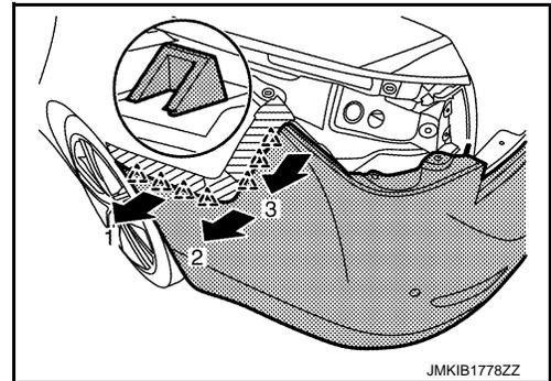
9. Disengage rear bumper fascia assembly fixing clips as shown by the arrow in the figure
