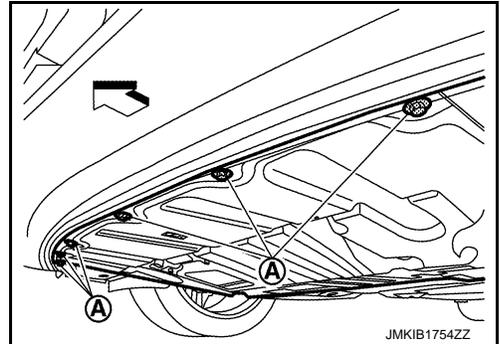
7. Remove fender protector mounting bolts ① from front side of front fender protector front (LH and RH).
