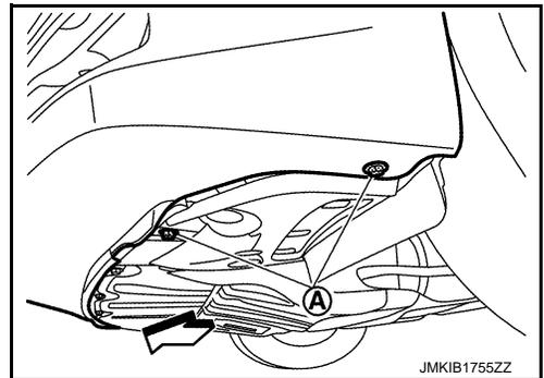
8. Remove front bumper fascia assembly fixing screws ① (LH and RH).
