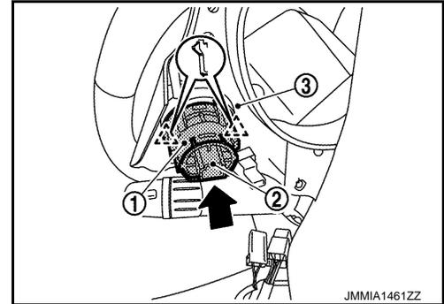
4. Disengage NATS antenna amp. fixing pawl and then remove NATS antenna amp. ② from push-button ignition switch ①.
