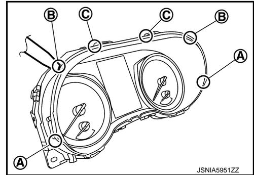
4. Pull the front cover straight to remove it from the unified meter control unit.
