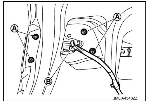
5. Pull rear combination lamp (trunk lid side) out off trunk lid panel and remove it.
