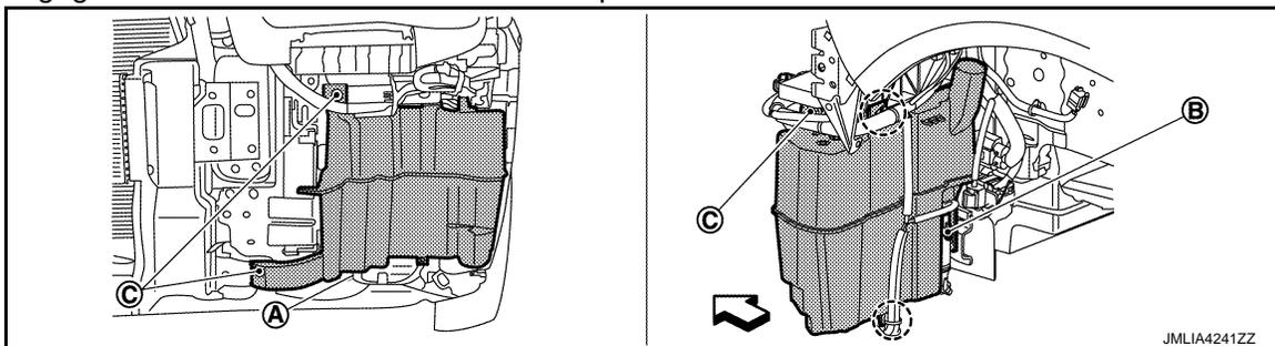
Ⓐ Washer level switch harness connector    Ⓑ Washer pump harness connector    Ⓒ Washer tank fixing bolt
