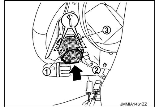
4. Disengage push-button ignition switch fixing pawl and then remove push-button ignition switch ① from NATS antenna amp. ②.
