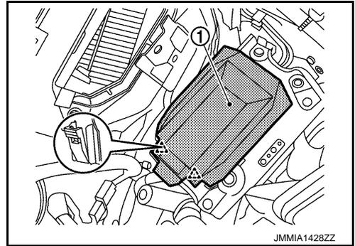
5. Disconnect harness connector and then remove IPDM E/R ① from IPDM E/R cover B ②.
