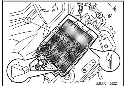
6. Remove the mounting bolts (A) and remove the bracket ①.
