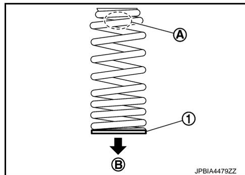
11. Install valve spring retainer.
