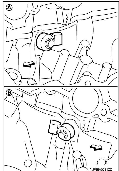
17. Install new rear oil seal. Refer to [EM-76](#), "REAR OIL SEAL : Removal and Installation".
