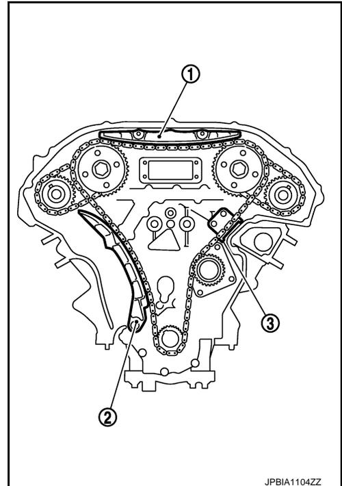
35. Remove timing chain (primary) and crankshaft sprocket.
