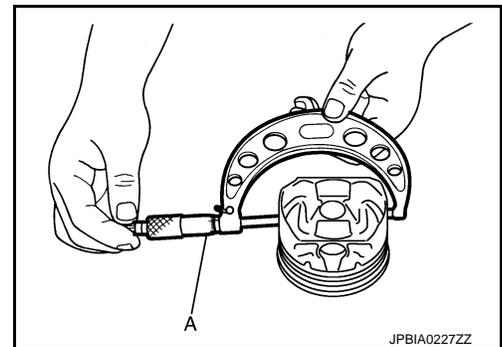
Piston-to-Cylinder Bore Clearance
