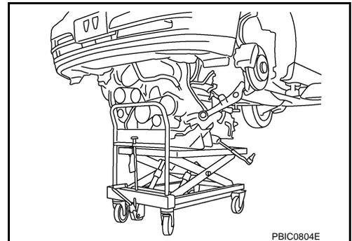
2. Remove rear engine mounting member bolts.
