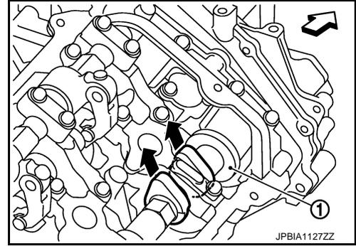
27. Remove crankshaft pulley as follows:
