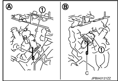
2. Install oil filter ①, if removed.
