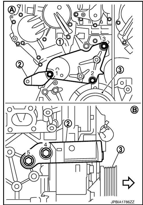
16. Install idler pulley brackets as follows (With DIRECT ADAPTIVE STEERING):
