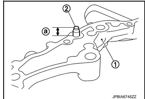
9. Install new front oil seal on front timing chain case.
