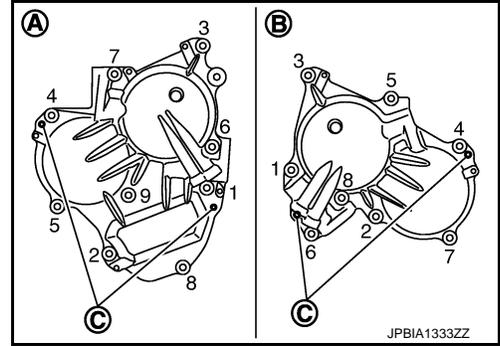
12. Install oil pan (lower). Refer to [EM-49, "Removal and Installation"](#).
