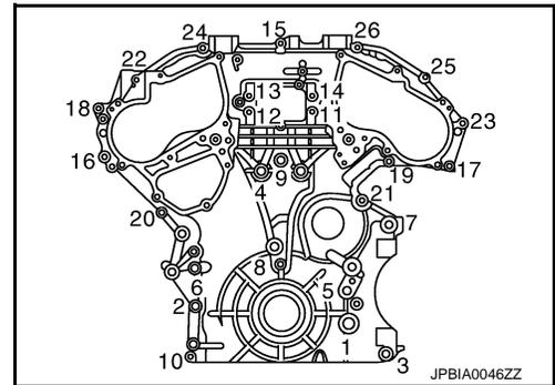
f. After all bolts are tightened, retighten them to the specified torque in numerical order shown in the figure.
