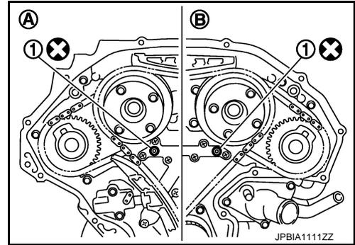
33. Remove timing chain tensioner (primary) ① as follows:
