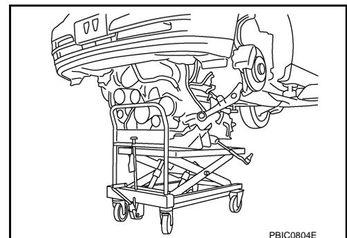
2. Remove rear engine mounting member bolts.
