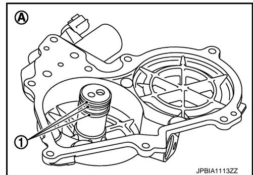
b. Install intake valve timing control cover with new gasket to front timing chain case.
