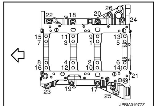
9. Remove lower cylinder block as follows:
