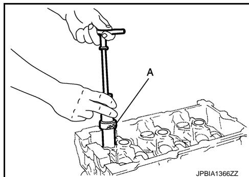
10. Remove valve seat (EXH), if valve seat (EXH) must be replaced.
