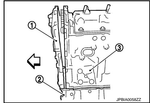
d. Install front timing chain case fitting its dowel pin hole together with dowel pin on rear timing chain case.
