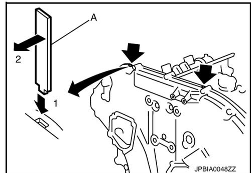
31. Remove front oil seal from front timing chain case using a suitable tool.
