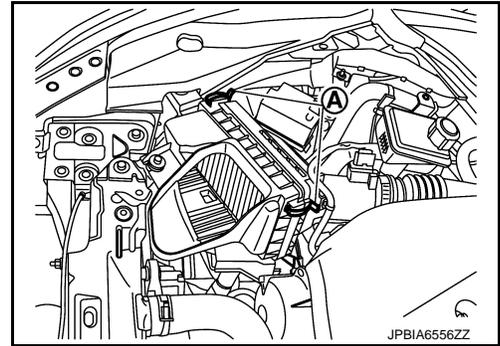
3. Lift up air cleaner cover (1), and remove air cleaner filter (2).
