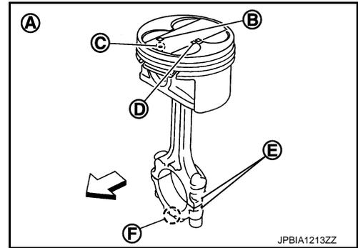
c. Install new snap ring to the groove of the piston front side.
