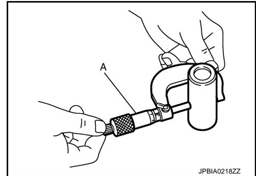
Connecting Rod Bushing Oil Clearance
