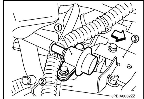
7. When separating fuel feed hose (with damper) and centralized under-floor piping connection, disconnect quick connector as follows:
