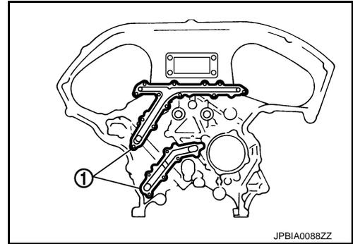
5. Remove O-rings ① from cylinder block.
