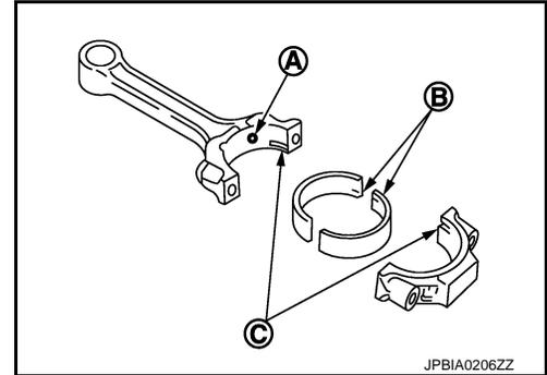
12. Install piston and connecting rod assembly to crankshaft.
