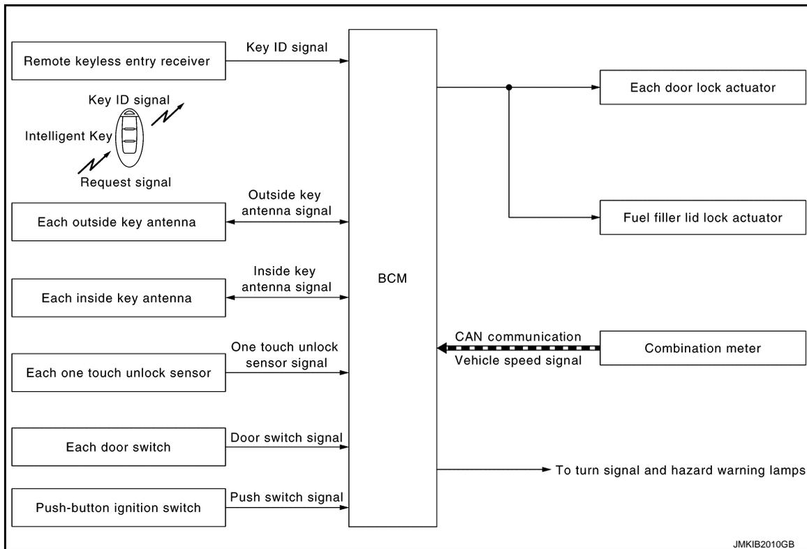
One touch unlock function controls operation function of the following items.
