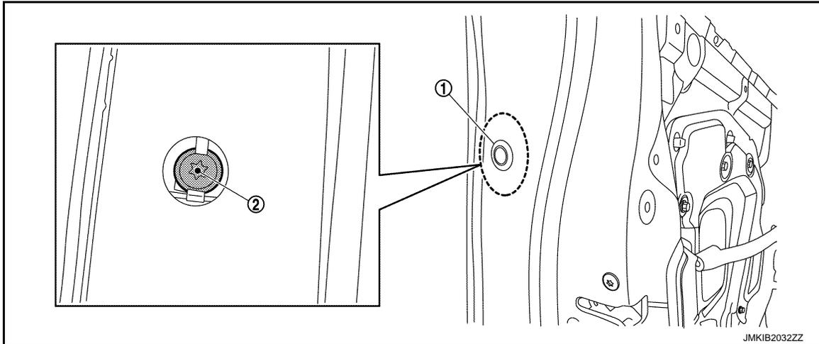
8. In the order of 1 → 2 as shown in the figure, while pulling outside handle grip ①, remove outside handle escutcheon ②.
