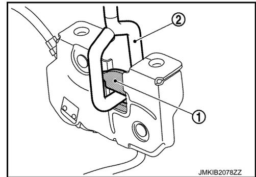
3. While operating the hood opener carefully, check that the front end of the hood is lifted by approximately 20 mm (0.787 in) (A). Also, check that the hood opener returns to the original position.
