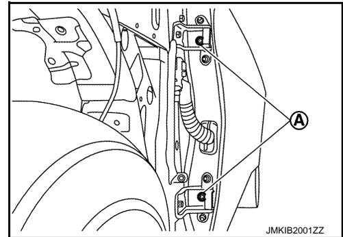
6. Temporarily tighten door hinge mounting nuts on door side.
