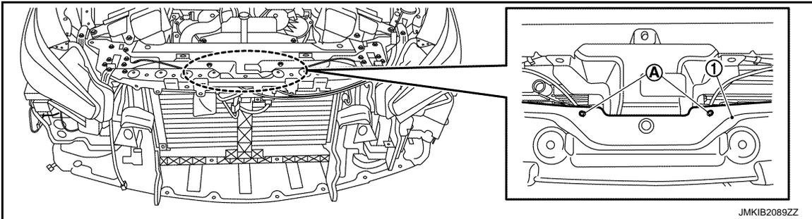
4. Remove hood lock control cable (front) from tube clip of front bumper upper retainer.
