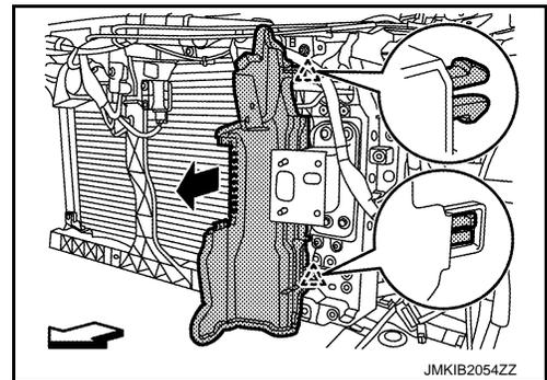
14. Disconnect hood lock control cable (rear) from hood lock control cable (front). Refer to [DLK-219, "HOOD LOCK CONTROL CABLE : Removal and Installation"](#).
