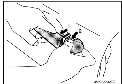
7. In the order of 1 → 2 as shown in the figure, while pulling outside handle grip ①, slide toward rear of vehicle to remove outside handle grip.
