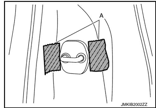
2. Disengage fixing pawls of door striker cover using a remover tool (A), and then remove door striker cover.
