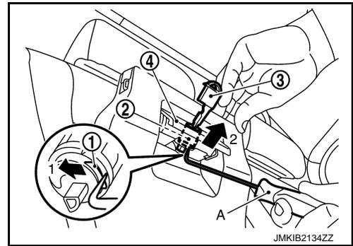
5. Remove sleeve ③ from seatback lid knob, and then install sleeve to seatback lid lock cylinder ②.
