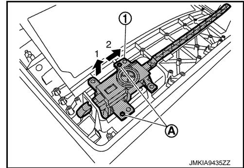
6. In the order of 1 → 2 as shown in the figure, disconnect rod ② from rod slide hole portion ① while pulling handle ① of glove box lock assembly.
