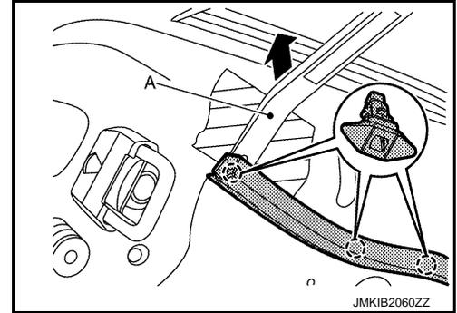
3. Remove radiator core seal.
