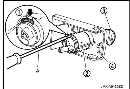
11. Remove sleeve ③ from handle, and then install sleeve to glove box lid lock cylinder ②.
