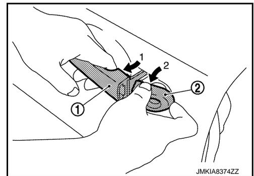
9. In the order of 1 → 2 as shown in the figure, while pulling outside handle grip ①, slide toward rear of vehicle to remove outside handle grip.
