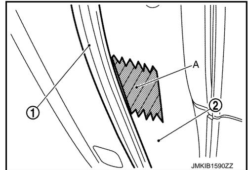
2. Disengage fixing clips on the reverse side of rear door weather-strip using a remover tool (A).
