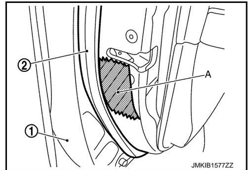
2. Disengage fixing clips on the reverse side of front door weather-strip using a remover tool (A).
