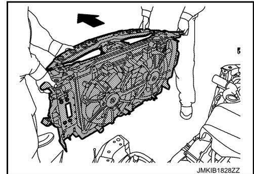
19. Remove the following parts after removing radiator core support.
