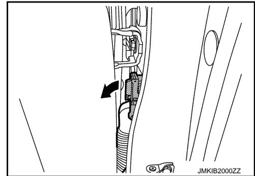
2. Remove door check link mounting bolt on vehicle body side.
