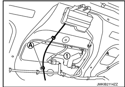
5. Disengage pawls of trunk lid lock cover ①. Open trunk lid lock cover in direction indicated by the arrow as shown in the figure.
