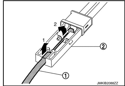
3. Disengage hood lock control cable (rear) ① fixing pawls, and then remove hood lock control cable (rear) from instrument lower panel ② according to the numerical order 1 → 2 indicated by arrows as shown in the figure.
