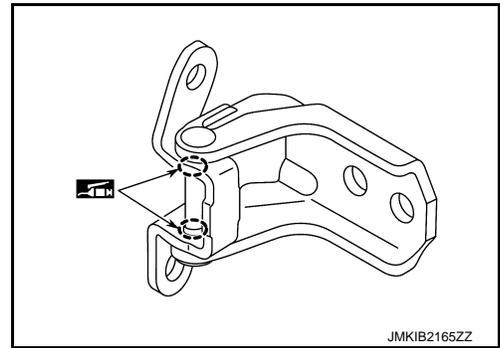
3. Check door check link rotating part for poor lubrication. If necessary, apply body grease.
