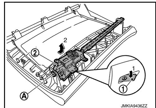
7. Remove glove box lock assembly.
