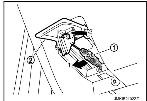
5. Remove dash side finisher (driver side). Refer to [INT-28. "DASH SIDE FINISHER : Removal and Installation"](#).
