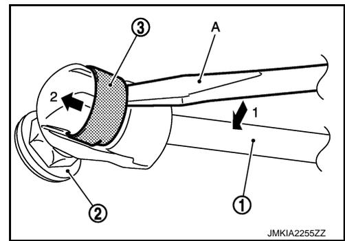
4. Disengage the stud ball from the hood stay (hood side).
