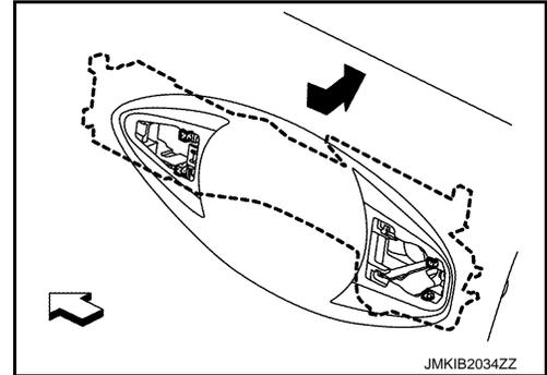
10. Disconnect outside handle cable ① according to the numerical order 1 → 2 indicated by arrows as shown in the figure from outside handle bracket ②.
