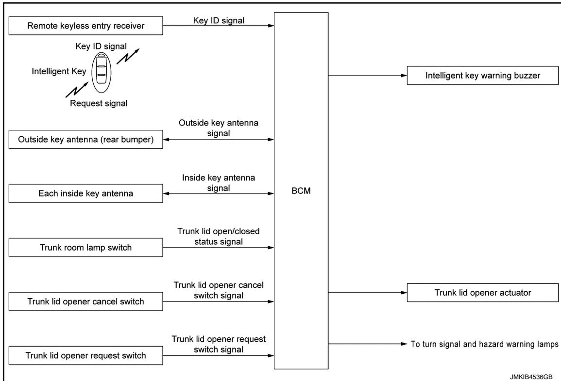
Trunk open function controls operation function of the following items.
