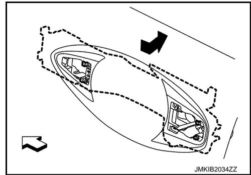
12. Disconnect outside handle cable ① according to the numerical order 1 → 2 indicated by arrows as shown in the figure from outside handle bracket ②.
