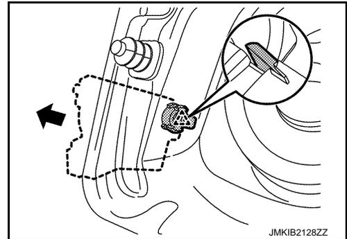
5. Disconnect fuel lid lock actuator harness connector, and then remove fuel lid lock actuator.
