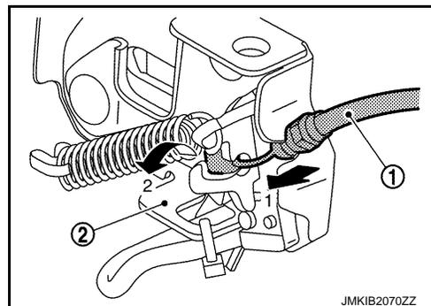
6. Remove hood lock mounting bolts, and then remove hood lock.
