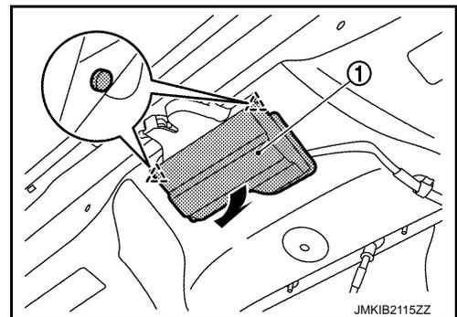
6. Disconnect harness connector from trunk lid lock assembly.
