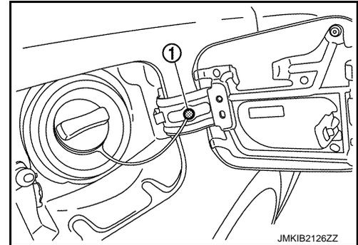
4. Remove fixing screws, and then remove fuel filler lid assembly.
