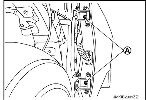
4. Adjust the surface height of front door according to the fitting standard dimension.
