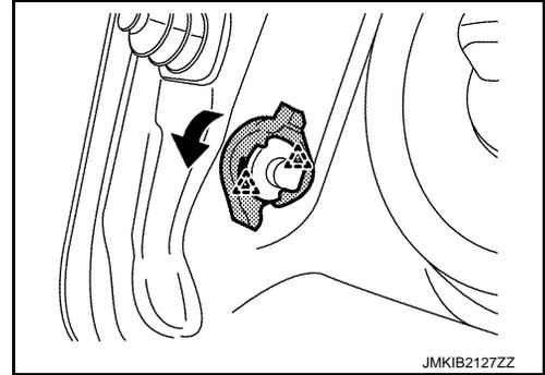
4. Push fuel lid lock actuator behind the vehicle, while pushing the pawl.
