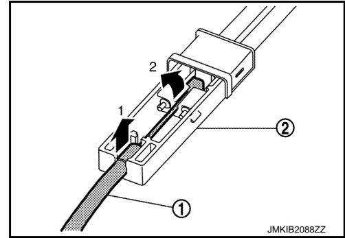
3. Remove hood lock control cable (front) fixing clips ① from front bumper upper retainer ①.
