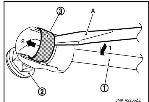
5. Disengage trunk lid stay from stud ball (trunk lid assembly side of trunk lid hinge).
