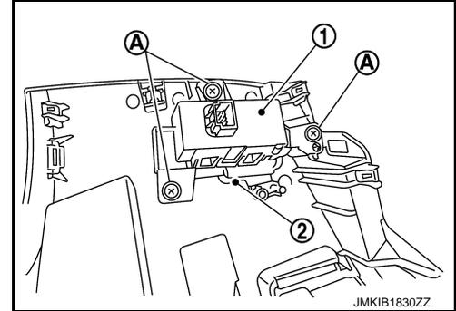
3. Remove trunk lid opener switch (1) from triple switch bracket (2).
