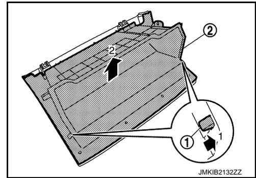
4. Remove glove box lock assembly fixing screws.
