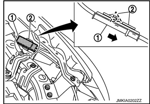
9. Remove the hood lock control cable cover from hood lock control cable protector.
