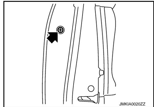
5. Disconnect door antenna and door request switch connector and remove harness clamp.
