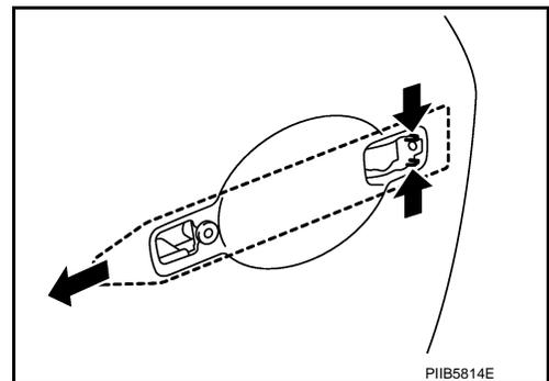
11. Disconnect the door lock actuator connector and remove the door lock assembly.
