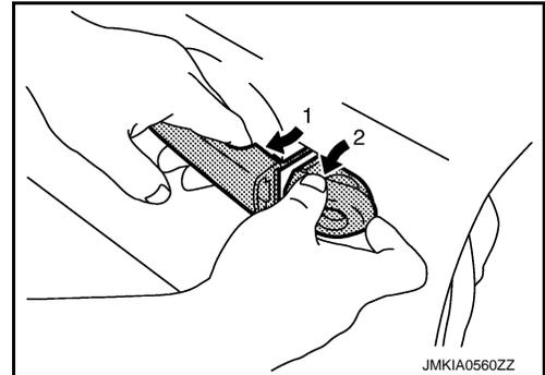
6. Slide outside handle (1) toward rear of vehicle and pull to remove outside handle.
