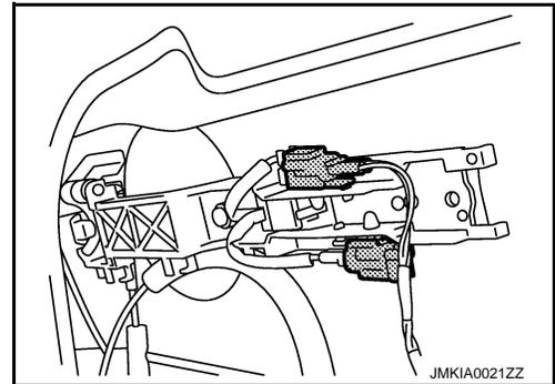
6. Reach in to separate the key rod connection (on the handle).
