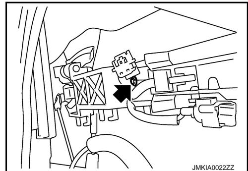
12. While pulling outside handle bracket, slide toward rear of vehicle to remove outside handle bracket.
