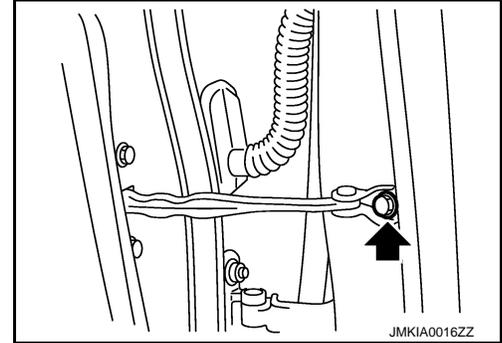
2. Pull out grommet and disconnect rear door harness connector.
