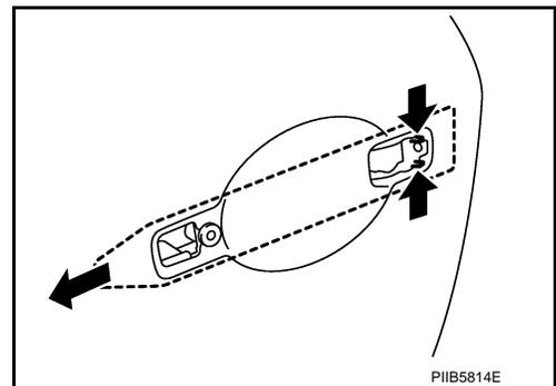
13. Disconnect the door lock actuator connector and remove the door lock assembly.
