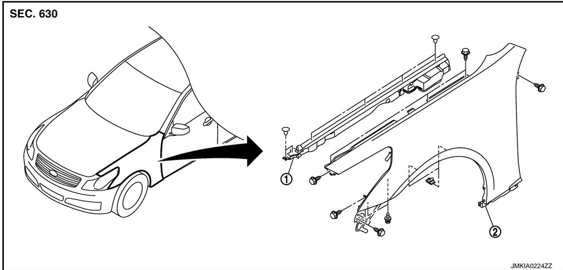
1. Hood seal assembly (side)      2. Front fender
